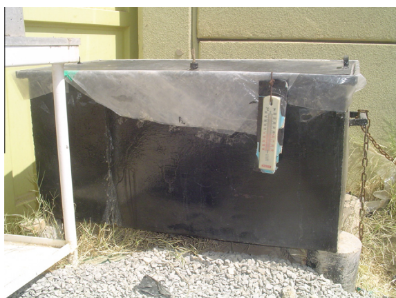
Fig. 2. Steam curing chamber exposed to solar radiation.
