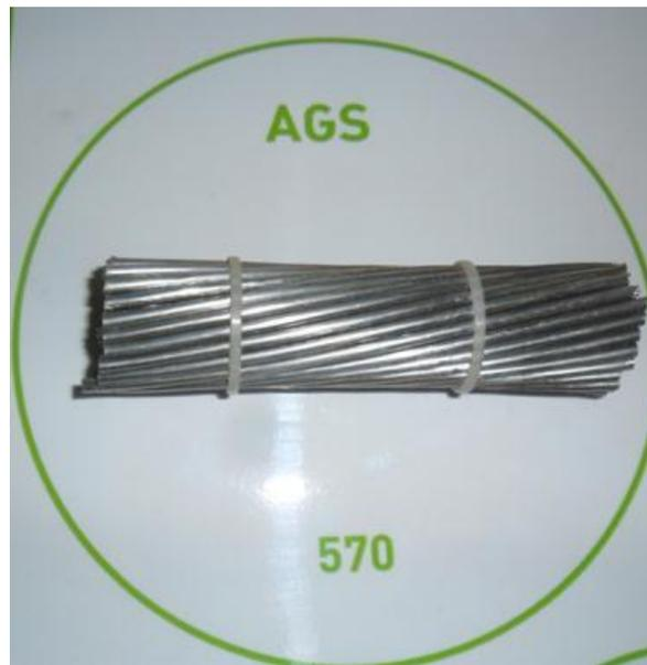
**Figure III.1** : Fil machine d'AGS
