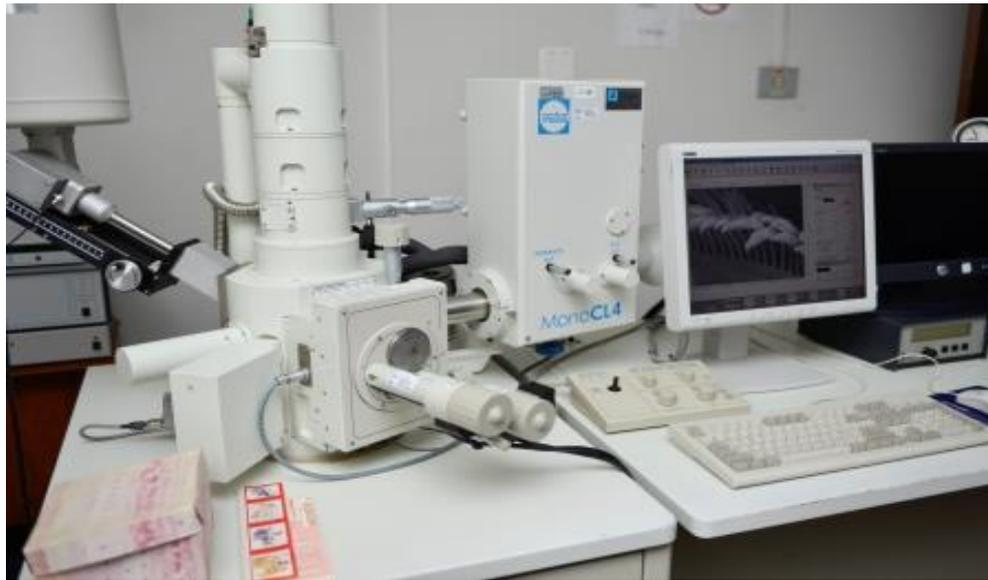
**Fig.II.15:** MEB type JEOL, JSM 6360 LV
