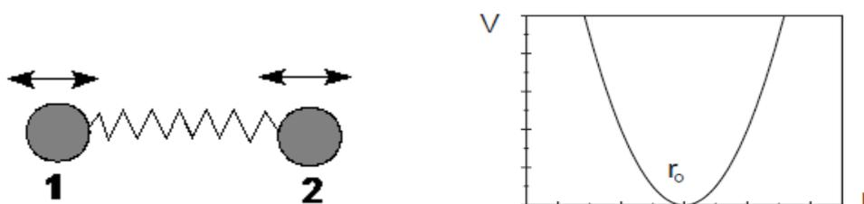
**Figure II.2** : Bond stretching between two bonded atoms.
