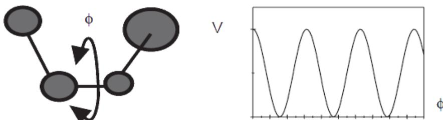
**Figure II.4:** Torsion between four bonded atoms.
