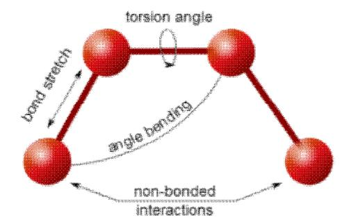
**Figure II.1 :** Intramolecular interactions between bonded and non-bonded atoms
