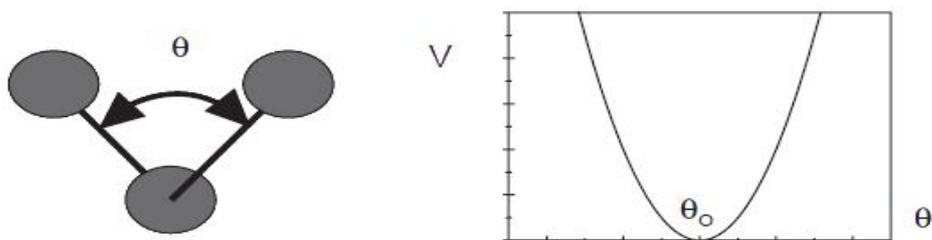
**Figure II.3:** Angle bending between three dependent atoms .
