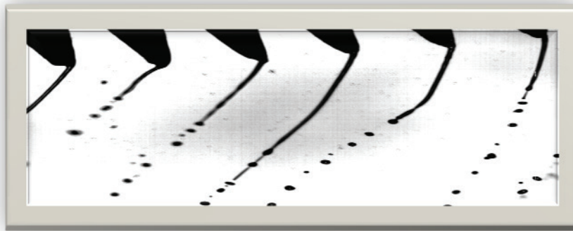
Fig. 2. Drop formation for Micromax 120.
