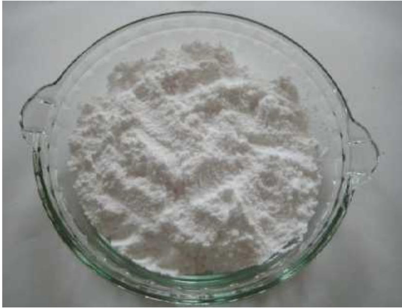
Figure. II.3: InCl<sub>3</sub> powder
