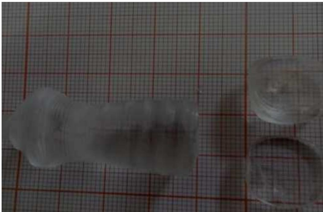
Fig.II.2: Photograph of a KCl single crystal substrate.
