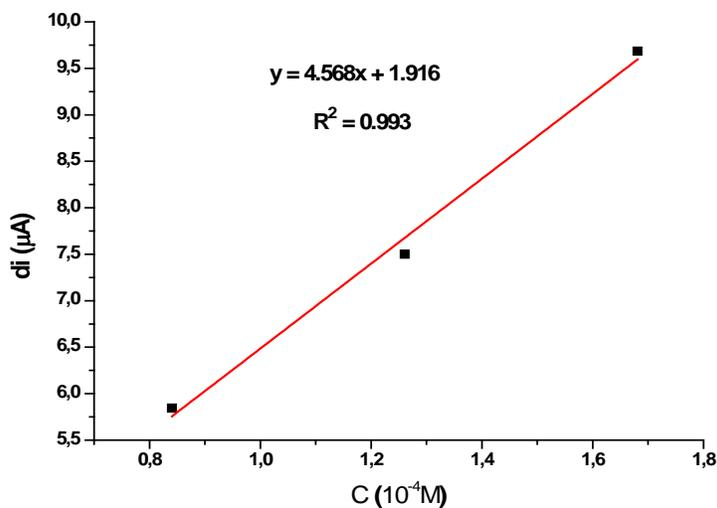
**Figure III-4-24:** Calibration curve obtained from SWV for different *N'*-Ferrocenylmethyl-*N'*-phenylbenzohydrazide concentrations in octanol.
