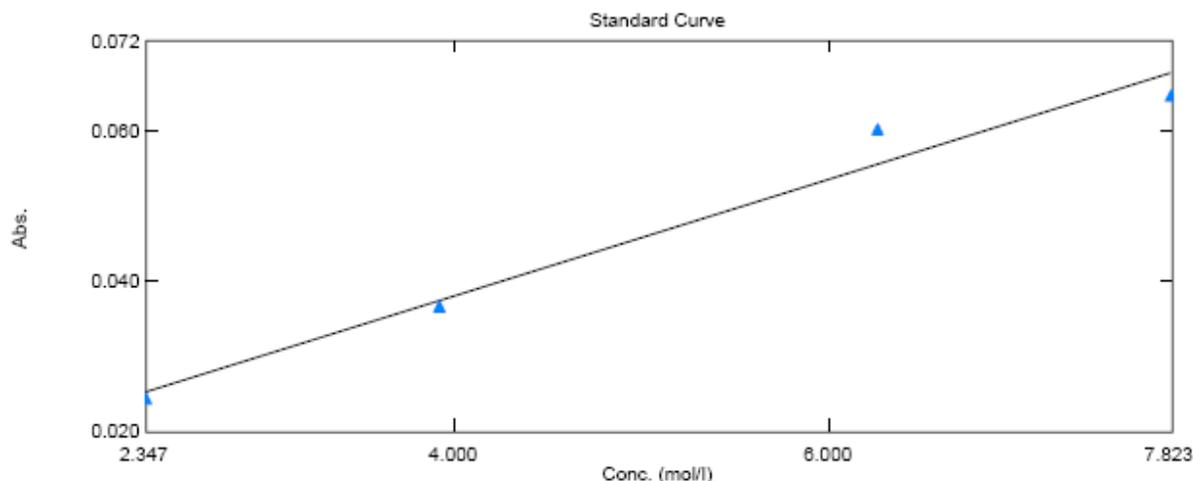
**Figure III-4-33:** Calibration curve obtained from UV-visible 1800 for different 1-ferrocenylethanol concentrations in aqueous at  $\lambda_{246nm}$  wavelength.
