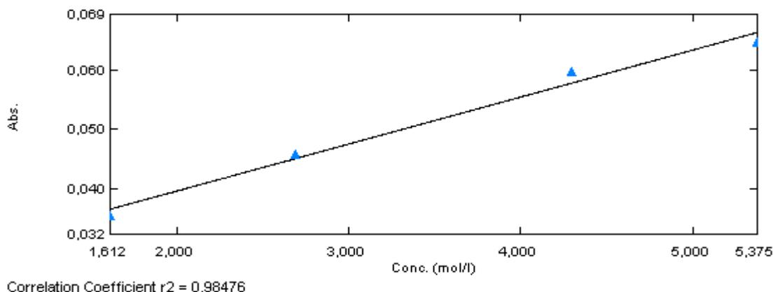
**Figure III-4-32:** Calibration curve obtained from UV-visible1800 for different ferrocene concentrations in aqueous at  $\lambda_{248nm}$  wavelength.
