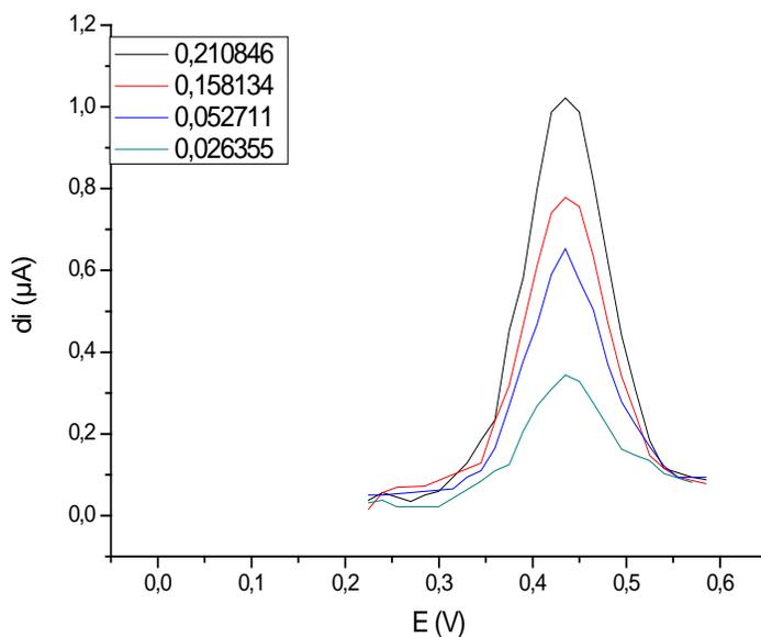
**Figure III-4-26:** Square wave voltammograms referring to different 2-(ferrocenyl methylamino)benzonitrile concentrations in octanol.
