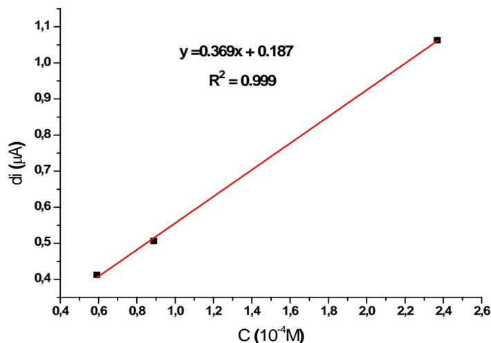
**Figure III-4-21:** Calibration curve obtained from SWV for different *N*-ferrocenylmethylaniline concentrations in octanol.
