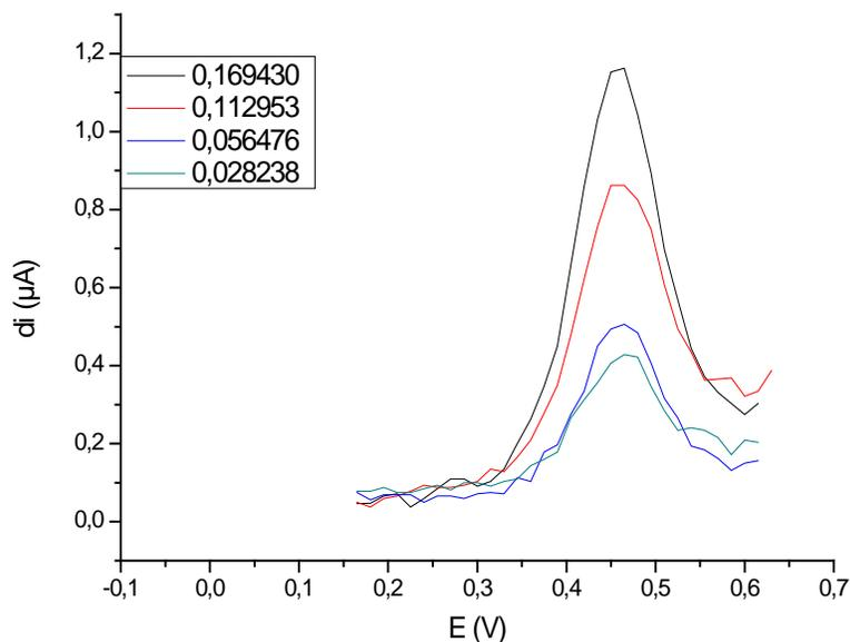
**Figure III-4-29:** Square wave voltammograms referring to different 4- (ferrocenyl methylamino)benzonitrile concentrations in octanol.
