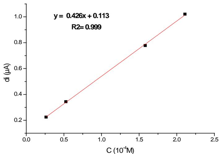
**Figure III-4-27:** Calibration curve obtained from SWV for different 2-(ferrocenyl methylamino)benzonitrile concentrations in octanol.
