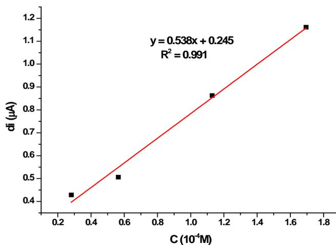
**Figure III-4-30:** Calibration curve obtained from SWV for different 4-(ferrocenyl methylamino)benzonitrile concentrations in octanol.
