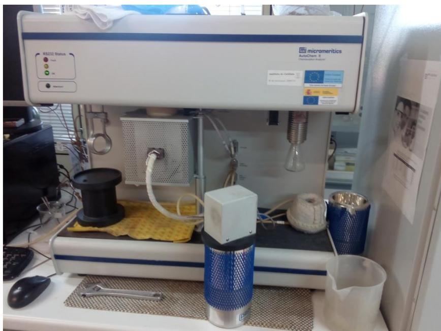
*Figure II.14 Micrometrics apparatus model ASAP-2000.*
