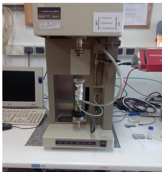
*Figure II.13 Perkin-Elmer TGA7 and a Perkin-Elmer DTA7 devices.*
