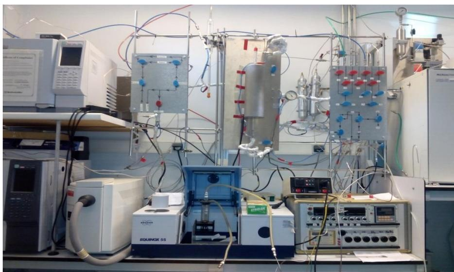
*Figure II.21* different parts used in tests of catalytic activity for CO oxidation.
