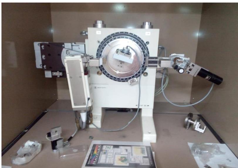
Figure II.6 Bruker D8 Advance diffractometer.
