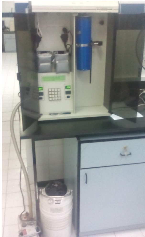
Figure II.7: Appareil d'analyse BET Quantachrome
