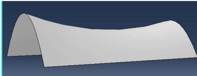
Fig.4.24 Optimal vault shape in case of  $S2$  and  $S3$  variables
