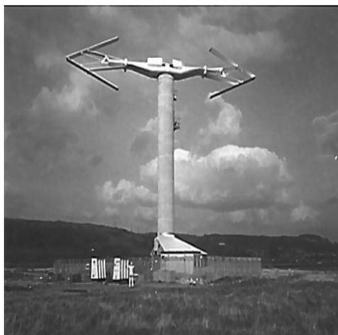
**Fig.I.9.** Darrieus–Masgrowe (two-tier) rotor [13]
