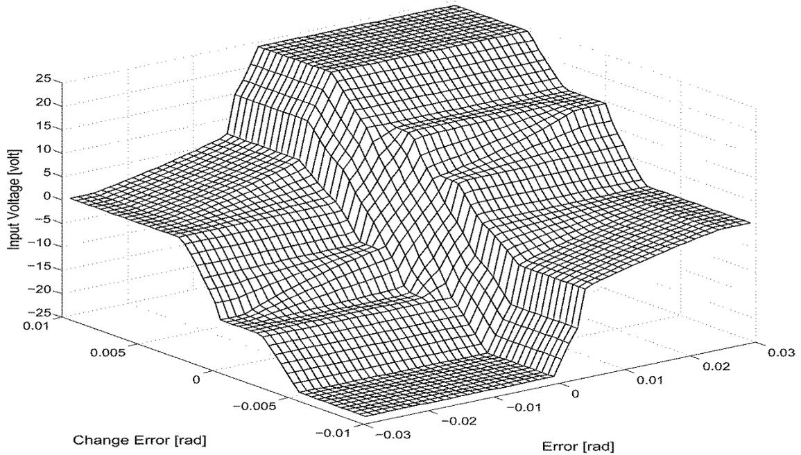
**Fig. IV.15. Control surface of the SFC evolved by the EA.**
