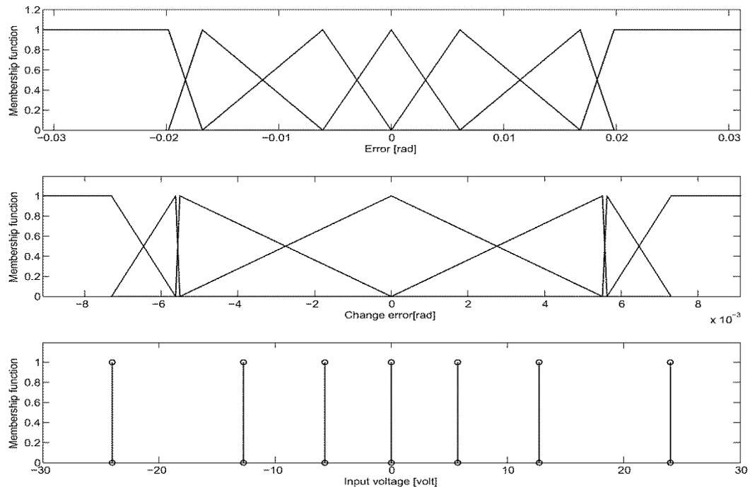
**Fig. IV.14. Best fuzzy partitions for the input/output variables of the SFC evolved by the proposed EA.**
