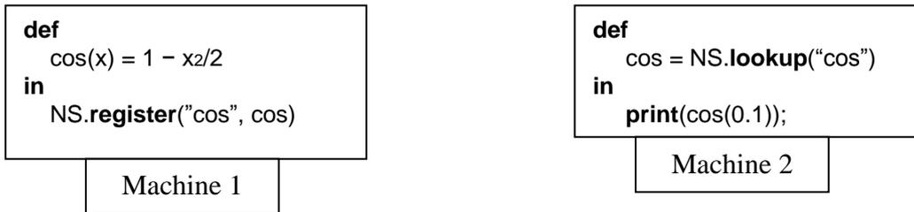
In this first example, on the machine 1, a process defines a local name **cos** and registers it to the name server NS. On the machine 2, a second process obtains the name **cos** and does a remote call.
