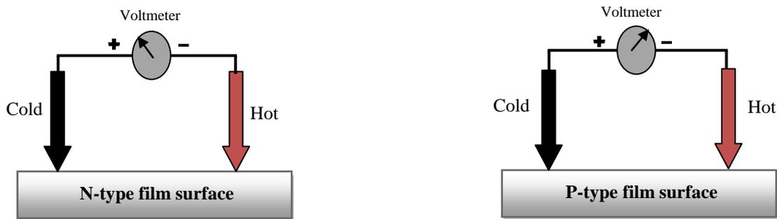
**Figure II.22.** Hot probe technique for measuring Conduction nature of thin Film
