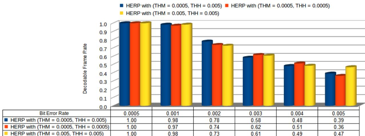
Figure 5.8: Variation of Decodable Frame Rate with BER between HERP with ( $THM = 0.0005$ ,  $THH = 0.005$ ), HERP with ( $THM = 0.0005$ ,  $THH = 0.0005$ ) and HERP with ( $THM = 0.005$ ,  $THH = 0.005$ )
