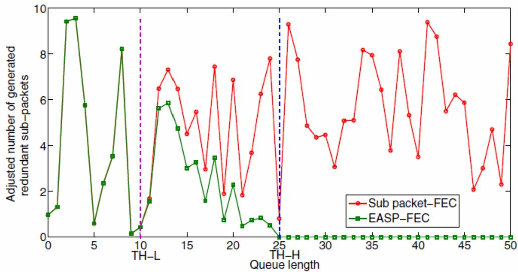
Figure 4.9: Variation of adjusted number of redundant sub-packets with Queue Length
