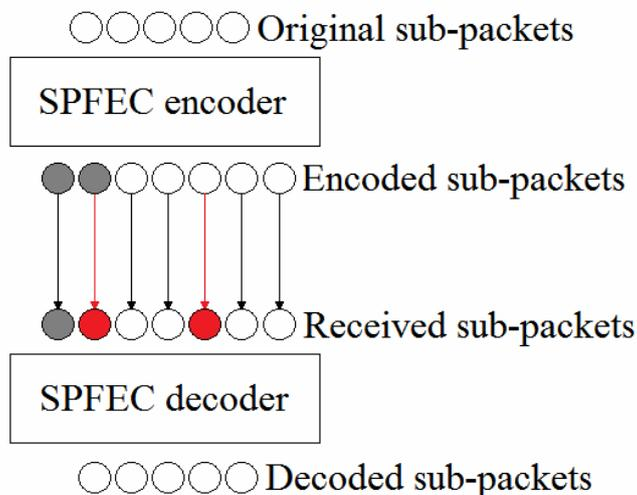
Figure 4.1: Sub-Packet Forward Error Correction mechanism
