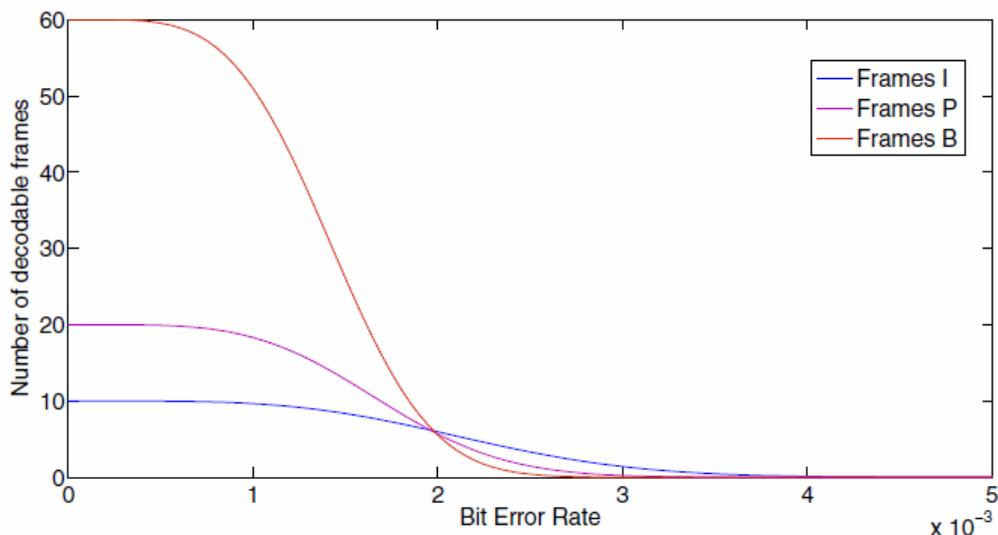
Figure 4.10: Variation of Number of decodable frames with Bit Error Rate
