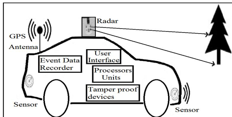
Figure 2.2: Vehicle On-Board Unit
