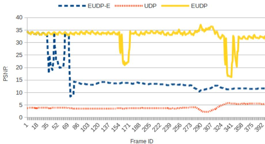
Figure 4.18: PSNR of video frames in the case of BER = 0.002
