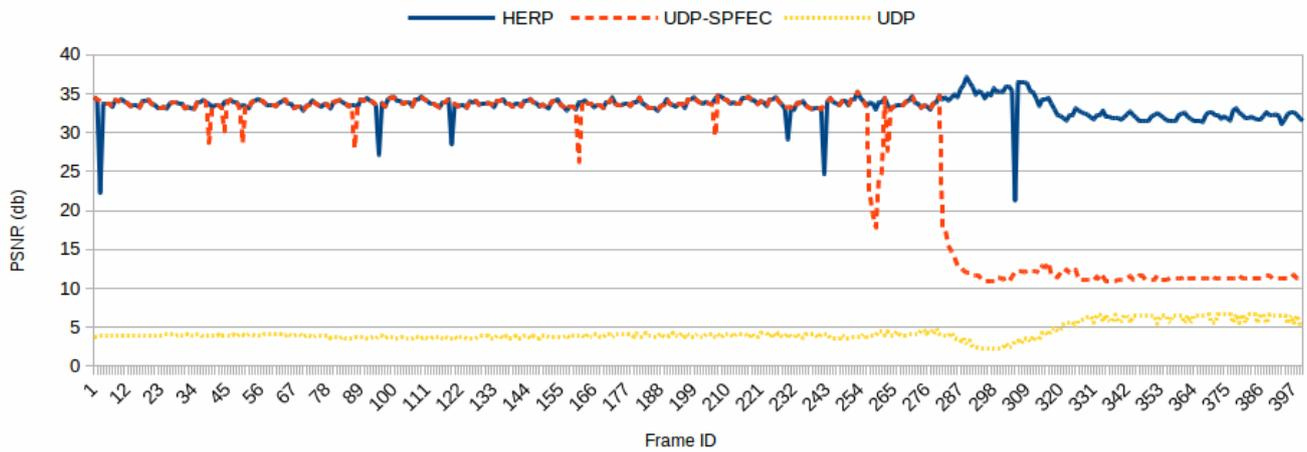
Figure 5.11: PSNR of video frames in the case of BER = 0.001
