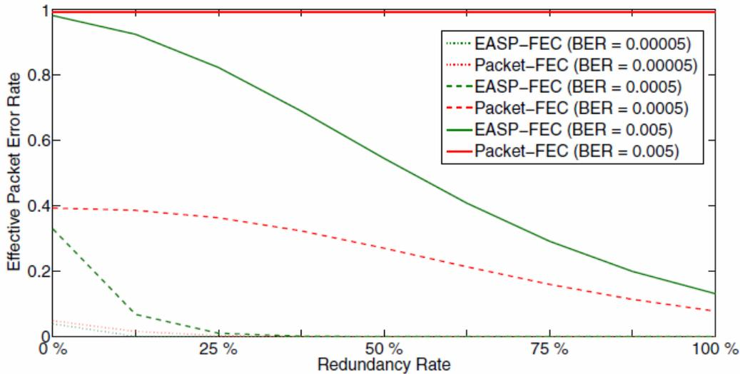
Figure 4.7: Variation of Effective Packet Error Rate with Redundancy Rate
