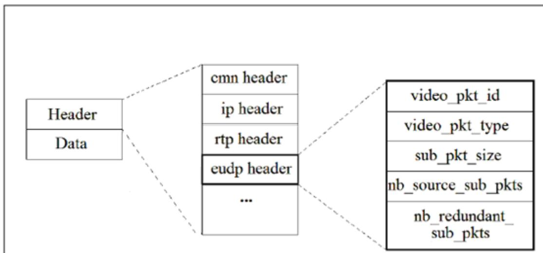
Figure 4.12: Video packet format in EUDP protocol
