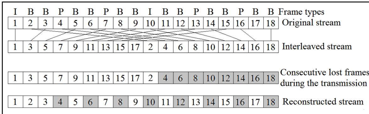
Figure 2.10: An example of interleaving technique with a distance of 2
