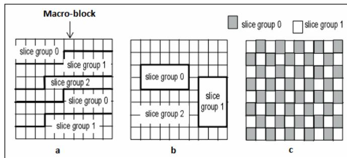
Figure 2.8: Three types of FMO coding of H.264/AVC standard
