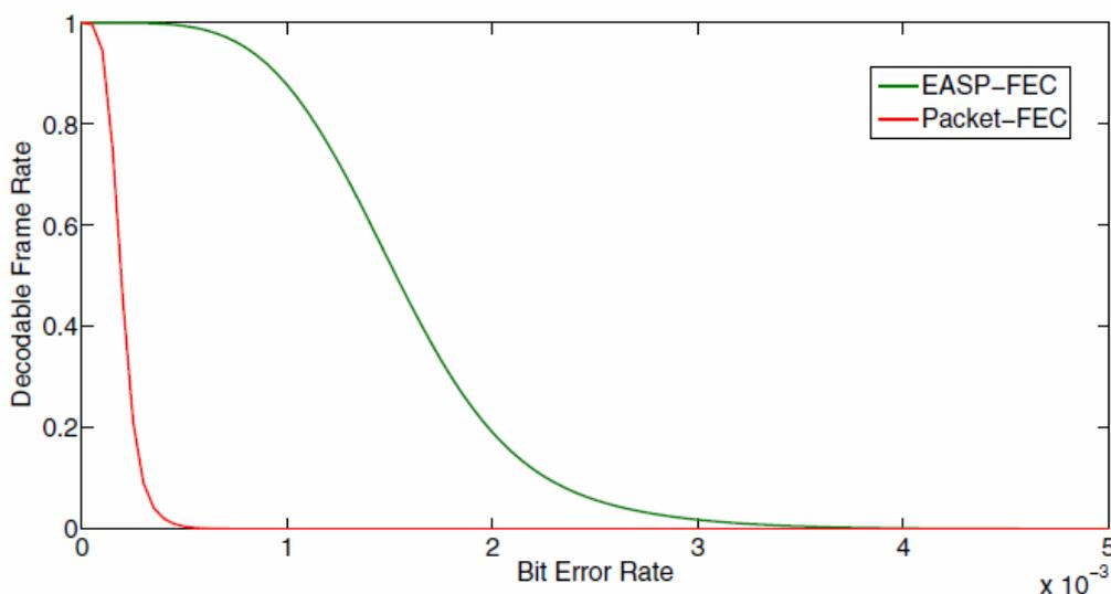
Figure 4.6: Variation of Decodable Frame Rate with Bit Error Rate
