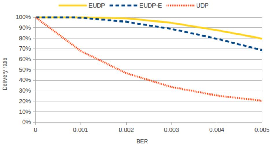
Figure 4.17: Variation of delivery ratio of video packets with BER
