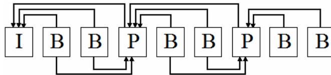
Figure 2.7: GoP structure of MPEG standard
