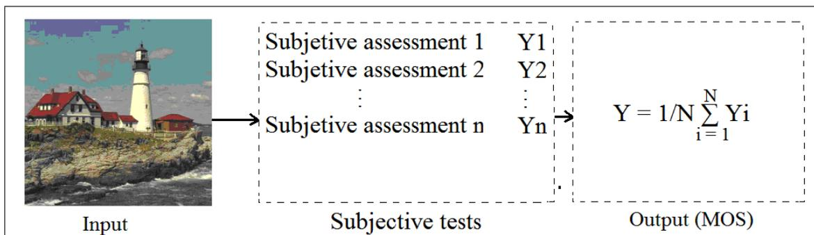
Figure 2.6: The process of obtaining MOS
