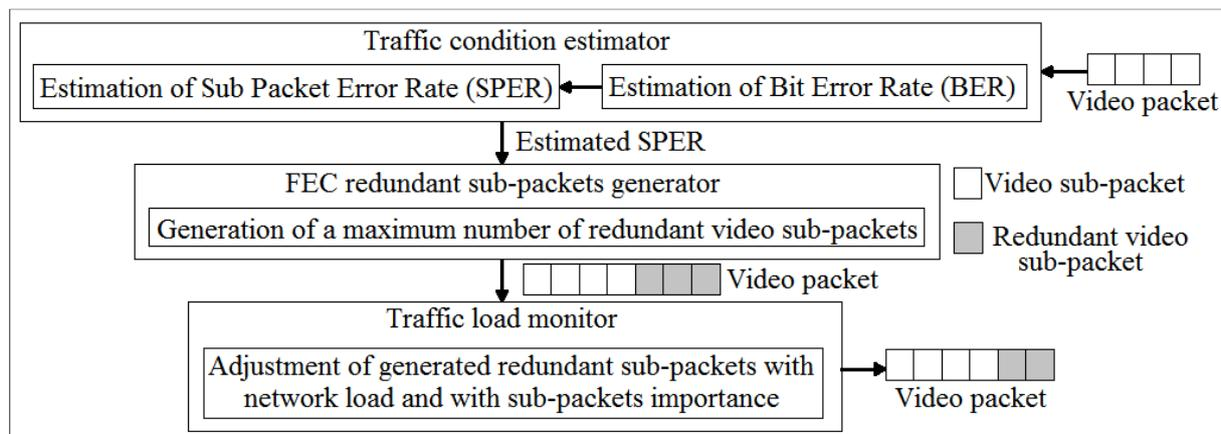
Figure 4.2: Architecture of EASP-FEC mechanism
