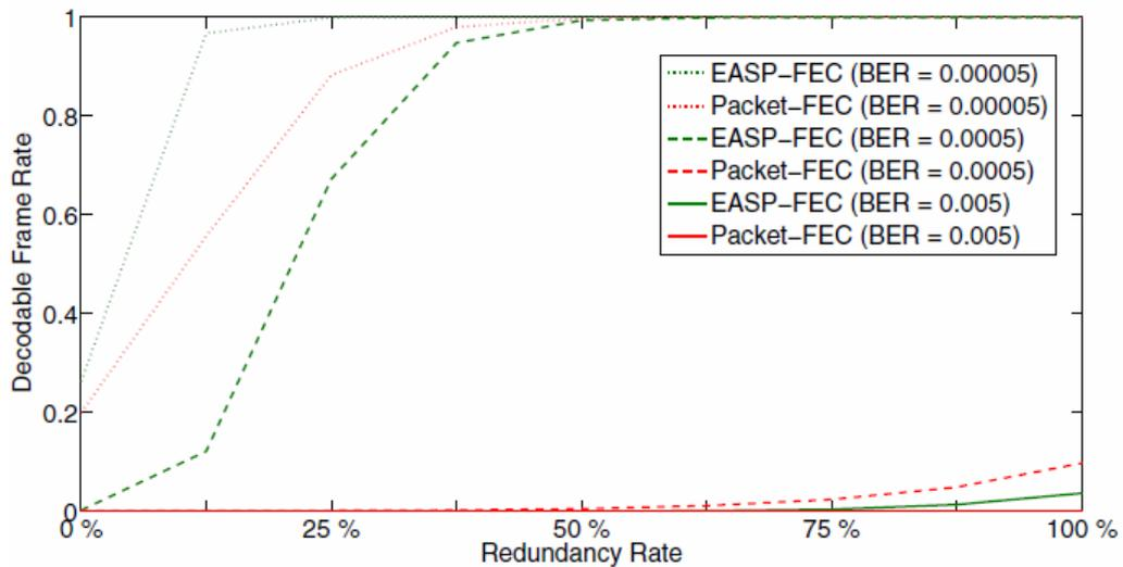
Figure 4.8: Variation of Decodable Frame Rate with Redundancy Rate
