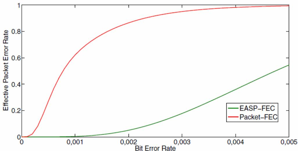
Figure 4.5: Variation of Effective Packet Error Rate with Bit Error Rate
