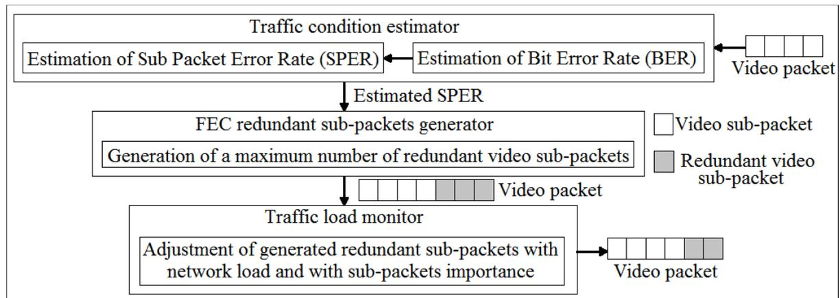
Figure 4.2: Architecture of EASP-FEC mechanism
