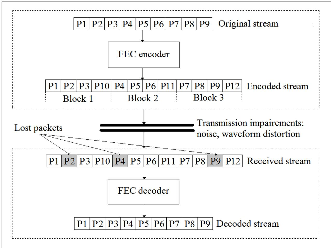
Figure 2.9: An example of Forward Error Correction mechanism
