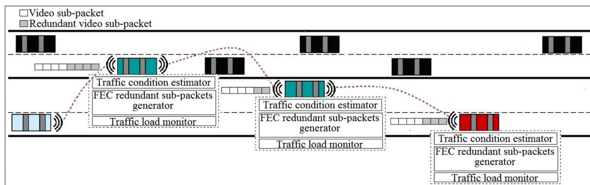
Figure 4.3: Video streaming transmission using EASP-FEC mechanism
