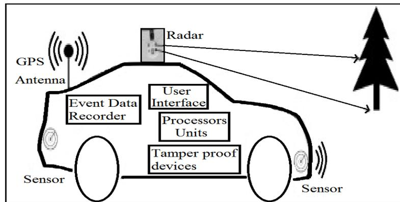
Figure 2.2: Vehicle On-Board Unit
