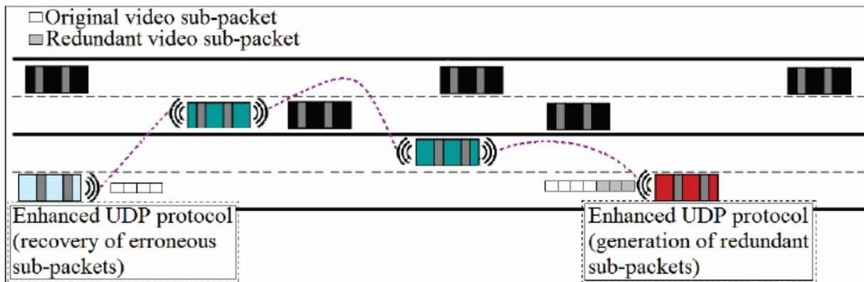
Figure 4.11: Video streaming using EUDP protocol
