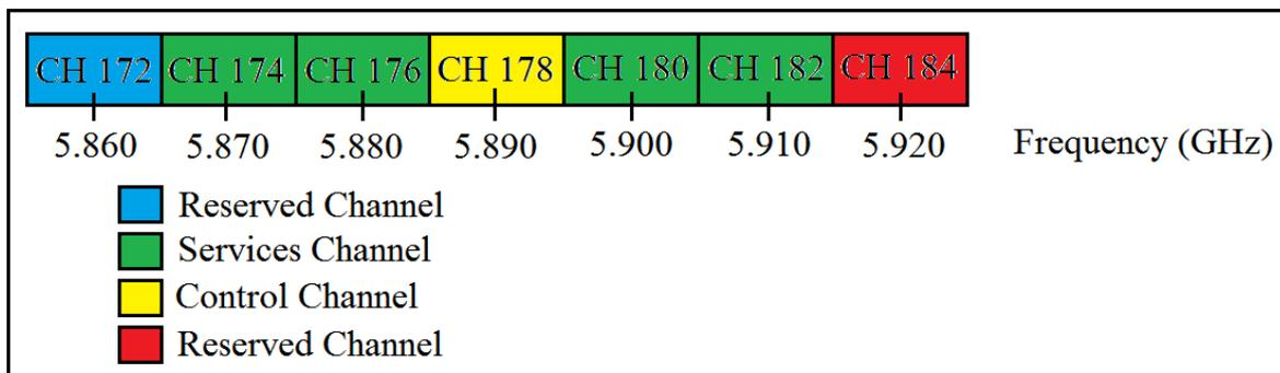
Figure 2.4: DSRC spectrum band for VANET allocated by FCC
