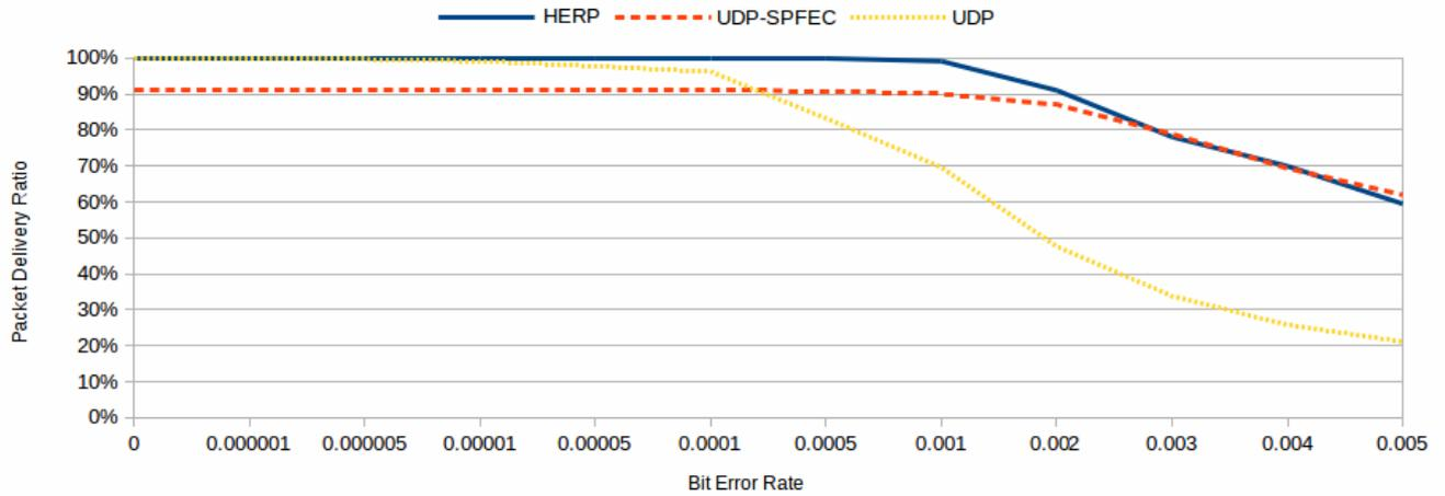
Figure 5.9: Variation of Packet Delivery Ratio with BER
