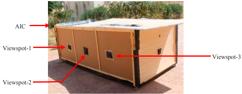
Fig. 1. Physical model with viewspots positions
