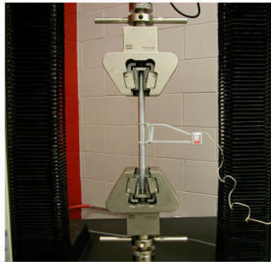
Figure III.7: La machine de traction Zwick/Roell (Z 100).
