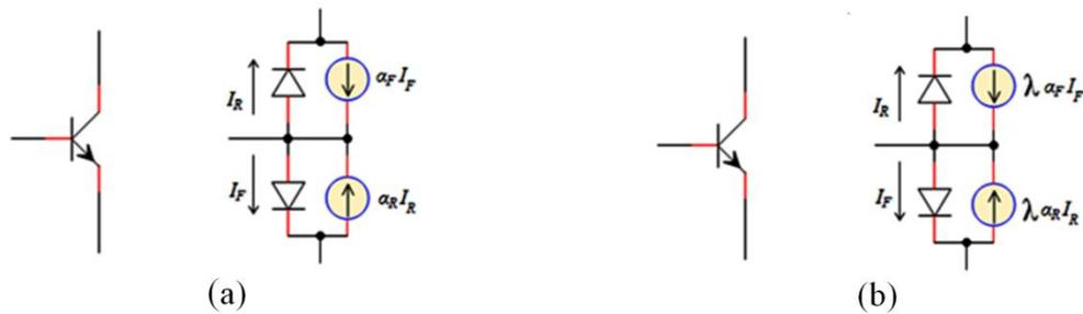
**Fig. II.1.** (a) The Ebers-Moll model for an npn BJT. (b) Reduced the high gain by the homotopy parameter.
