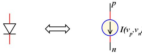
**Fig. IV.13.** The equivalent of diode by dependent voltage source.
