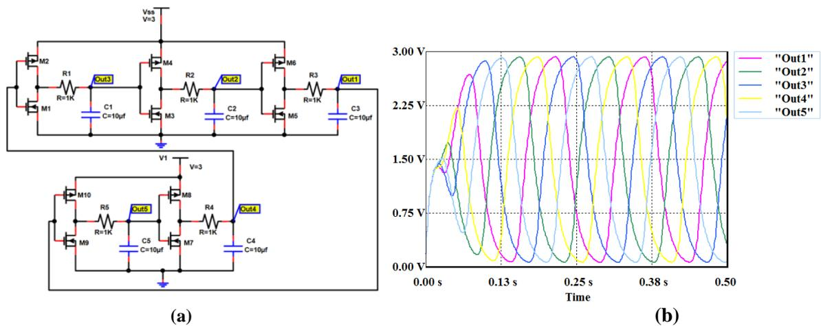
**Fig. IV.35.** Five-stage ring oscillator circuit: (a)- the circuit (b)- simulation results of generation of oscillations in five position of circuit.
