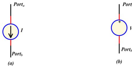
**Fig. IV.8.** Direction of out signal for voltage and current in PyAMS Language.
