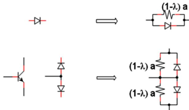
**Fig. II.2.** The position of  $A$  element in semi-conductor device when applying VGH equation.
