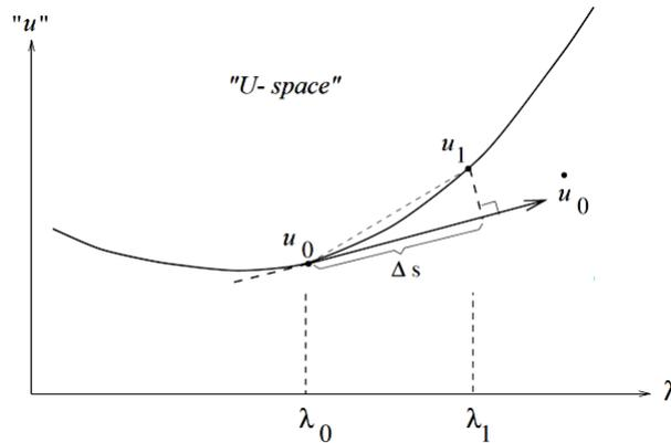
Fig. I.24. Fuses new space (Parameter-independent) pseudo-arclength continuation.
