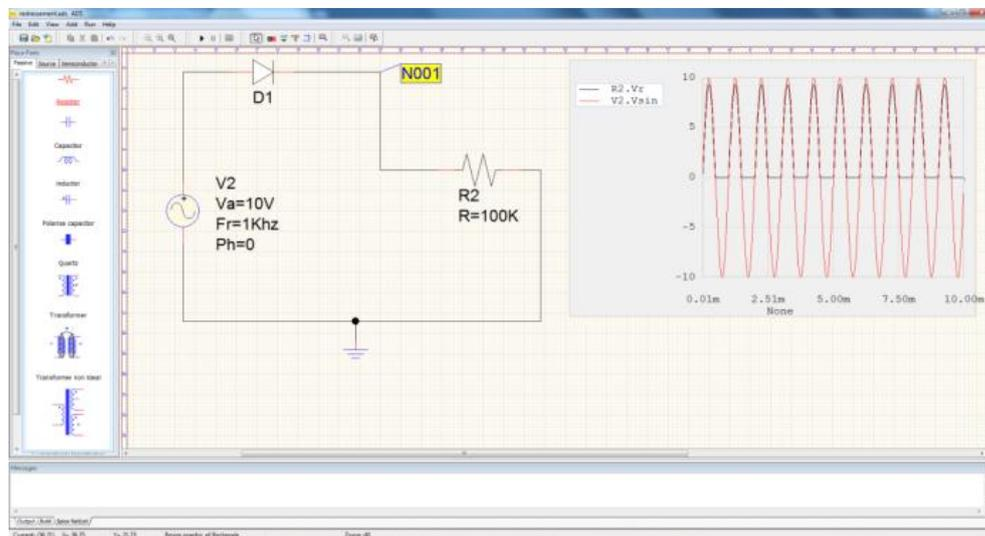
**Fig. IV.24.** The result of simulation presented in schematic editor.
