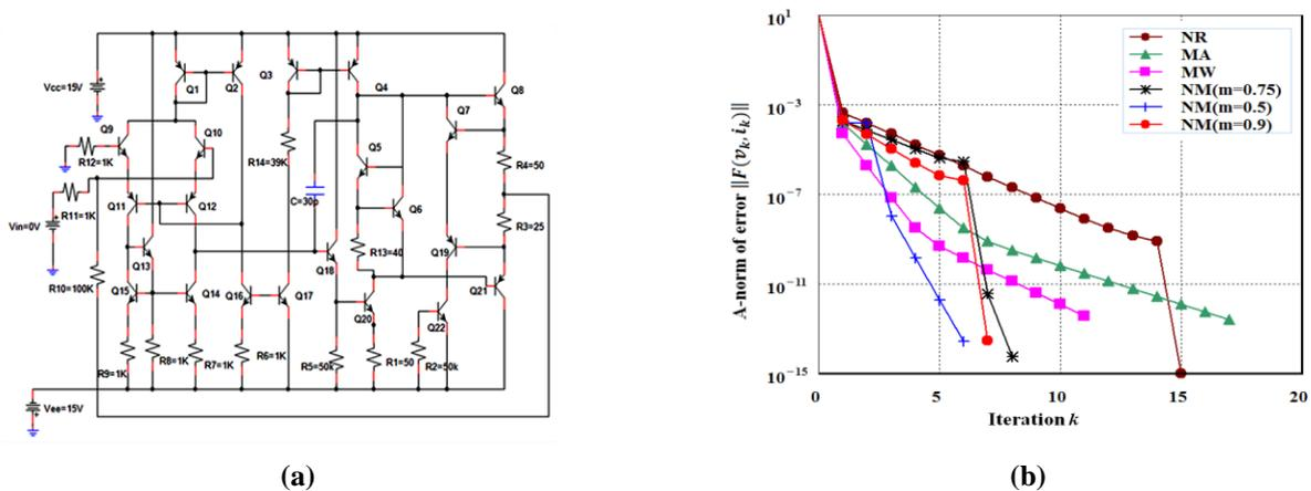
**Fig. III.1.** Operational amplifier  $\mu A741$ : (a) The circuit (b) Convergence the circuit when applying NR, MA, MW and NM.
