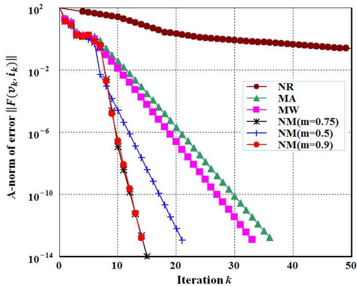
**Fig. III.6.** Six-stage limiting amplifier (6sLA): (a) the circuit (b) convergence the circuit when applying NR ,MA, MW and NM.
