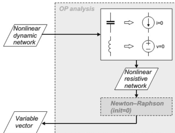
Fig. I.12. Algorithm of operation point [1].
