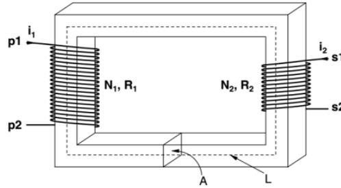
**Fig. IV.32.** A transformer with two windings [1].
