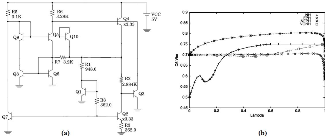
Fig. I.20. Solution curves for the hybrid voltage reference circuit (HVRef): (a) Circuit (b) Solution curves.
