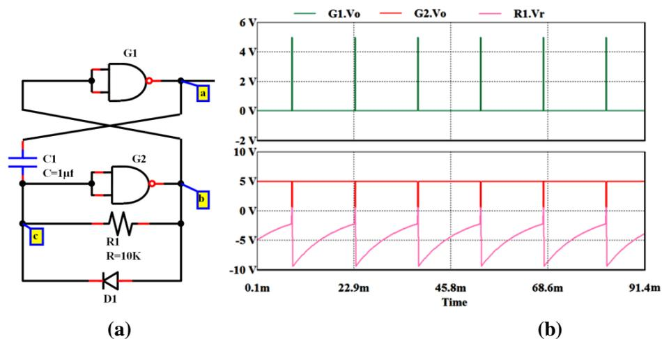
Fig. IV.42. Pulse generator circuit: (a)-the circuit, (b)-simulation results.
