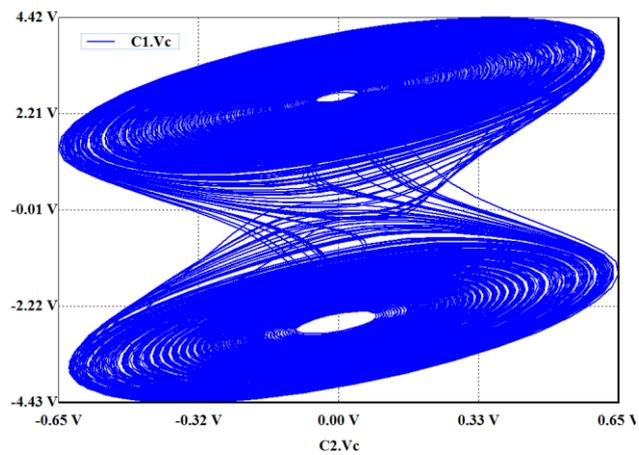
Fig. IV.31. Resulte of simulation of Chua's Diode.
