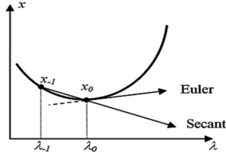
**Fig. II.4.** Calculating the tangent by the secant method and the Euler method.
