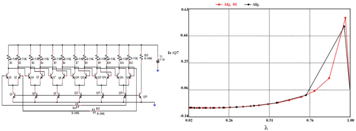
Fig. II.12. The 6sLA circuit: left) the schematic diagram of the circuit, right) the comparison between Alg. 01 and Alg. 02
