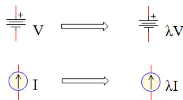
**Fig. I.19.** The equivalent of current source and voltage source when applying the stepping in the source.
