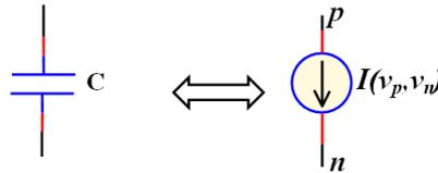
**Fig. IV.12.** The equivalent of capacitor by dependent current source.
