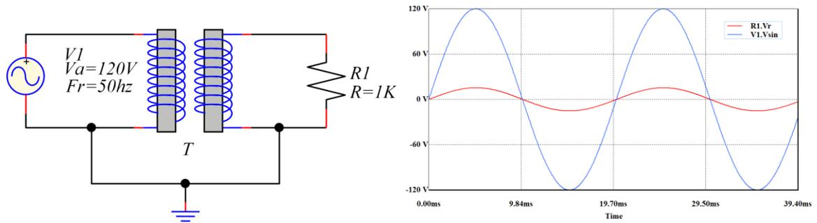
**Fig. IV.34.** Response to sinusoidal voltage at the primary coil of nonlinear transformer.
