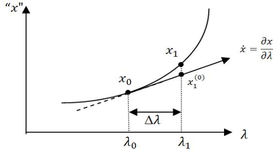
**Fig. IV.3.** Predictor-corrector method ( $x = v \cup i$ )
