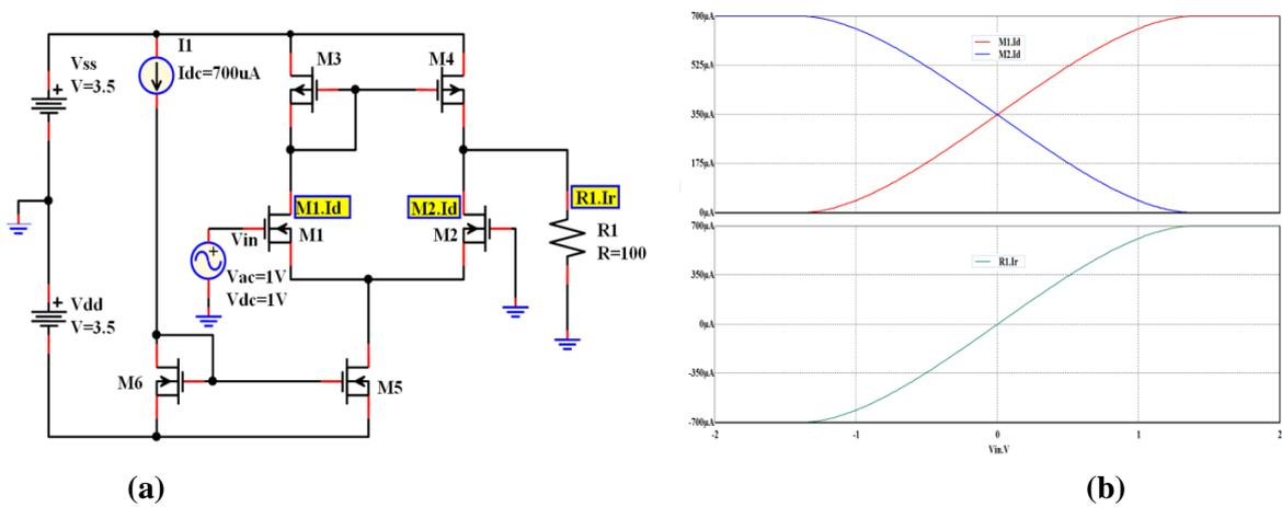
Fig. IV.40. Operational transconductance amplifier (OTA): (a)- the circuit (b)-simulation results of output current in drin of M1 with M2 and resistor dependent by input voltage.
