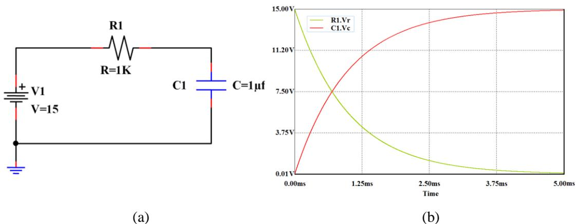
**Fig. IV.26.** (a) Simple RC circuit. (b) Simulation results of RC circuit.
