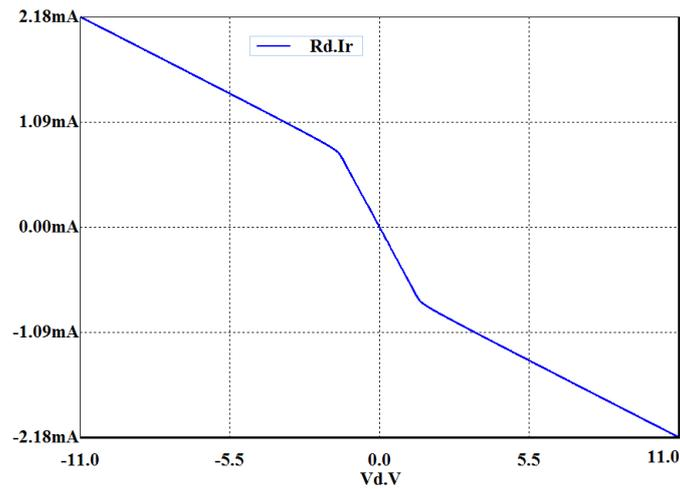
Fig. IV.30. Characteristic of Chua's Diode
