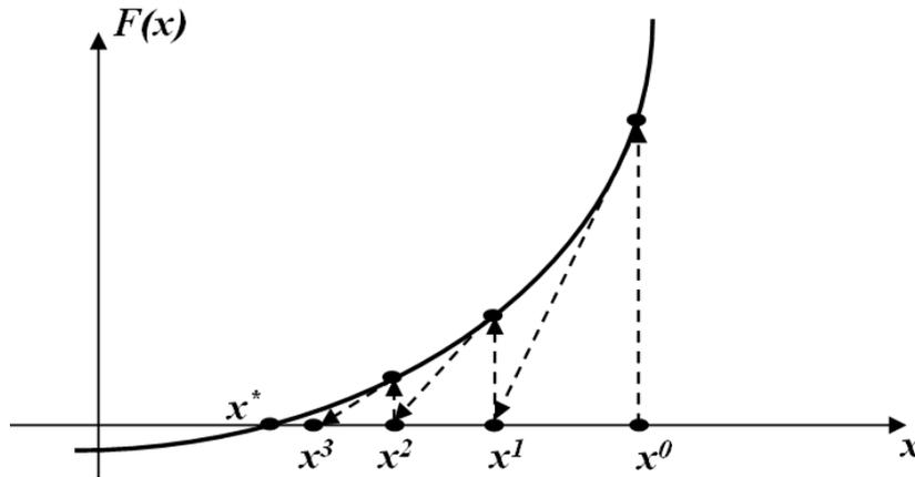
Fig. I.1. The successful case for Newton-Raphson method.
