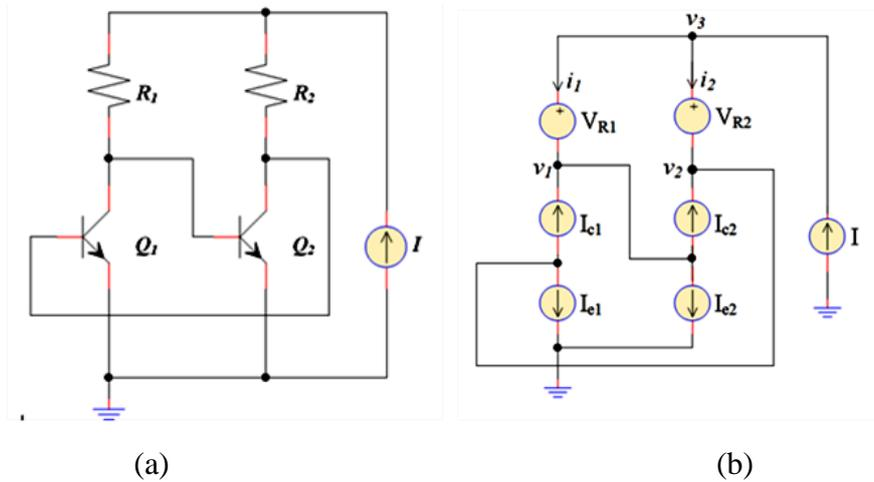
**Fig. II.10.** Example of a circuit: a) Simple oscillator circuit with BJTs, b) The equivalent of the circuit using dependent source
