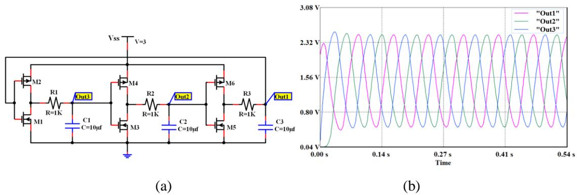
Fig. IV.28. Oscillator circuit: (a) the schema of circuit (b) the result of simulation in mode TR.
