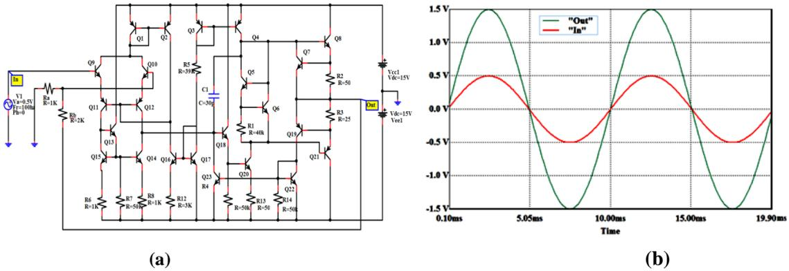
Fig. IV.36. The LM741 non-inverting Amplifier circuit: (a)- the circuit, (b)- the waveforms for LM741 input and output
