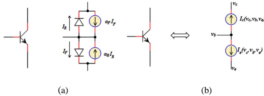
**Fig. II.7.** (a) The Ebers-Moll model for an npn BJT. (b)The equivalent of BJT by dependent current source.
