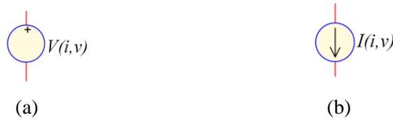
**Fig. IV.1.** Dependent sources: (a) voltage source, (b) current source.
