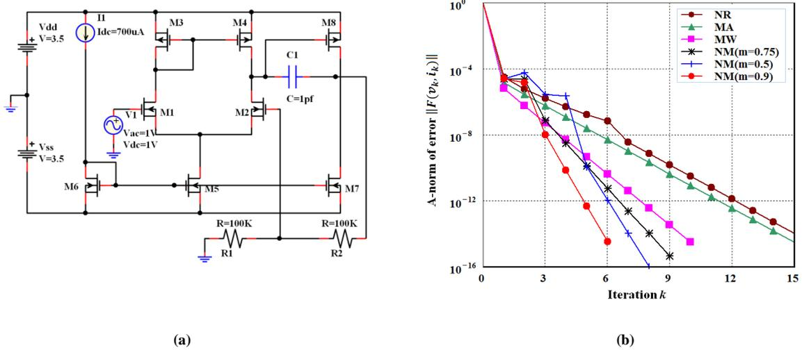
**Fig. III.5.** Operational transconductance amplifier (OTA) with outstage : (a) the circuit (b) convergence the circuit when applying NR ,MA, MW and NM.
