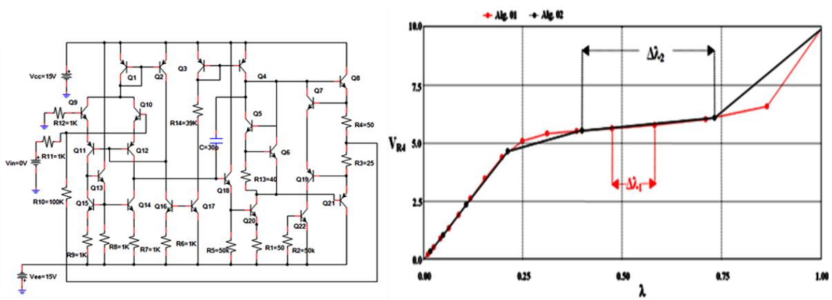
Fig. II.13. The  $\mu$ A741 circuit: left) the schematic diagram of the circuit, right) the comparison between Alg. 01 and Alg. 02
