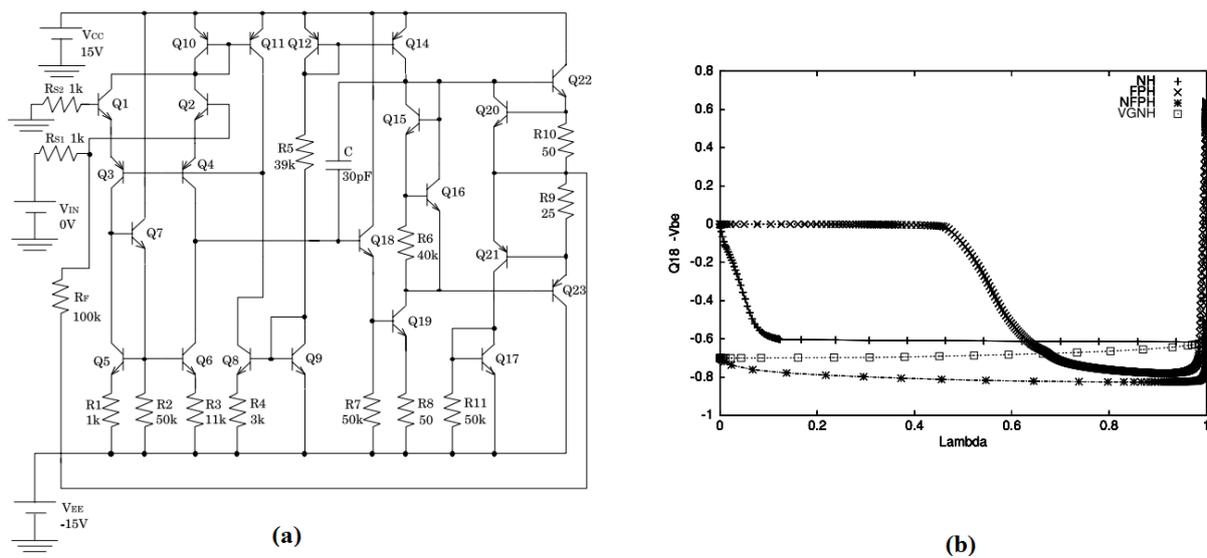
Fig. I.21. Solution curves for the high gain operational amplifier: (a) Circuit (b) Solution curves.
