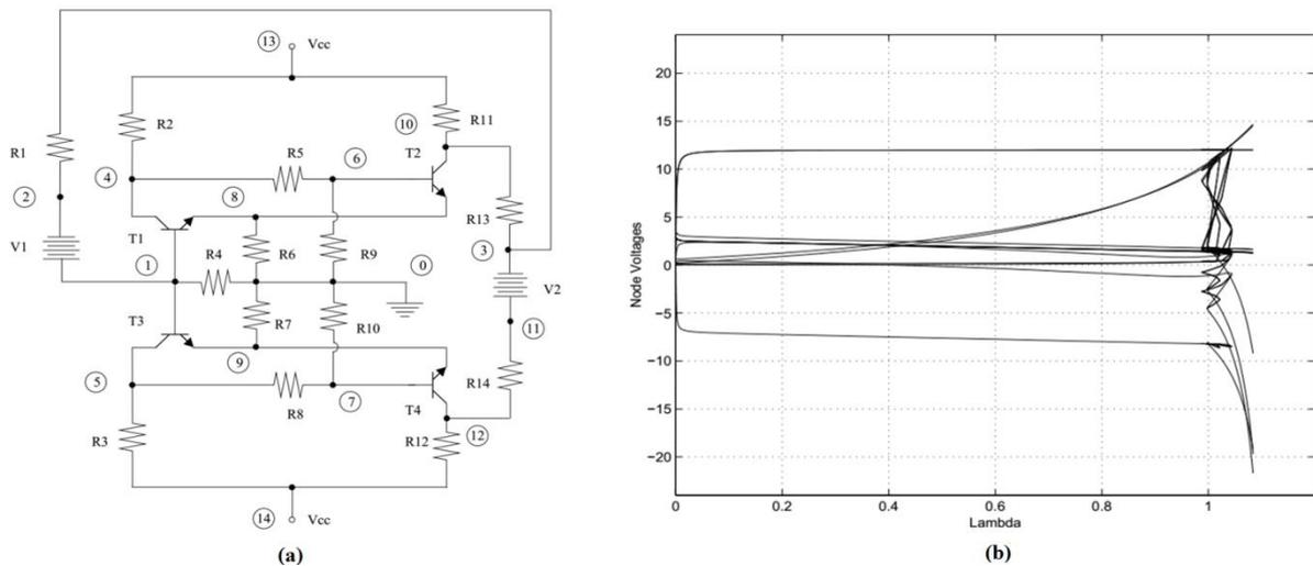
**Fig. I.25.** (a) Four-transistor circuit that has nine dc operating points. (b) Homotopy paths for the fourteen node voltages of the four-transistor circuit [28,29].
