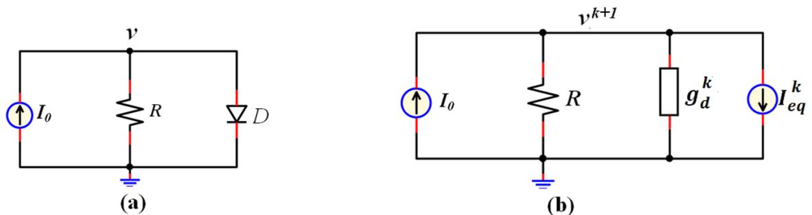
**Fig. I.9.** Example of circuit : (a)-Nonlinear circuit. (b)-The linear circuit of (a) by NR.
