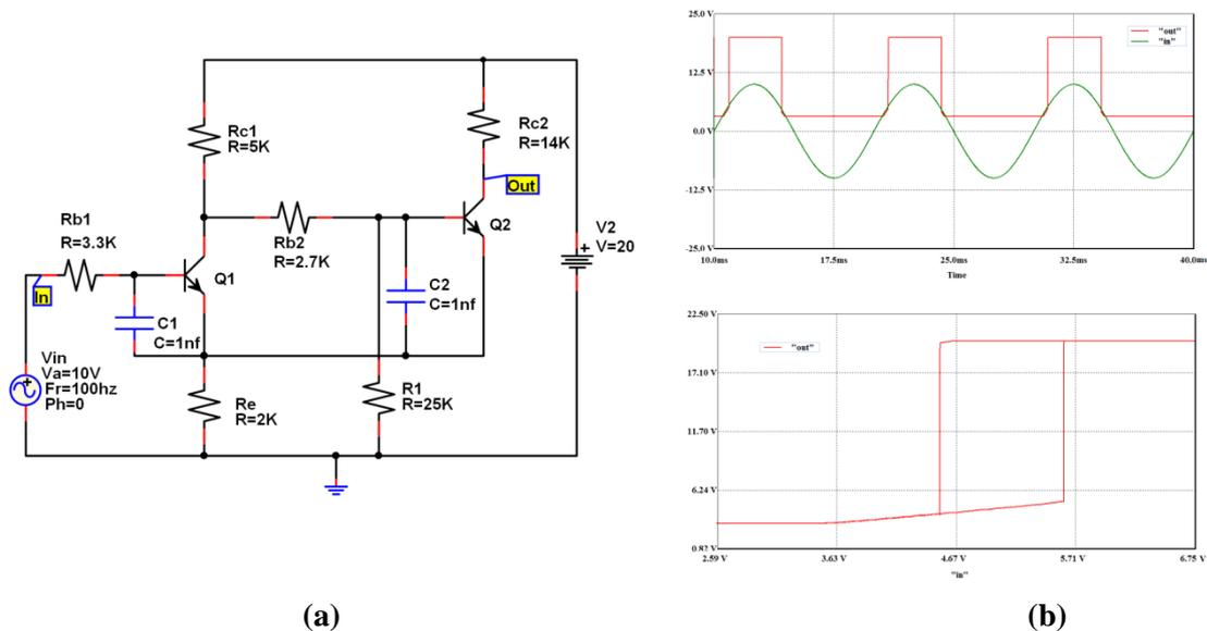
Fig. IV.38. Schmitt trigger circuit: (a)- the circuit (b)-simulation results of comparator input signal presented by output and curve non-inverting of schmitt trigger.
