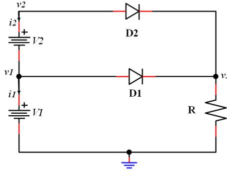
Fig. I.3. Example of nonlinear circuit with two diodes.
