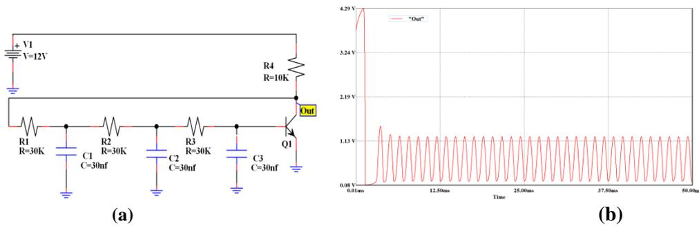
Fig. IV.37. Phase-shift oscillator circuit: (a)- the circuit (b)-simulation results of oscillation in “out” of circuit.
