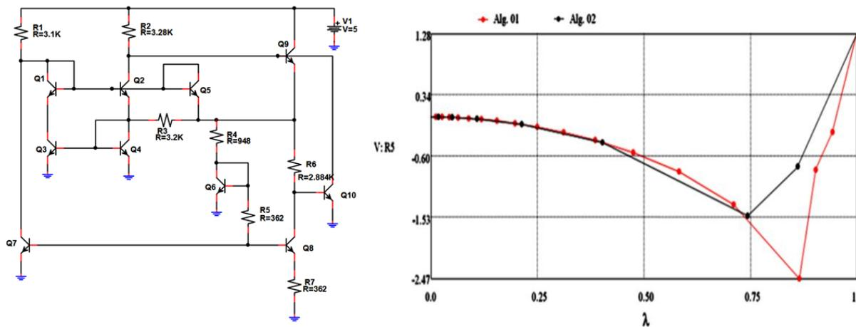
**Fig. II.11.** The HVRef circuit: left) the schematic diagram of the circuit, right) the comparison between Alg. 01 and Alg. 02
