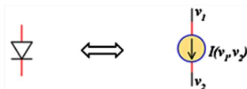
**Fig. II.6.** The equivalent of diode by dependent voltage source.
