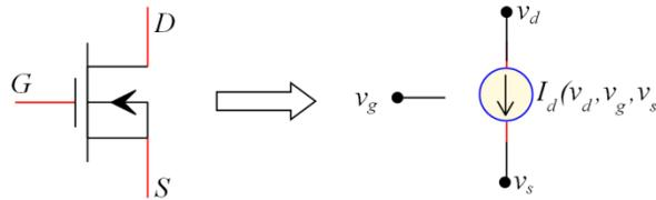
**Fig. II.9.** The equivalent of NMOS by dependent current source.
