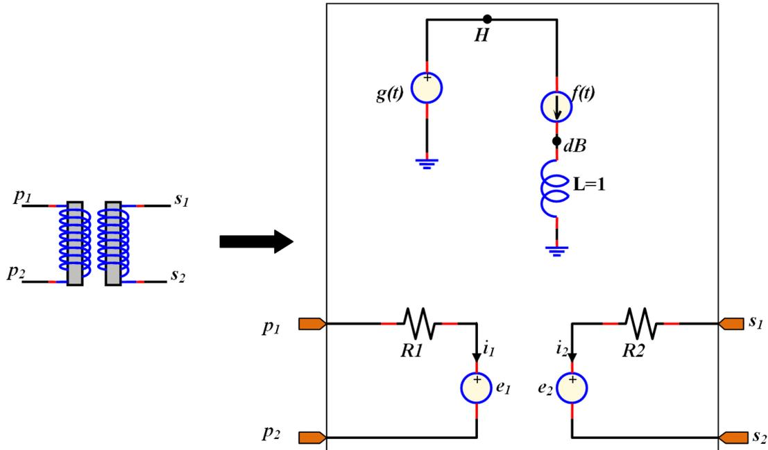
**Fig. IV.33.** A nonlinear transformer symbol (left) and the corresponding model (right).
