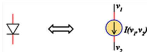
**Fig. II.6.** The equivalent of diode by dependent voltage source.
