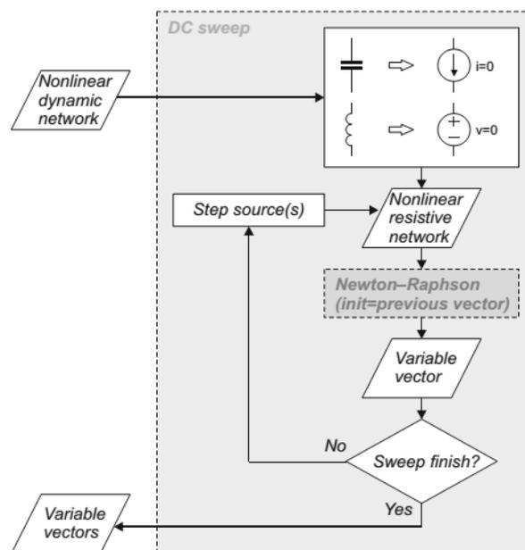
Fig. I.13. Algorithm of DC sweep analysis [1].
