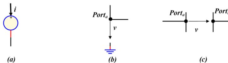
**Fig. IV.9.** Direction of in signal for voltage and current in PyAMS Language.
