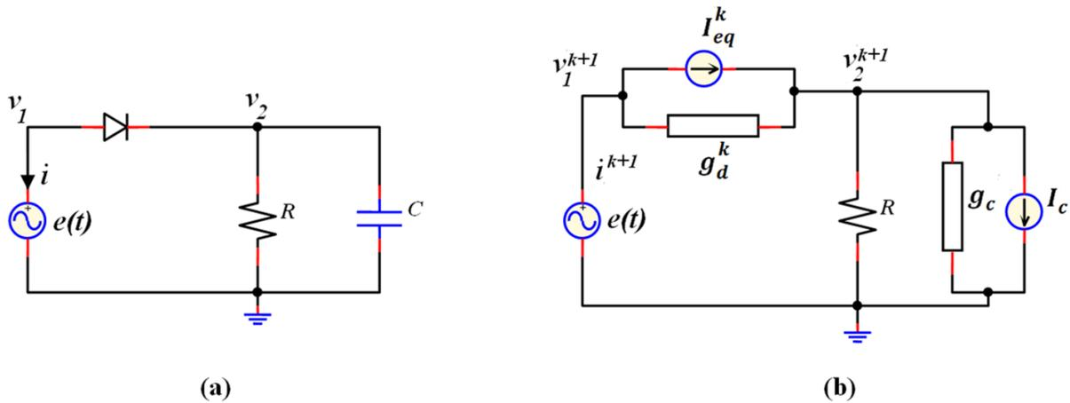
**Fig. I.10.** Example of circuit : (a)- circuit Nonlinear with dynamique element.
