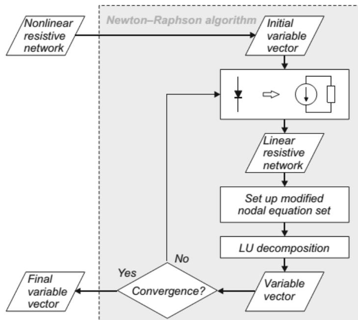
**Fig. I.11.** Algorithm of Newton-Raphson [1].
