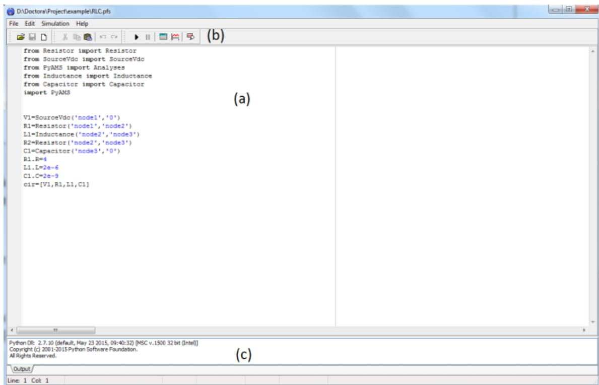
**Fig. IV.19.** The interface for design of circuit by textual method: (a) Editeur of texte. (b) Command of : editing, compilation and analyses. (c) Output messages.
