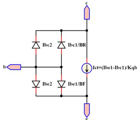
Fig. IV.15. Bipolar Transistor npn Model type Gummel-Poon without substrate.
