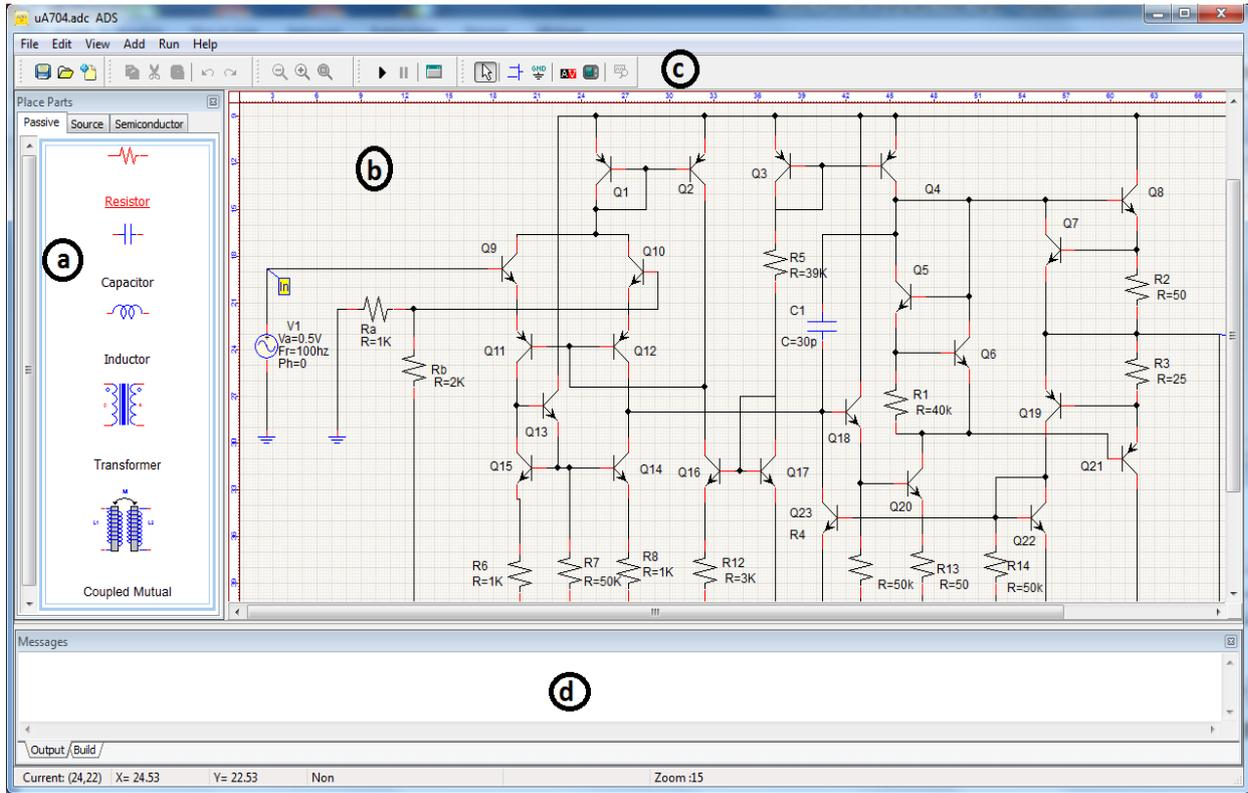
**Fig. IV.20.** The Interface for design circuit by schema method: (a) List of Parts. (b) Schematic editor. (c) Command of: add wires and parts, compilation and analyzing. (d) Out messages.
