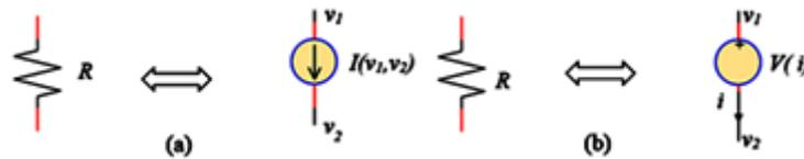
**Fig. II.5.** The equivalent of resistor: (a) dependent current source. (b) dependent voltage source.
