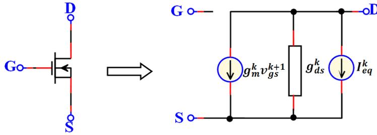
Fig. I.5. The linear of NMOS model by application of NR.
