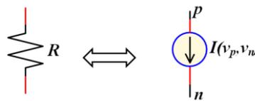
**Fig. IV.10.** The equivalent of resistor by dependent current source.
