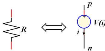
**Fig. IV.11.** The equivalent of resistor by dependent voltage source.
