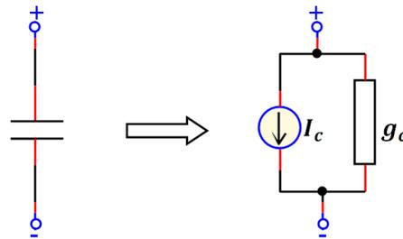
**Fig. I.8.** Linear companion model for capacitor.
