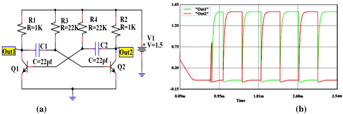
Fig. IV.41. Astable multivibrator circuit: (a)-the circuit (b)-simulation results of astable multivibrator circuit presented in two output.
