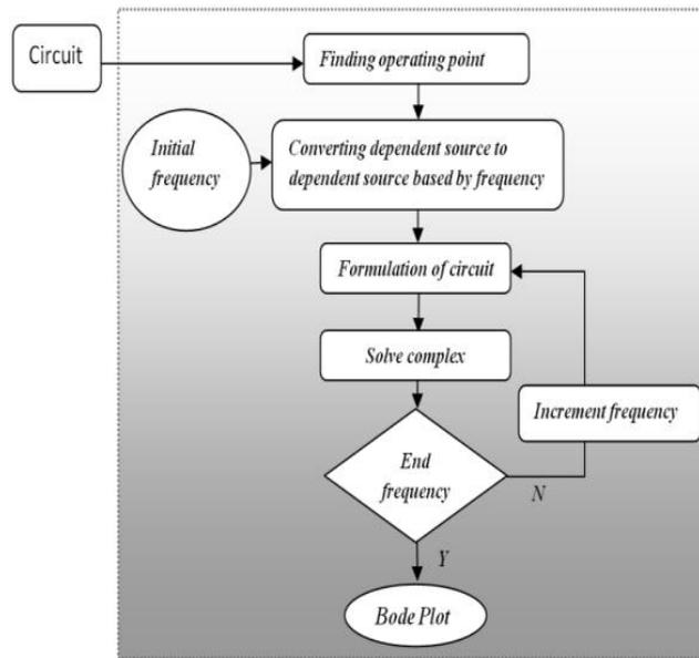
Fig. IV.7. Algorithm small signal AC analysis.
