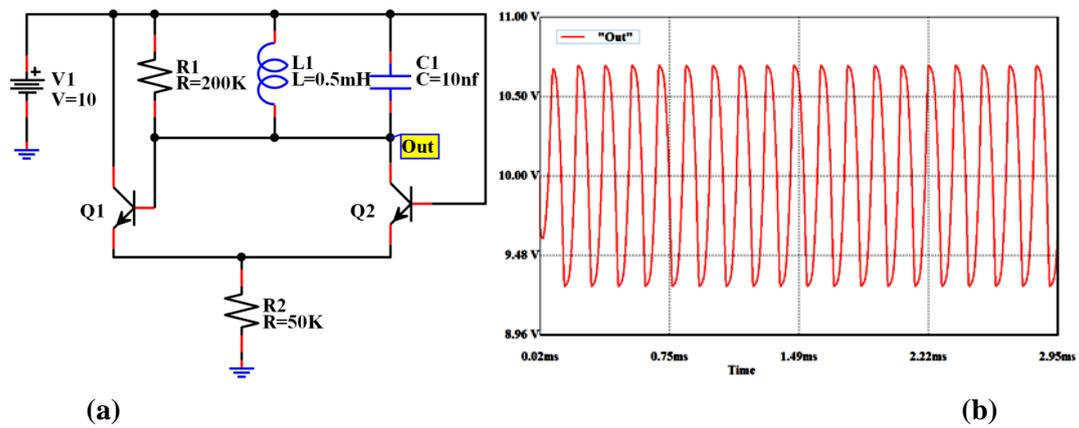
Fig. IV.39. The Peltz oscillator Circuit: (a)- the circuit, (b)- simulation results.
