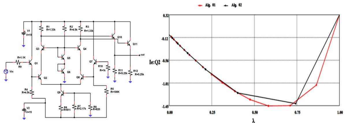
Fig. II.14. The RCA3040 circuit: left) the circuit, right) the comparison between Alg. 01 and Alg.02
