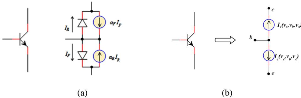
**Fig. IV.14.**(a)The Ebers-Moll model for an npn BJT. (b)The equivalent of BJT by dependent current source.
