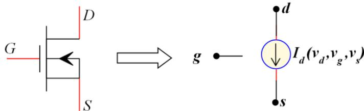
**Fig. IV.17.** The equivalent of NMOS by dependent current source
