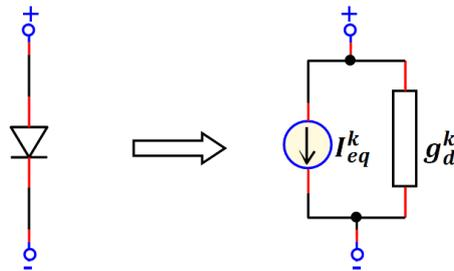
**Fig. I.4.** The linear of diode model by application of NR.
