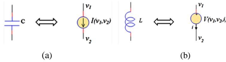
**Fig. II.8.** (a) The equivalent of capacitor by dependent current source. (b) The equivalent of inductance by dependent voltage source.
