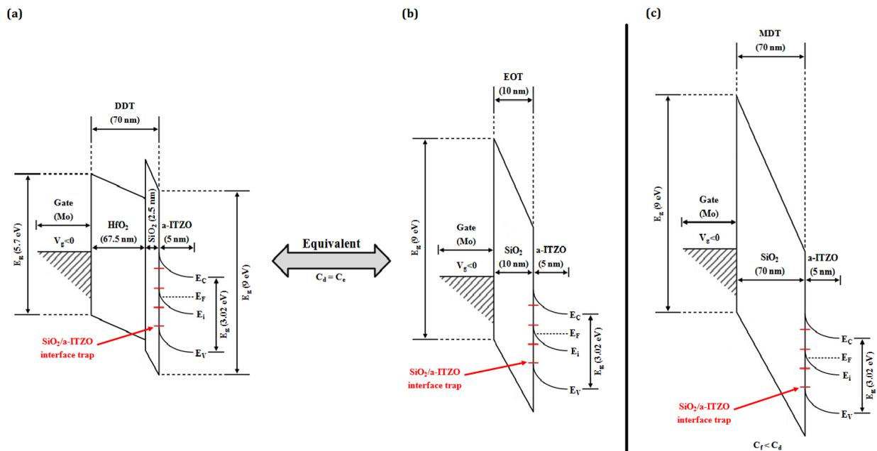
Figure III.12 Schematic band energy diagram of the channel/dielectric interface in the a-ITZO TFT with (a) 70 nm of the bi-layer SiO<sub>2</sub>/HfO<sub>2</sub> gate dielectric, (b) the equivalent 10 nm of SiO<sub>2</sub> without ALE and (c) 70 nm of SiO<sub>2</sub> mono-layer.
