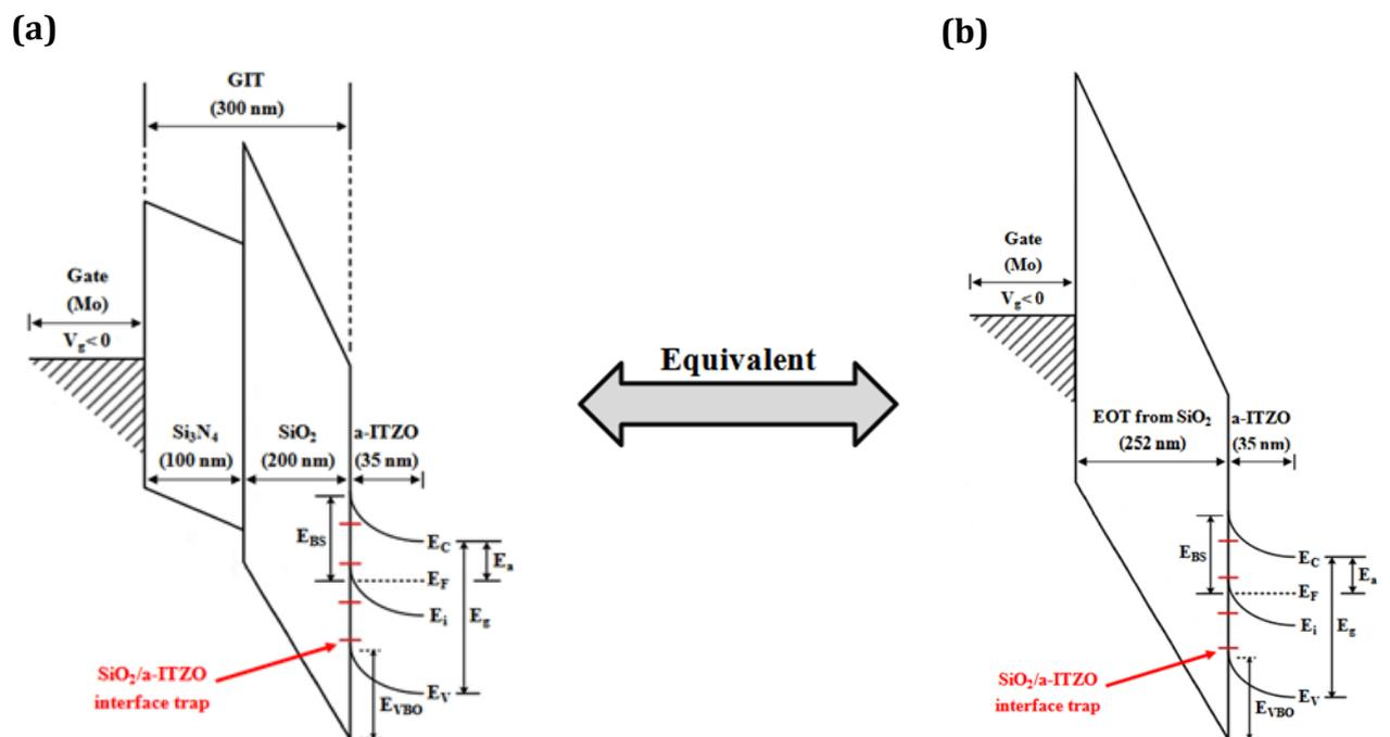
Figure I.10 The energy band diagram of the semiconductor/dielectric interface in a-ITZO TFT where (a) shows the energy band diagram of the semiconductor/double-layered dielectric oxide (a-ITZO/SiO<sub>2</sub>/Si<sub>3</sub>N<sub>4</sub>) interface in a-ITZO TFT while (b) shows the energy band diagram of the semiconductor/mono-layer equivalent dielectric oxide (a-ITZO/equivalent SiO<sub>2</sub>) interface in a-ITZO TFT [1].
