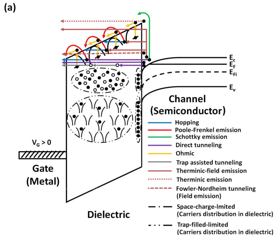
Figure III.20 The energy band diagram of the semiconductor/dielectric interface in TFT depending on the type of gate bias with most leakage mechanisms that can contribute to the charge leakage through the gate dielectric.
