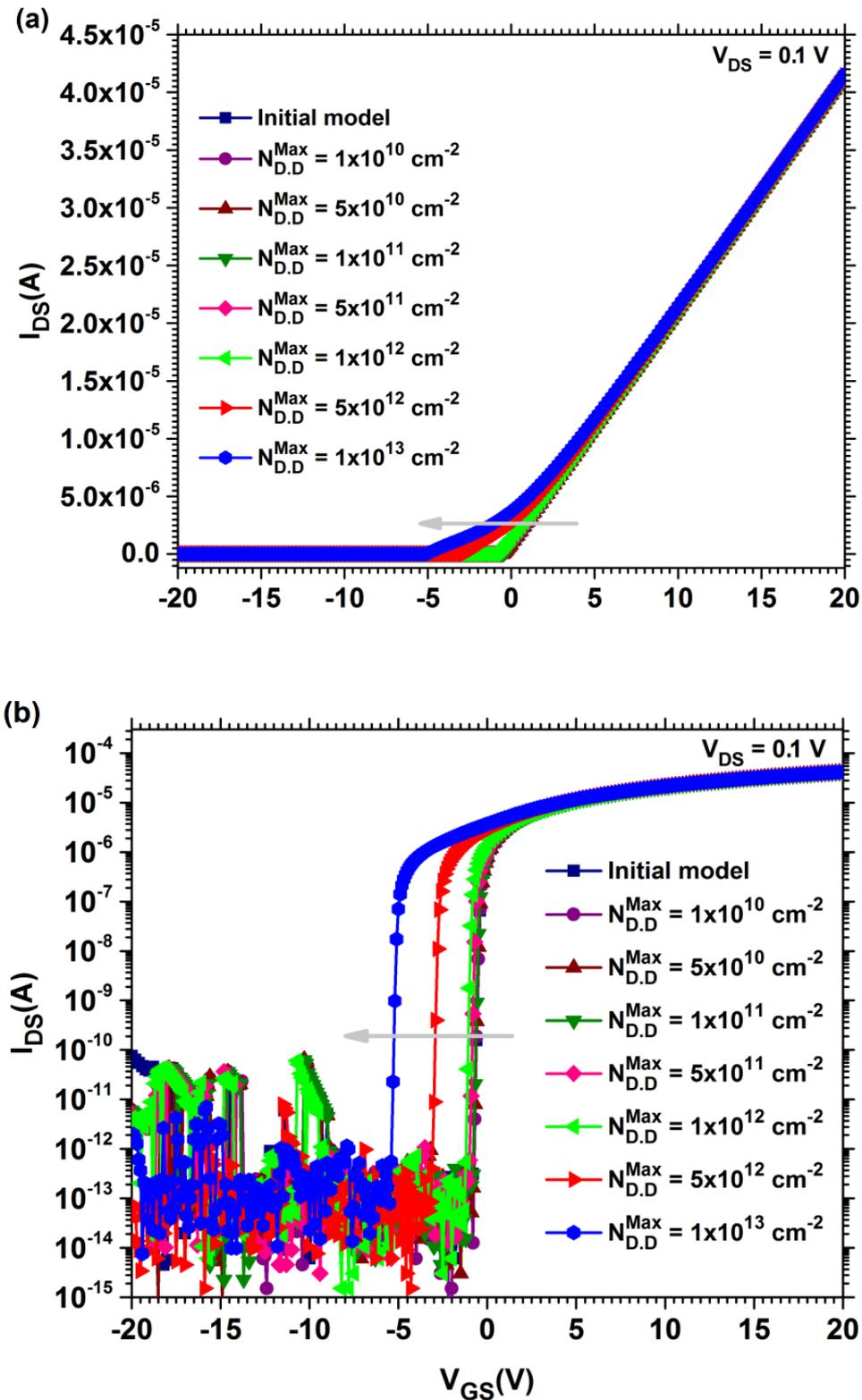
Figure III.16 Transfer ( $I_{DS} - V_{GS}$ ) characteristics of the a-ITZO TFT with bi-layer ( $\text{SiO}_2/\text{HfO}_2$ ) gate dielectric: (a) linear plot and (b) semi-logarithmic plot, for different  $\text{SiO}_2/\text{HfO}_2$  interface state densities.
