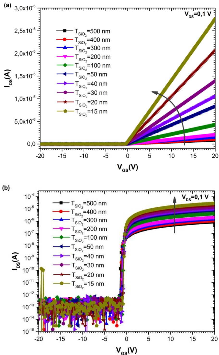
Figure III.6 The transfer ( $I_{DS} - V_{GS}$ ) characteristics of the a-ITZO TFT depending on the SiO<sub>2</sub> gate dielectric thicknesses; (a) in the linear plot and (b) in the semi-logarithmic plot.
