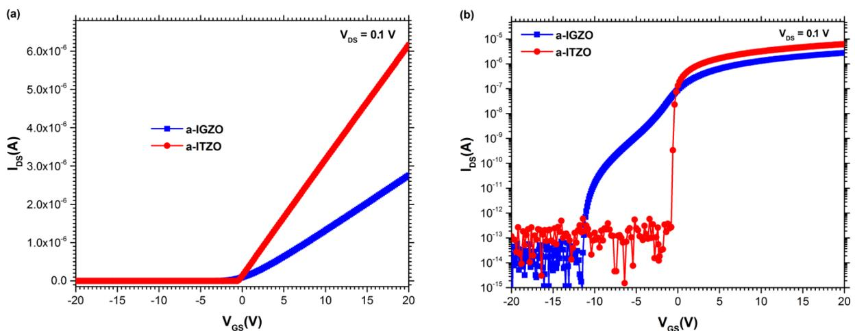
Figure III.2 The calculated of transfer ( $I_{DS} - V_{GS}$ ) characteristics of the a-IGZO and a-ITZO TFTs where (a) shows the evolution of the transfer characteristics in the linear plot while (b) shows the evolution of the transfer characteristics in the semi-logarithmic plot.
