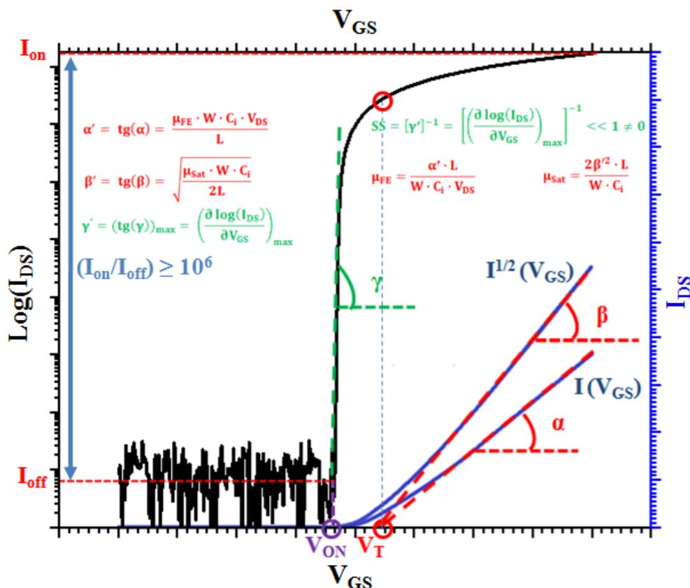
Figure I.6 The extraction methods of the a-ITZO TFT output parameters.
