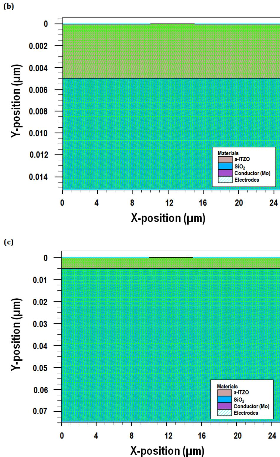
Figure III.11 Schematic diagram of the two-dimensional cross-section of the bottom-gate a-ITZO TFT structures generated by Silvaco Atlas depending on the different types of gate dielectrics: (a) 70 nm of the bi-layer low-k(SiO<sub>2</sub>)/high-k(HfO<sub>2</sub>) gate dielectric, (b) the equivalent 10 nm of SiO<sub>2</sub> without ALE and (c) 70 nm of low-k SiO<sub>2</sub> gate dielectric.
