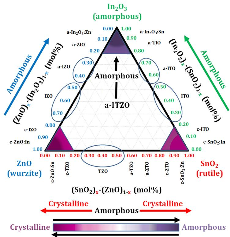
Figure I.3 The ternary diagram of TCOs in  $\text{In}_2\text{O}_3\text{-SnO}_2\text{-ZnO}$  system where (a) shows crystalline phase diagram of TCOs in  $\text{In}_2\text{O}_3\text{-SnO}_2\text{-ZnO}$  system and (b) shows some TCO semiconductors of this material family [15, 25].
