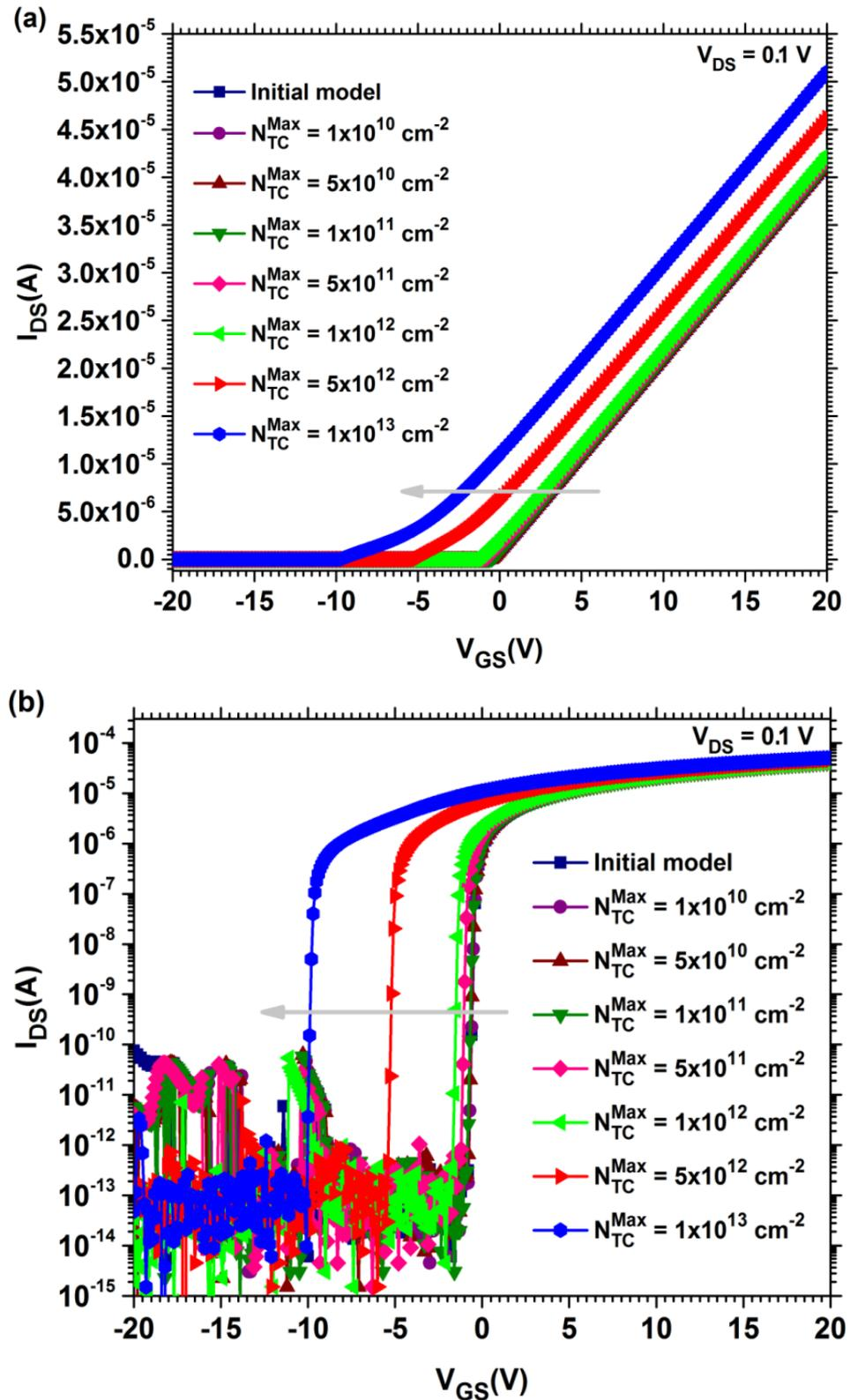
Figure III.17 Transfer characteristics of the a-ITZO TFT with bi-layer SiO<sub>2</sub>/HfO<sub>2</sub> gate dielectrics:
