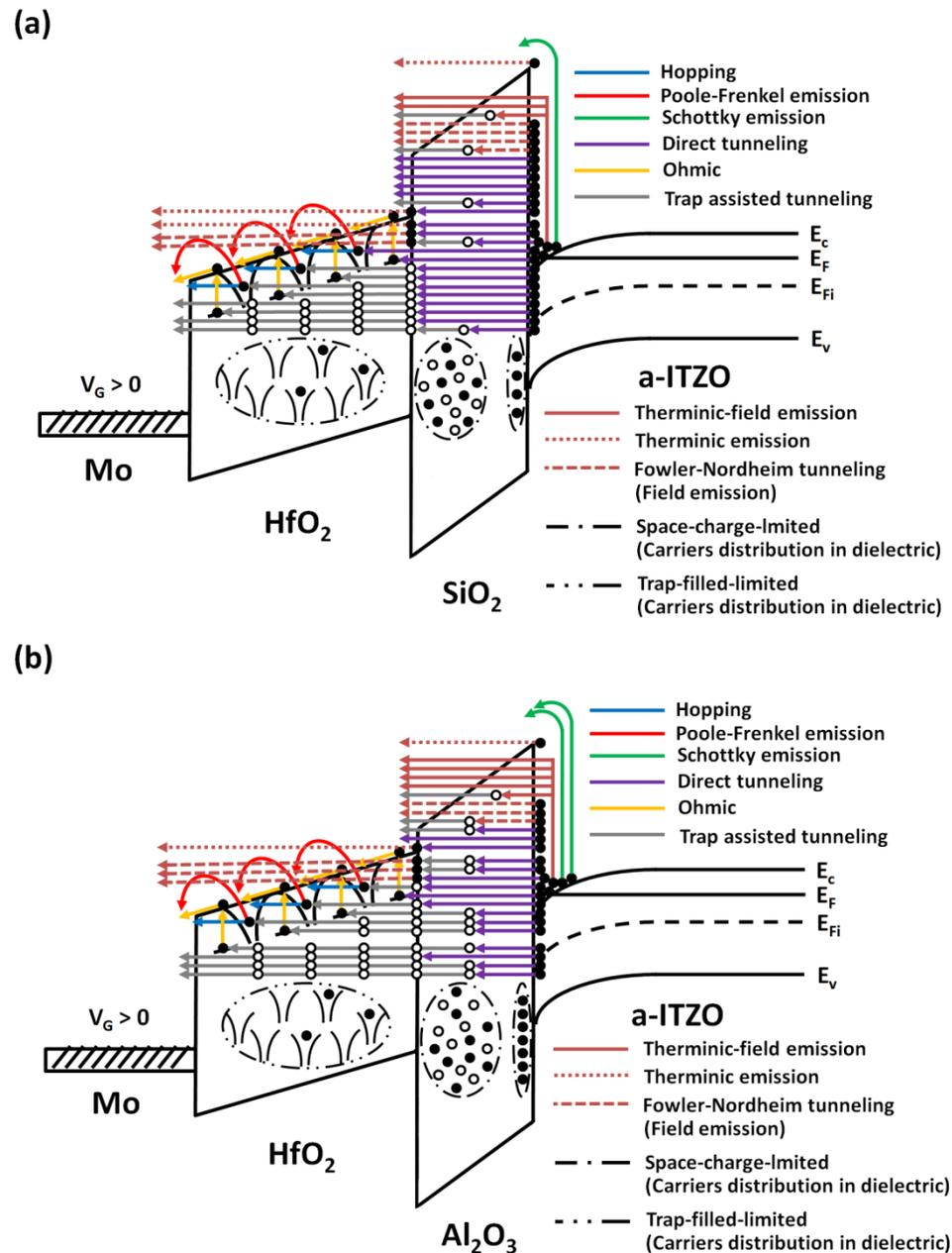
Figure III.23 The energy band diagram of the semiconductor/dielectric interface in TFTs with different leakage mechanisms that contribute to the charge leakage through the gate dielectric depending on the different types of the interfacial dielectrics: (a) with an interfacial low-k SiO<sub>2</sub> and (b) with an interfacial high-k Al<sub>2</sub>O<sub>3</sub>.
