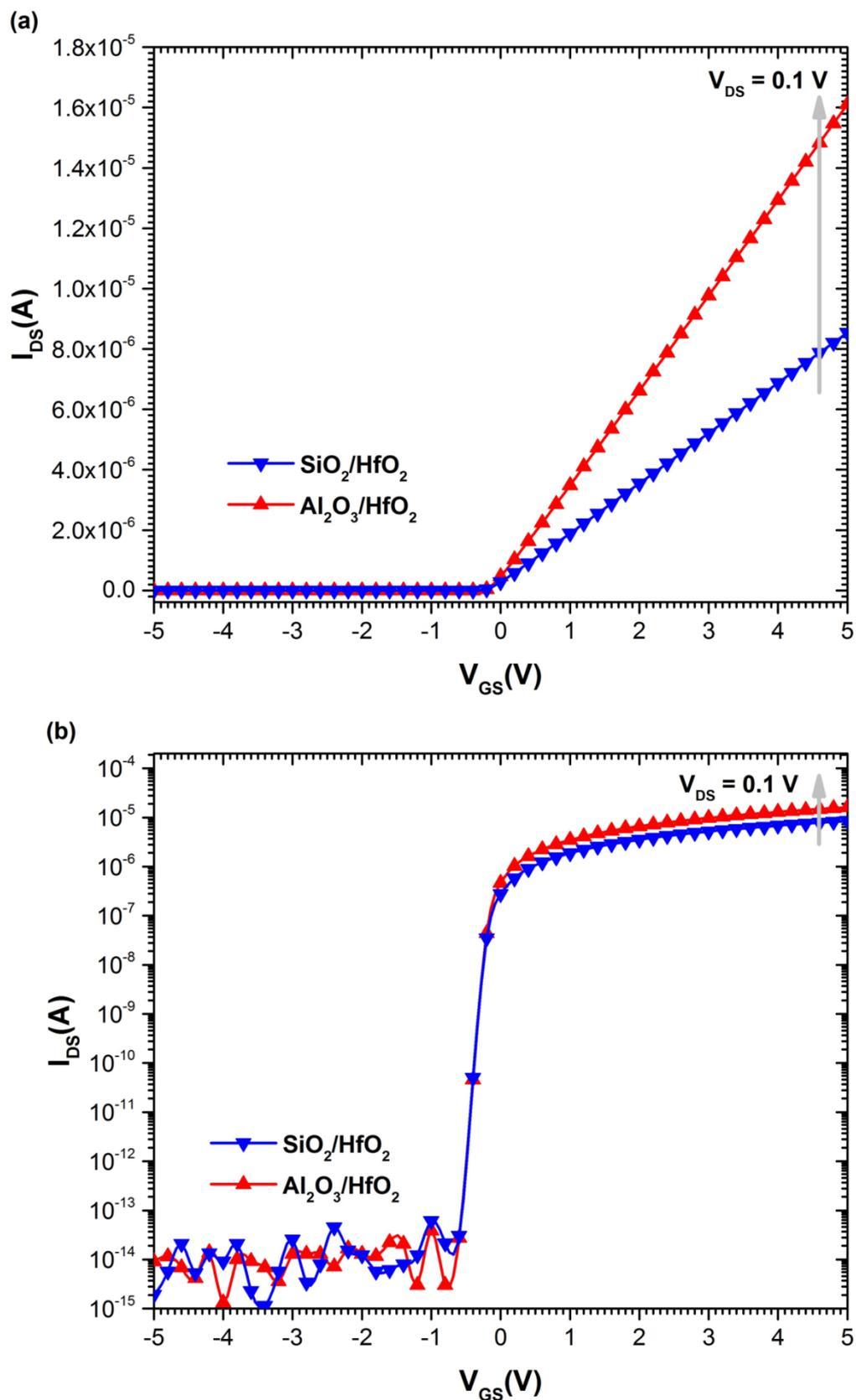
Figure III.19 The calculated of transfer ( $I_{DS} - V_{GS}$ ) characteristics of the a-ITZO TFT depending on the different types of the interfacial dielectrics: (a) transfer characteristics in the linear plot and (b) transfer characteristics in the semi-logarithmic plot.
