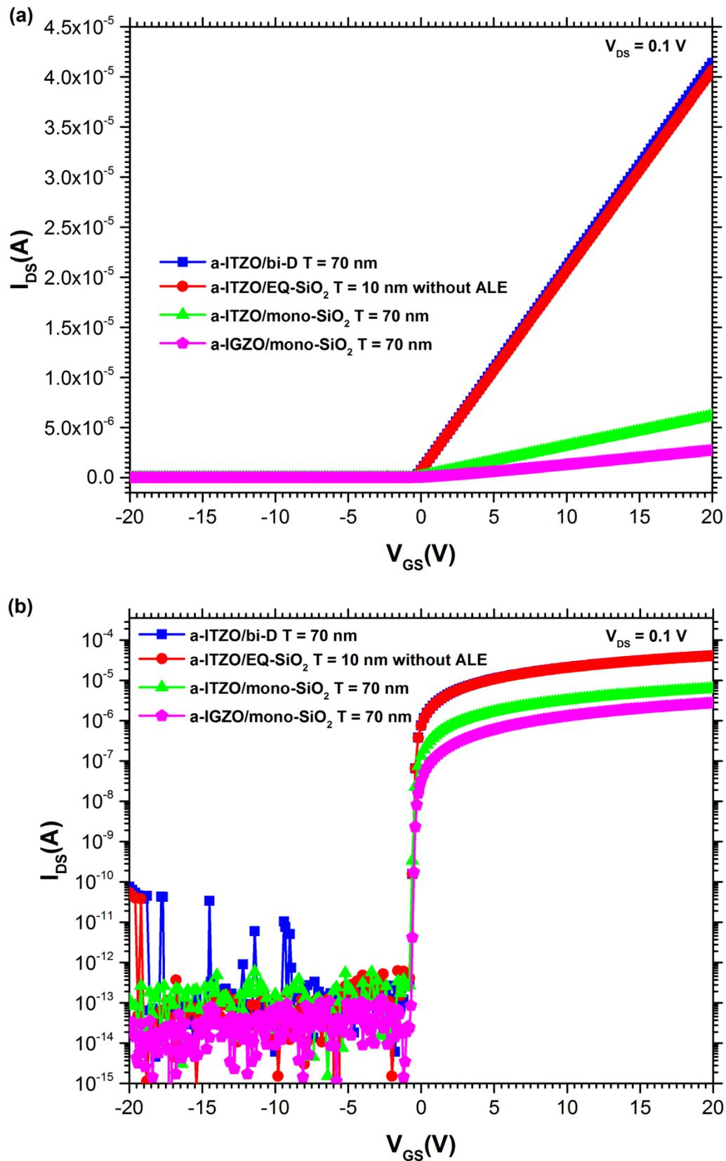
Figure III.13 The simulated a-ITZO TFT transfer ( $I_{DS} - V_{GS}$ ) characteristics for the different types of the gate dielectrics: (a) in the linear plot and (b) in the semi-logarithmic plot.
