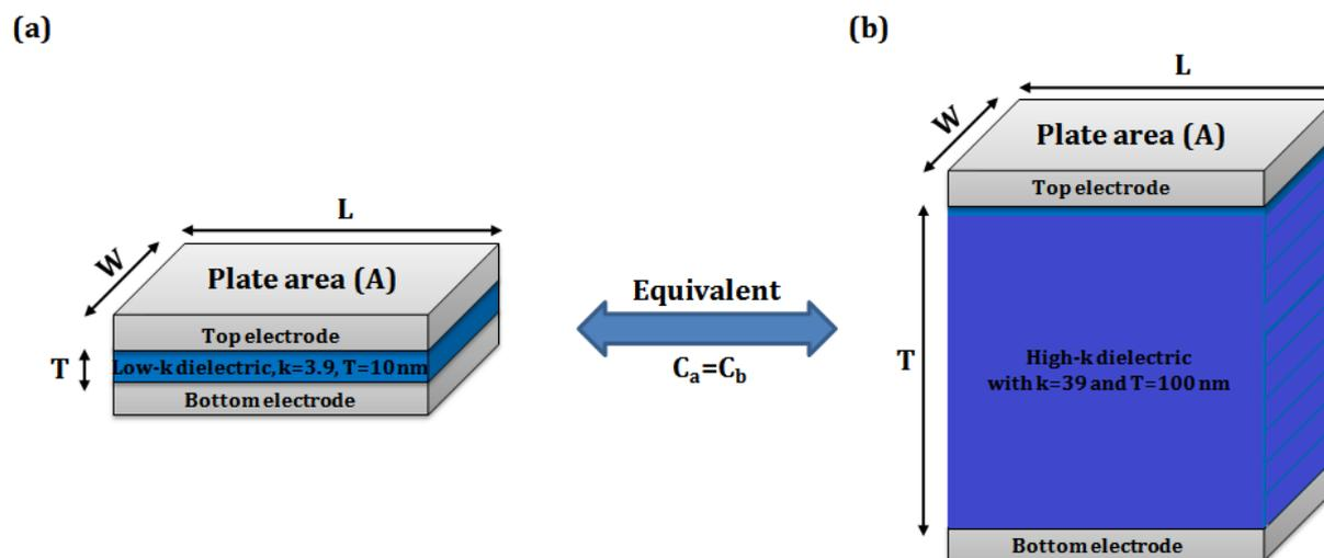
Figure I.9 Simplified representation of the three-dimensional parallel plate capacitor (a) with a low-k dielectric and (b) with a high-k thicker dielectric.
