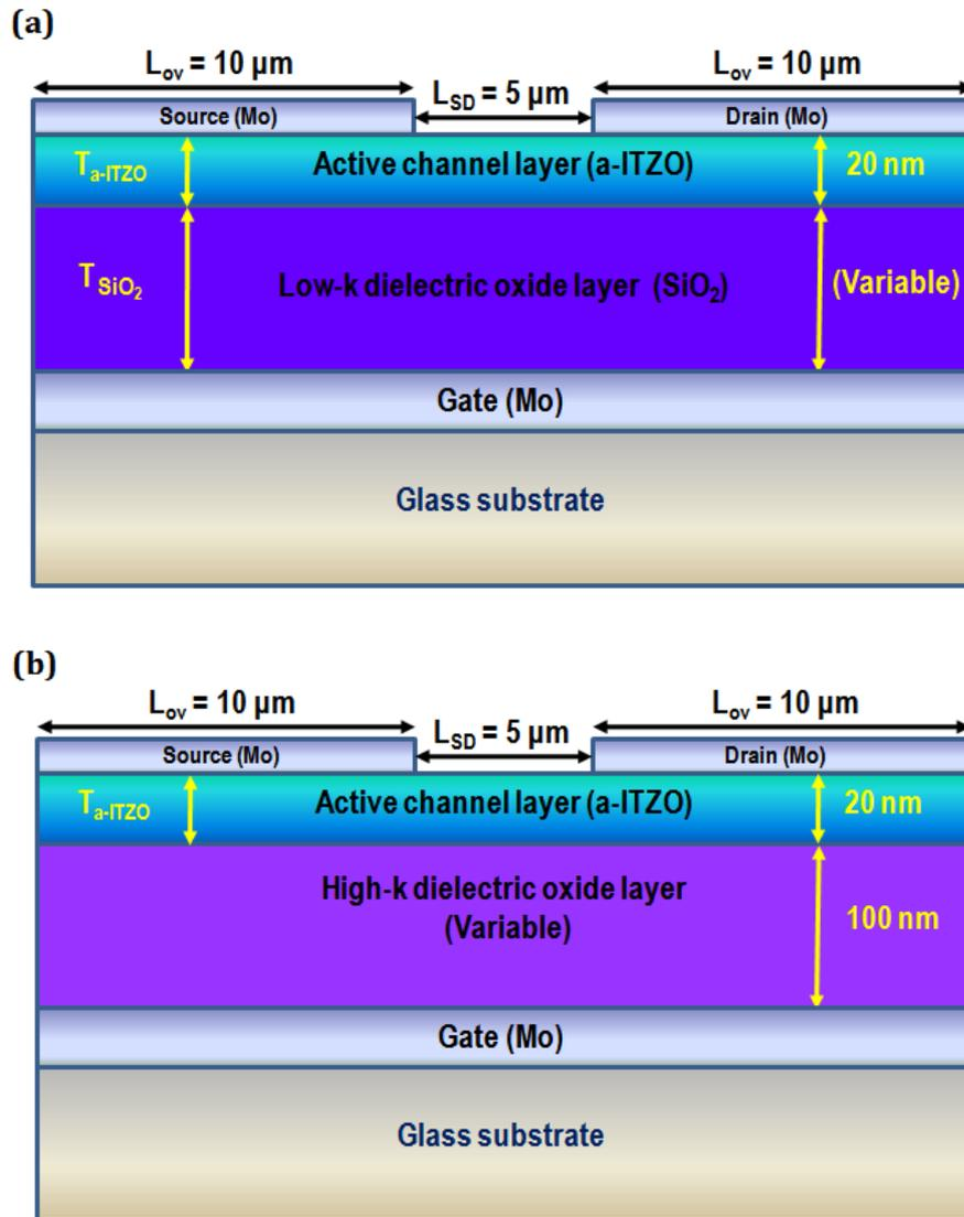
Figure III.4 Schematic diagram of a two-dimensional cross-section of the staggered bottom-gate a-ITZO TFT; dimensions, regions, and materials used in the simulation for (a) low-k  $\text{SiO}_2$  gate dielectric and (b) high-k gate dielectric.
