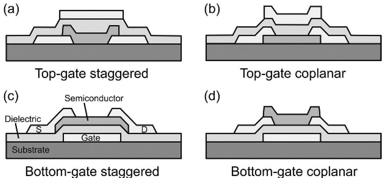
Figure I.5 The most typical TFT structures depending on the positioning of layers: (a) top-gate staggered, (b) top-gate coplanar, (c) bottom-gate staggered, (d) bottom-gate coplanar TFT configurations [39].
