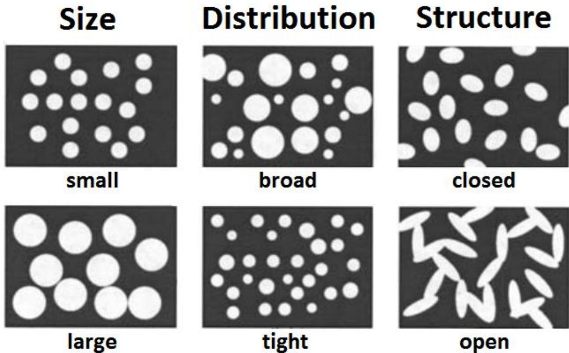
Figure I.7 Different sizes, distribution, and structure of pores inside a low-k porous dielectric material [66].
