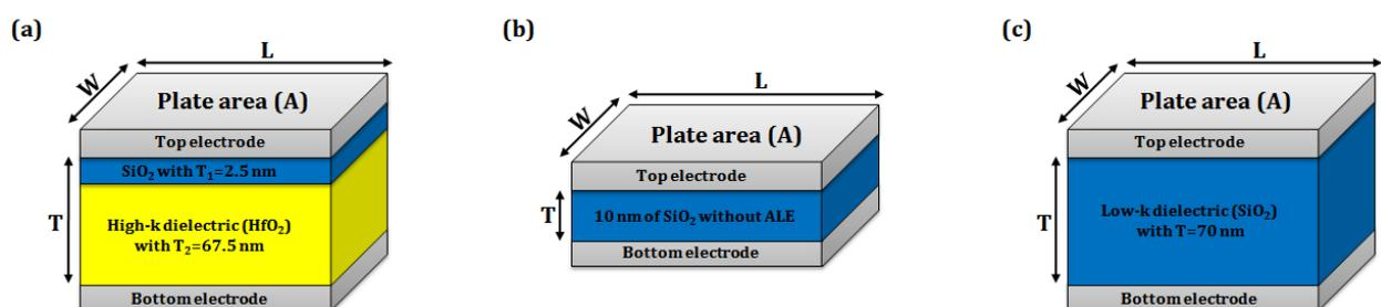
Figure III.9 Schematic diagram of the three-dimensional structure of a simple parallel plate capacitor depending on the different types of gate dielectrics: (a) 70 nm of a bi-layer dielectric oxide ( $\text{SiO}_2/\text{HfO}_2$ ), (b) 10 nm of  $\text{SiO}_2$  without associated leakage effect (ALE) and (c) 70 nm of  $\text{SiO}_2$ .
