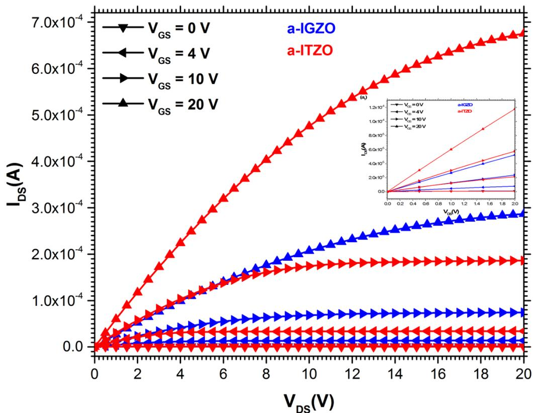
Figure III.3 The evolution of output ( $I_{DS} - V_{DS}$ ) characteristics of the a-IGZO and a-ITZO TFTs.
