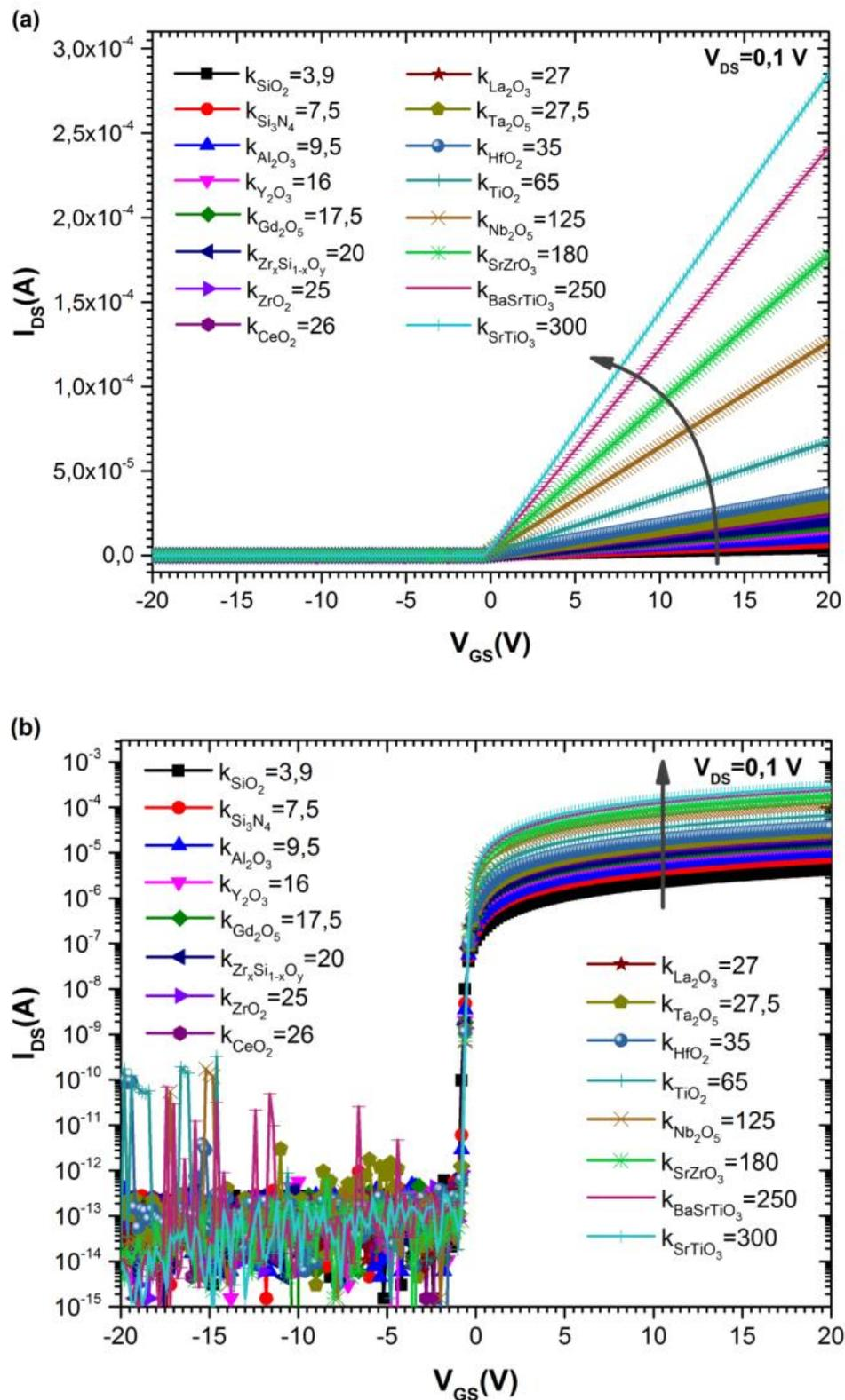
Figure III.8 The transfer ( $I_{DS} - V_{GS}$ ) characteristics of the a-ITZO TFT depending on the dielectric constant; (a) linear plot and (b) semi-logarithmic plot.
