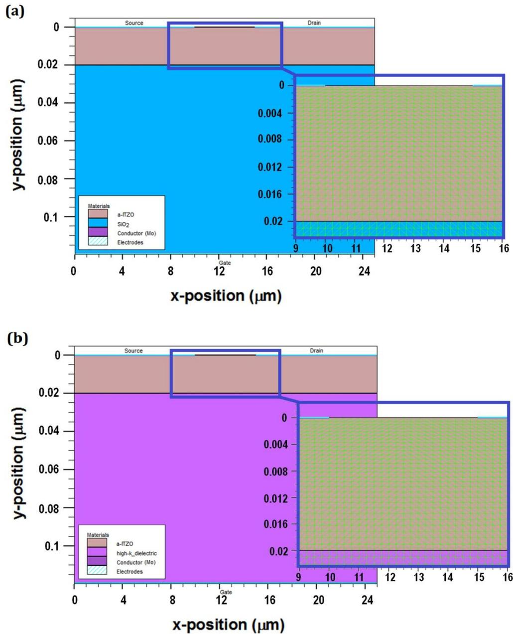
Figure III.5 The two-dimensional cross-section of the staggered bottom-gate a-ITZO TFT generated by Silvaco Atlas for (a) low-k SiO<sub>2</sub> gate dielectric and (b) high-k gate dielectric.
