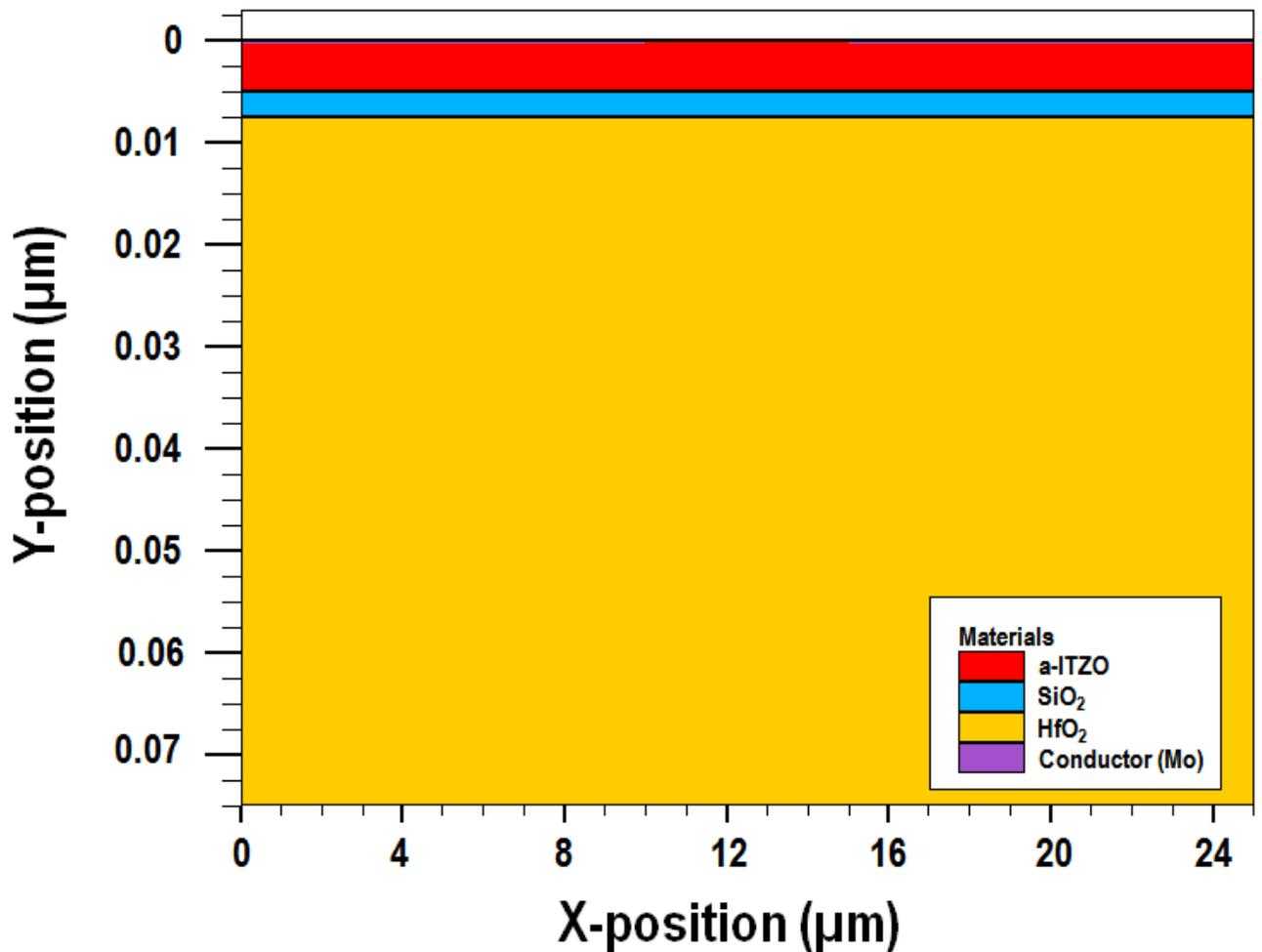
Figure II.3: Schematic diagram of a structure consisting of three regions generated by Silvaco Atlas.
