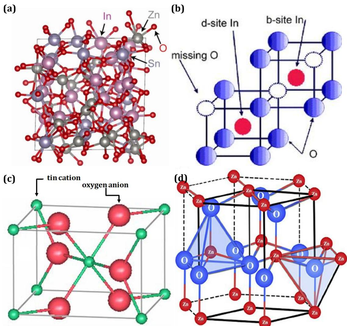
Figure I.2 Structures for each of a-ITZO,  $\text{In}_2\text{O}_3$ ,  $\text{SnO}_2$ , and ZnO, respectively, where (a) shows the amorphous structure of ITZO [20], (b) shows bixbyite-type cubic crystal structure of  $\text{In}_2\text{O}_3$ [21], (c) shows a rutile crystal structure of  $\text{SnO}_2$ [22], and (d) shows a wurtzite crystal structure of ZnO [23].
