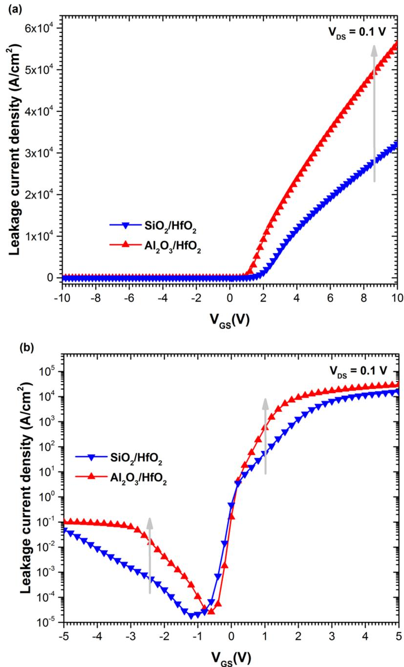
Figure III.22 The calculated of the leakage current density of the a-ITZO TFTs depending on the different types of the interfacial dielectrics: (a) the evolutions of the leakage current density in the linear plot while (b) the evolutions of the leakage current density in the semi-logarithmic plot.
