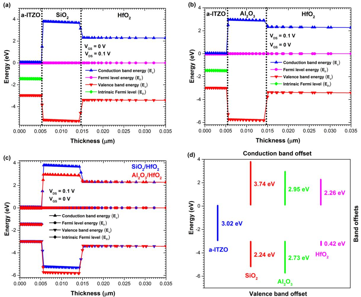
Figure III.21 The energy band diagram of the semiconductor/bi-layer dielectric oxide interface in a-ITZO TFTs and the different band offsets where (a) and (b) show the energy band diagrams of a-ITZO/SiO<sub>2</sub>/HfO<sub>2</sub> and a-ITZO/Al<sub>2</sub>O<sub>3</sub>/HfO<sub>2</sub> interfaces, respectively, and (c) shows comparative diagram of the energy bands while (d) shows the different band offsets in a-ITZO TFTs.
