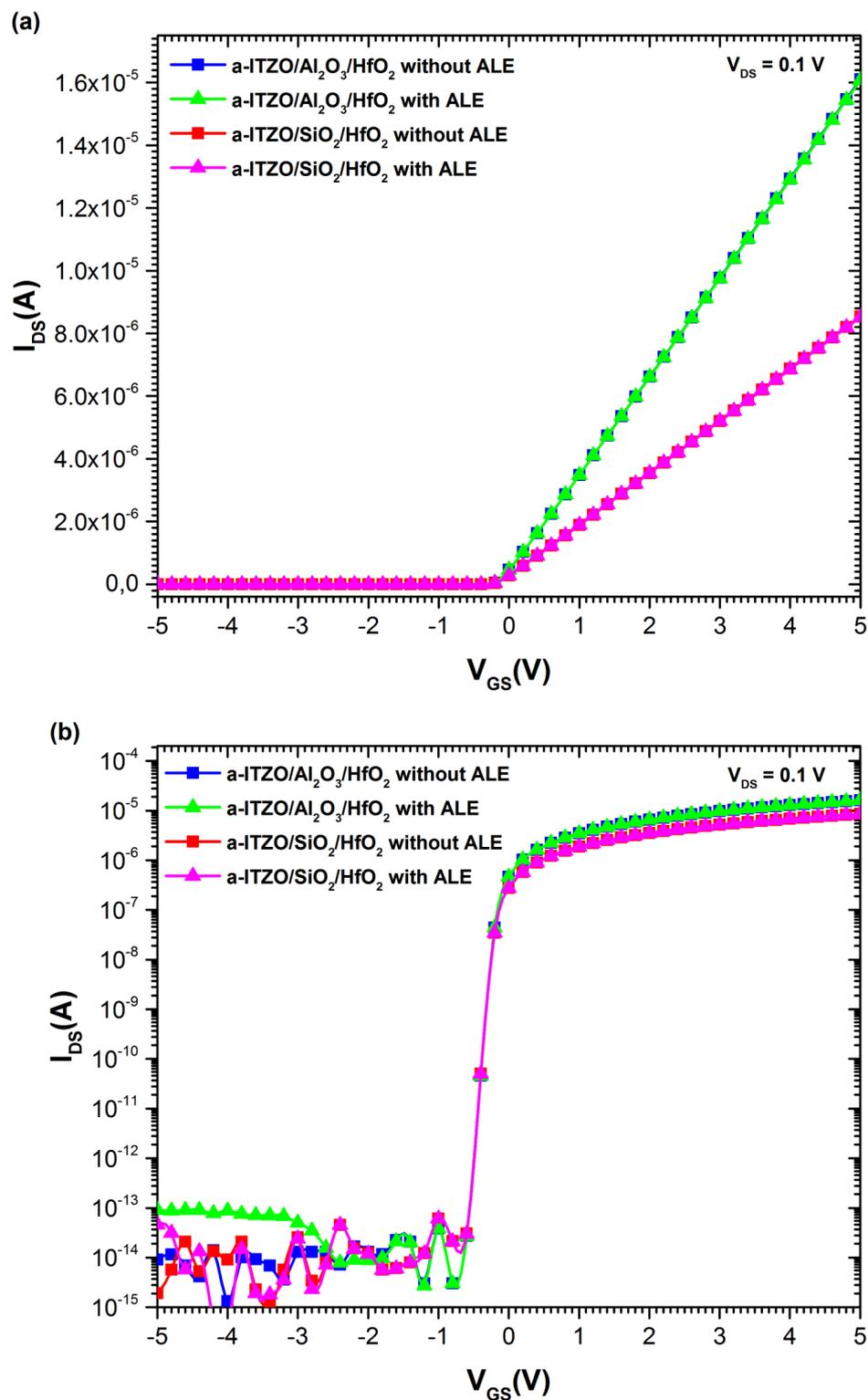
Figure III.24 The calculated of transfer ( $I_{DS} - V_{GS}$ ) characteristics of the a-ITZO TFTs with/without ALE depending on the different types of the interfacial dielectrics: (a) transfer characteristics in the linear plot and (b) transfer characteristics in the semi-logarithmic plot.
