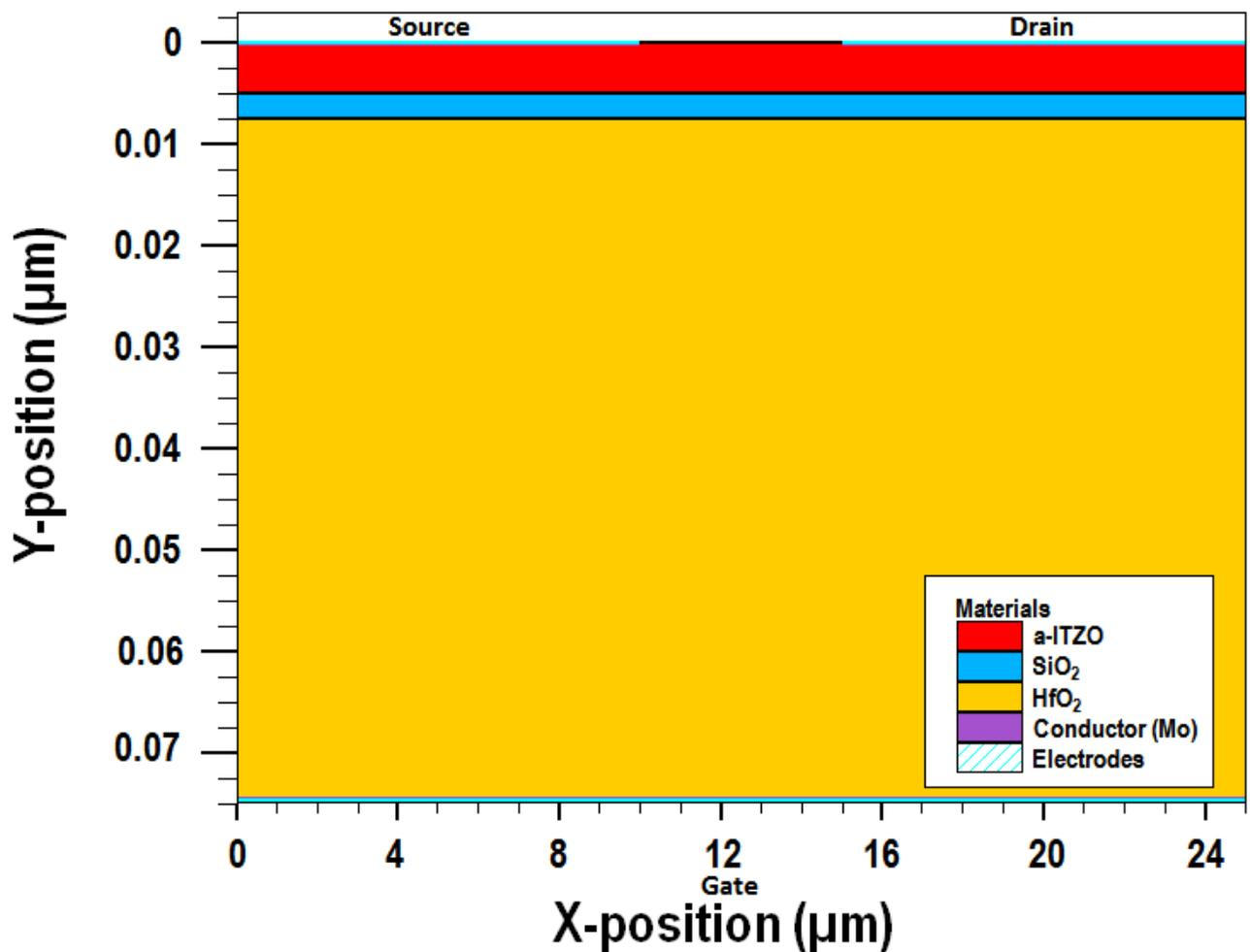
Figure II.4: Schematic diagram of a structure consisting of three regions with the source, drain and gate electrodes generated by Silvaco Atlas.
