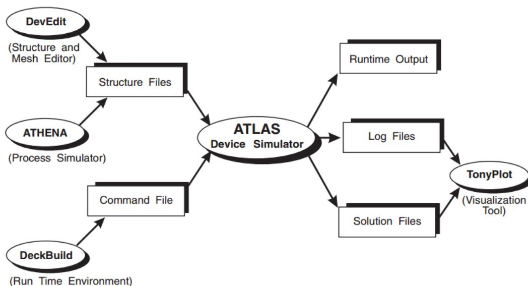
Figure II.1 Atlas inputs and outputs [1].
