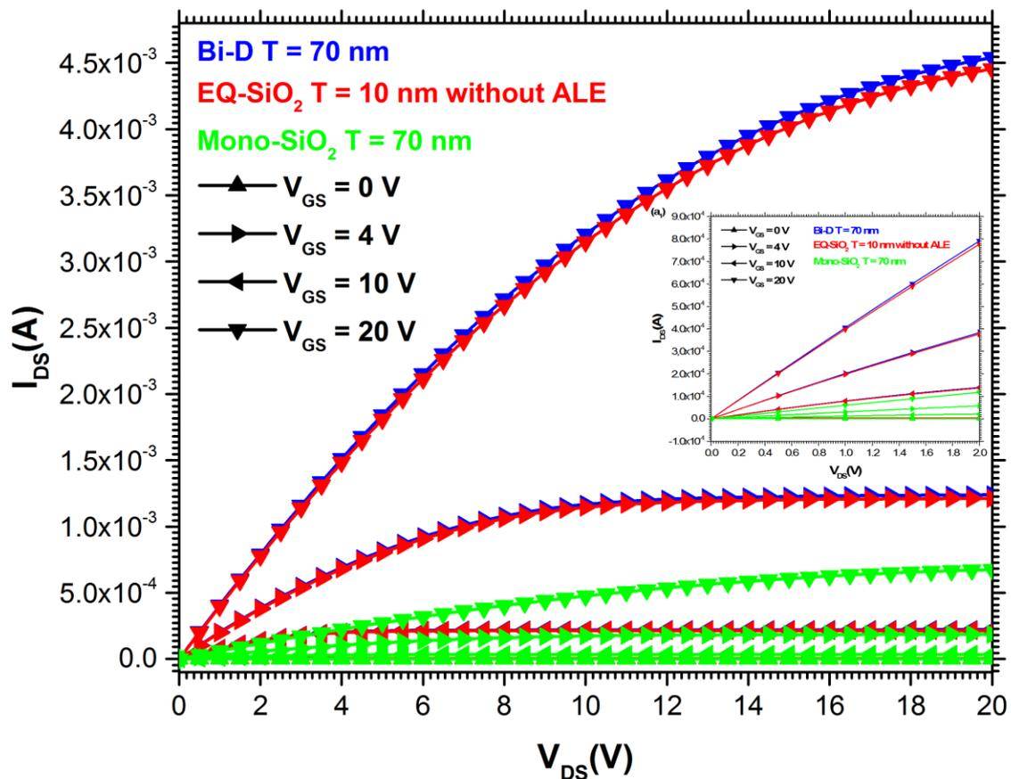
Figure III.15 The evolution of the  $I_{DS} - V_{DS}$  characteristics of the a-ITZO TFTs depending on the different types of the gate dielectrics: bi-layer dielectric thickness (Bi-D T), equivalent  $\text{SiO}_2$  thickness (EQ-  $\text{SiO}_2$  T) and monolayer  $\text{SiO}_2$  thickness (Mono- $\text{SiO}_2$  T).
