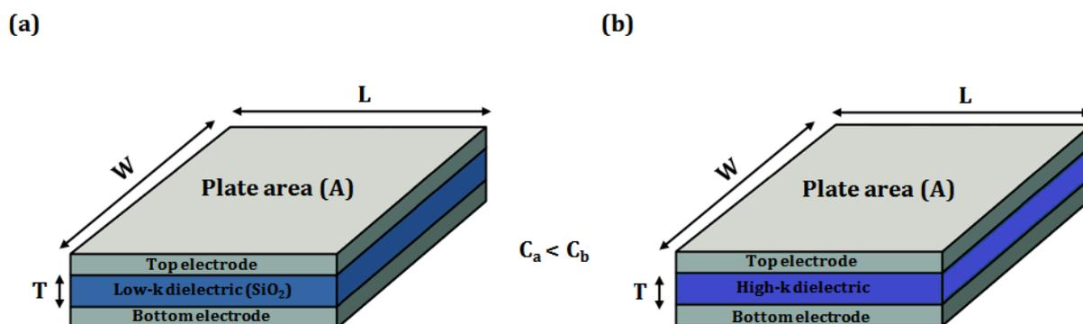
Figure I.8 Simplified representation of the three-dimensional structure of a simple parallel plate capacitor with (a) low-k dielectric and (b) high-k dielectric.
