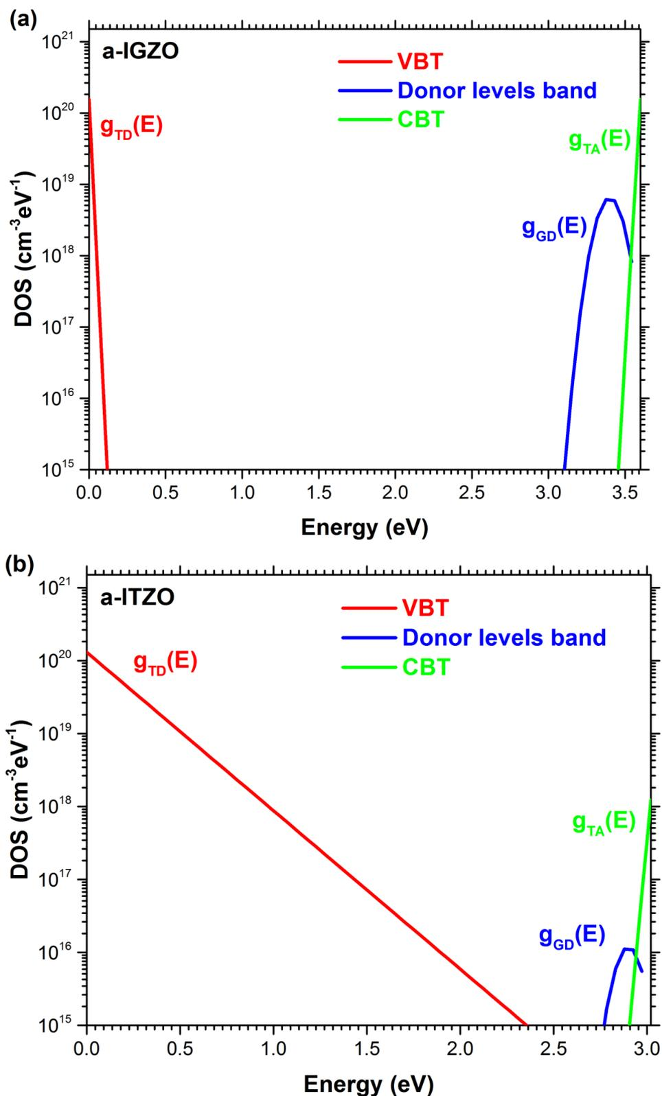
Figure II.5: Schematic of DOS models used in the simulation of the total subgap energy range of
