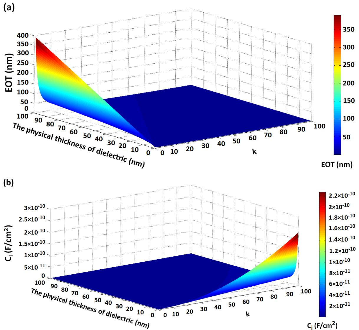
Figure III.14 The evolutions of (a) the EOT and (b)  $C_i$  depending on  $k$  and the physical thickness of the dielectric material.
