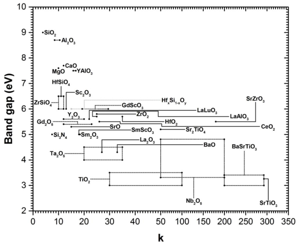
Figure III.7 Band gap energy as a function of the dielectric constant for different dielectric materials [17, 23-42].
