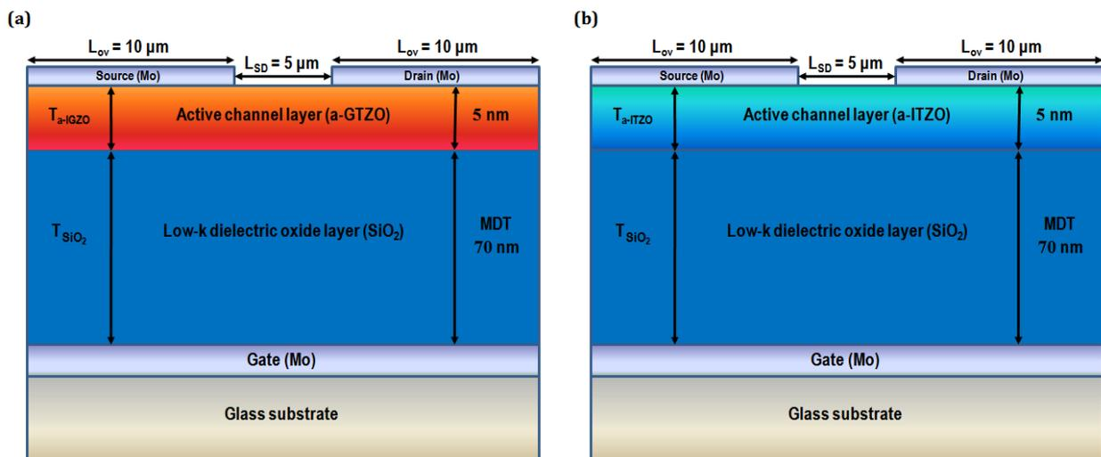
Figure III.1 Schematic diagram of a two-dimensional cross-section of the bottom-gate TFTs structure, dimensions, regions, and materials depending on the types of channel material: (a) a-IGZO and (b) a-ITZO.
