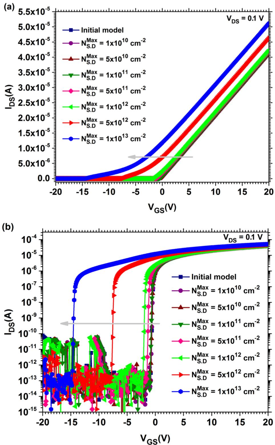
Figure III.18 Transfer characteristics of the a-ITZO TFT with bi-layer  $\text{SiO}_2/\text{HfO}_2$  gate dielectrics: (a) linear plot and (b) semi-logarithmic plot, for different densities of the a-ITZO/ $\text{SiO}_2$  interface states.
