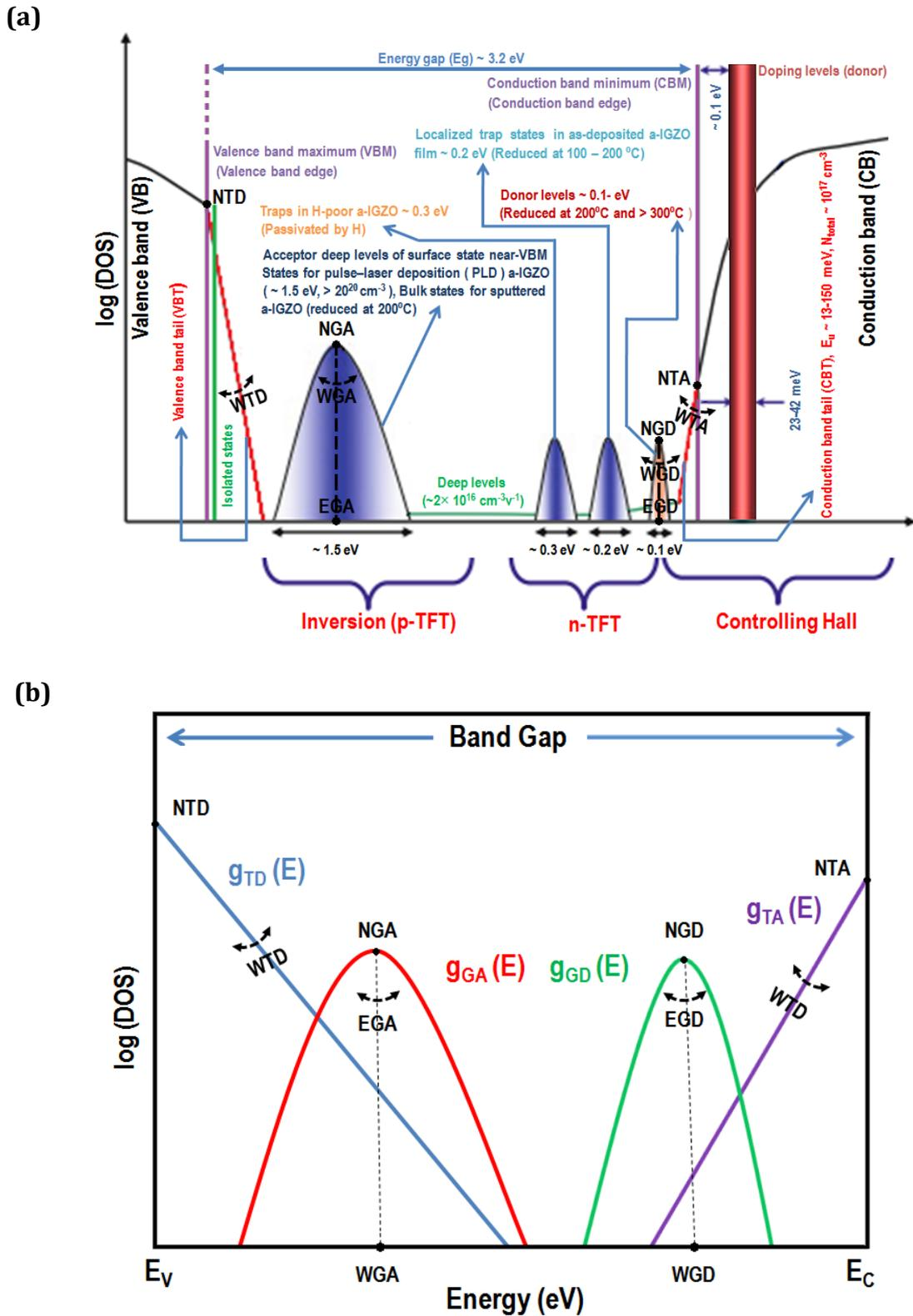
Figure I.1 Schematic electronic structure of a-IGZO where (a) shows the total density of states (DOS) within the band gap of as-deposited a-IGZO [10-13], while (b) shows the density of states (DOS) within the subgap of disordered materials after annealing ( $g(E)$ )[14].
