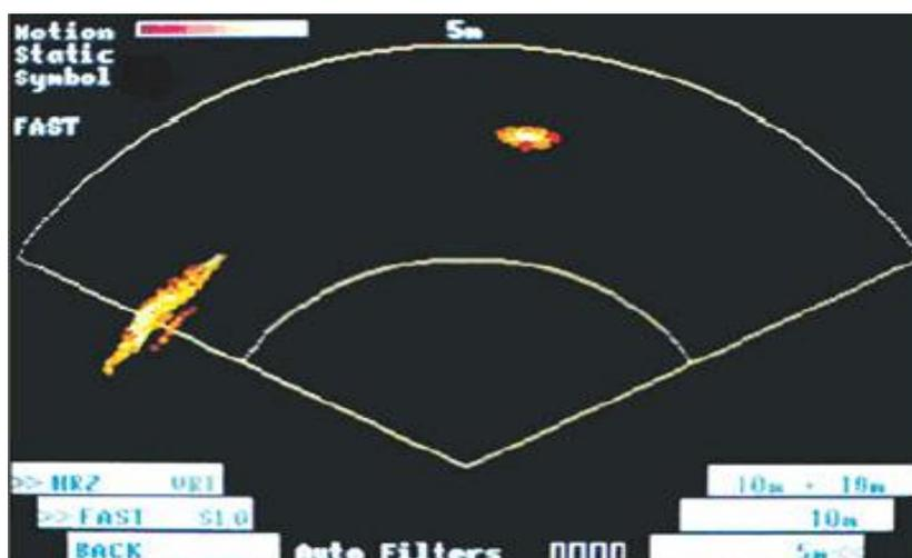
Fig I.7.b Example of GPR that detects two targets at a distance of 5m [11]
