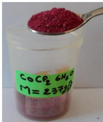
**Figure 3.22:** Cobalt (II) chloride hexahydrate.
