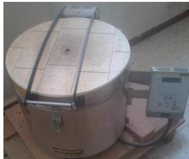
Figure 3.15: The annealing oven.
