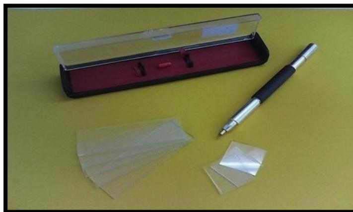
**Figure II.2:** Cut glass substrates using a sharp pen
