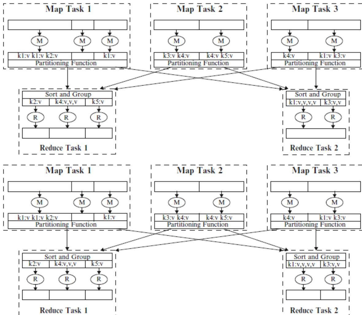
**Figure II.6:** Distributed Processing using Map Reduce.
