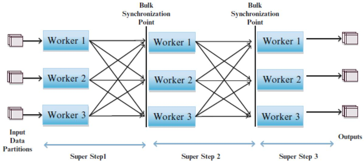
**Figure II.5:** Distributed Processing using the Bulk Synchronous Parallel.
