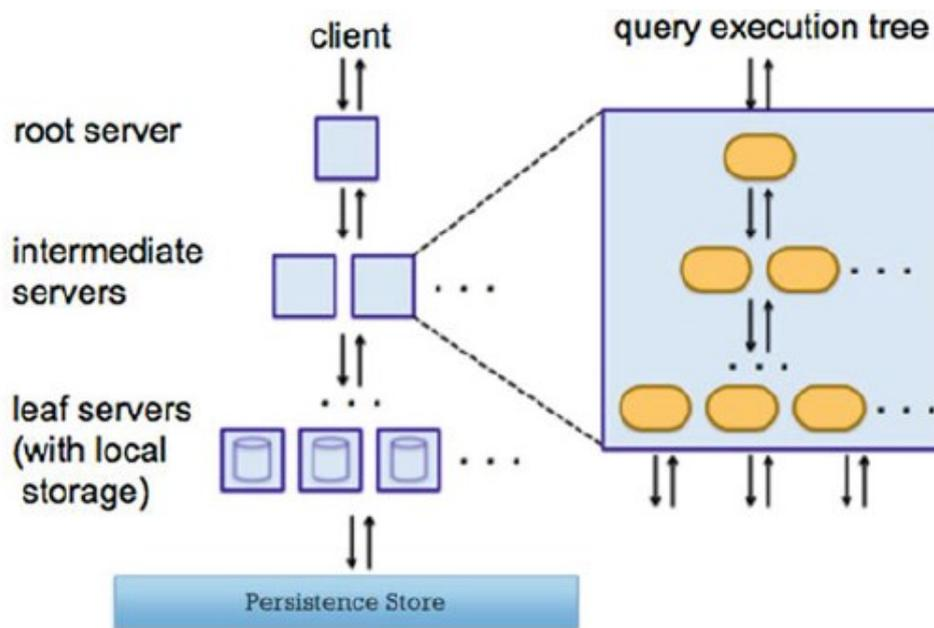
**Figure II.4:** Distributed Processing using Multi-Level Serving Tree (Reproduced from).
