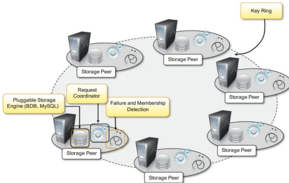
**Figure II.9:** The architecture of Amazon Dynamo.
