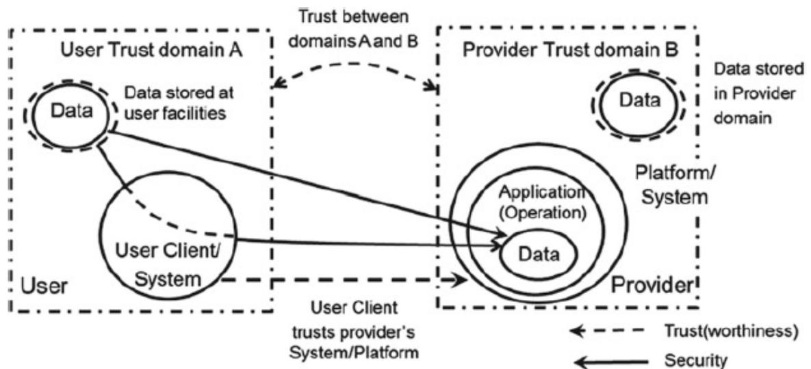
Figure .III.2. Security and Trust in Data Services and Infrastructure.
