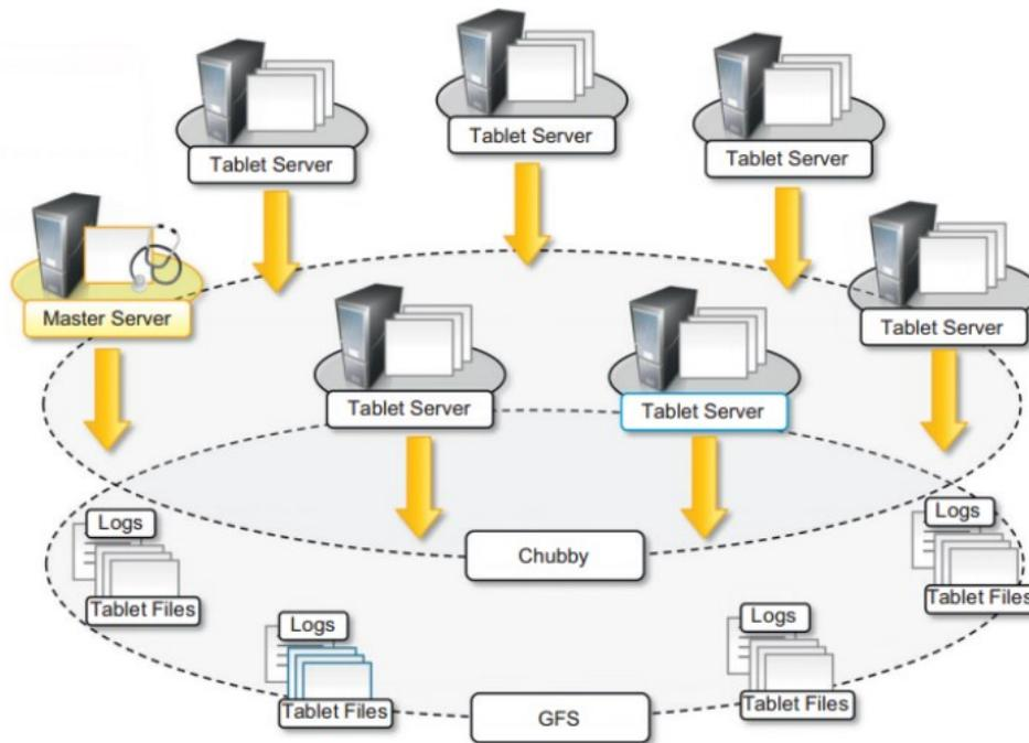
*Figure II.10:* The architecture of the Bigtable.
