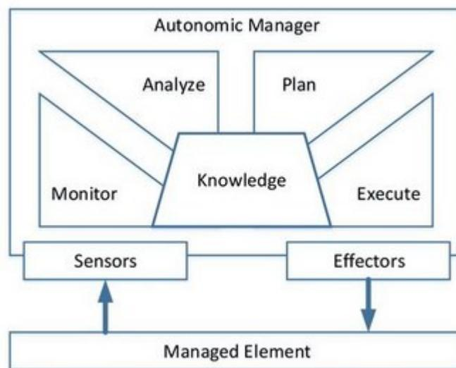
**Figure V.1:** Autonomic System MAPE-k [65].
