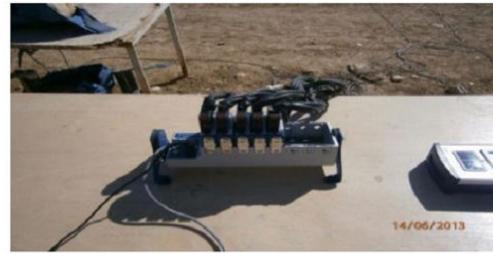
Figure 4. DAQ-9188 acquisition card (National Instruments)
