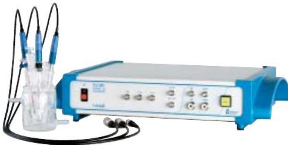
**Figure II. 16:** The VOLTALAB PGZ-301 potentiostat.
