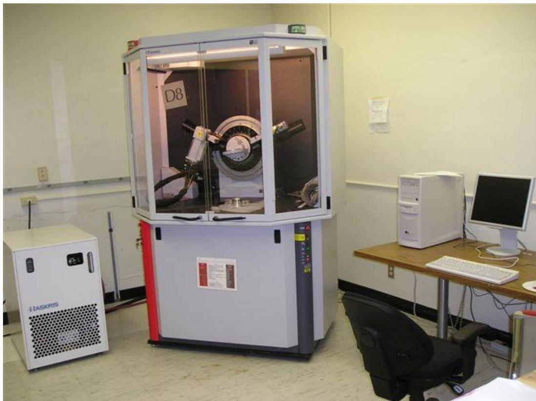
**Figure II.8:** Bruker D8- Advanced diffractometer.
