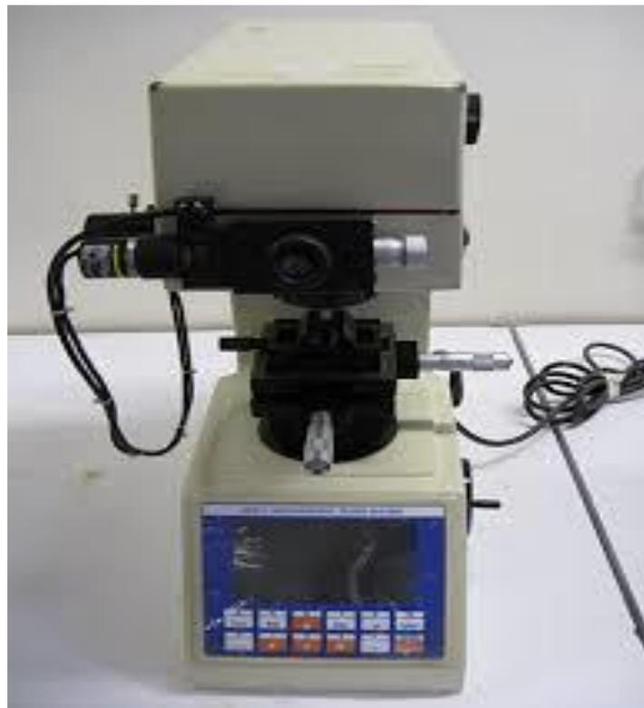
**Figure II.6:** Microhardness apparatus.
