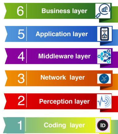
Figure 2.5: IoT-Architecture Based on Formation Model.
