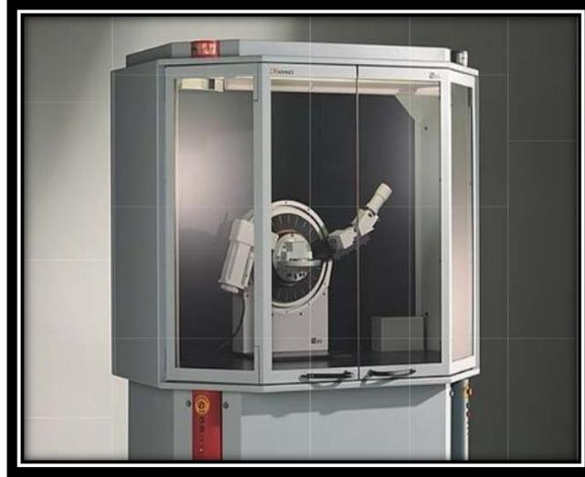
**Figure (II-3):** Bruker D8 Advanced X-ray Diffractometer[6].
