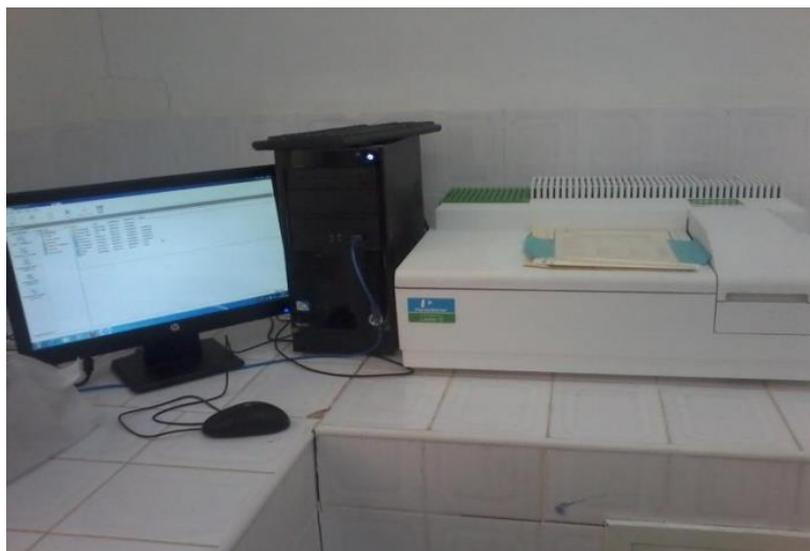
*Figure (II-6):Ultraviolet-visible spectrophotometer (LAMBDA 25)*
