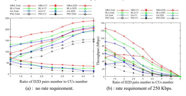
Figure 4.6. Effect of the ratio of D2D to the CU, average results on 50 runs.
