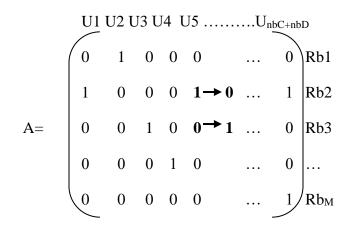
Figure 3.3. Food foraging: For example, if U5 is the picked D2D communication, we swap from Rb2 to Rb3 and improve its transmission power.
