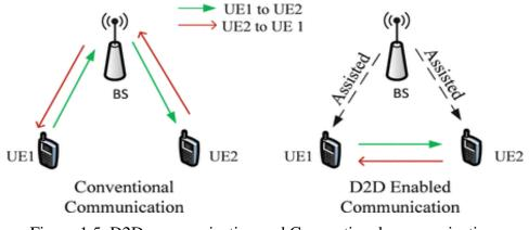
Figure 1.5. D2D communication and Conventional communication.
