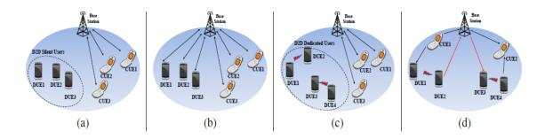
Figure 1.11. Modes of communication in D2D networks (a) Pure cellular mode (b) Partial cellular mode (c) Dedicated mode (d) Underlay mode.
