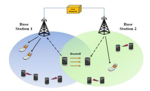
Figure 1.12. Typical handover scenario in D2D Communication.
