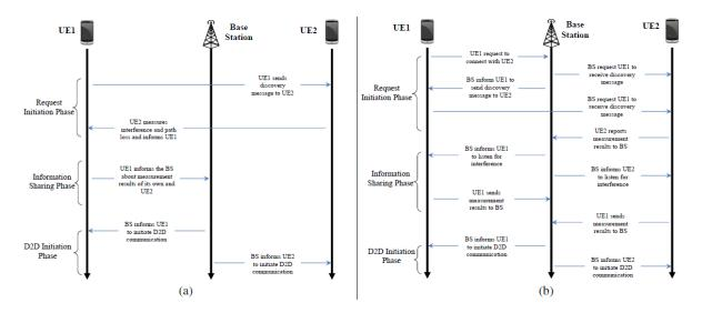
Figure 1.10. Centralized device discovery (a) Partial involvement of BS, (b) Complete involvement of BS.
