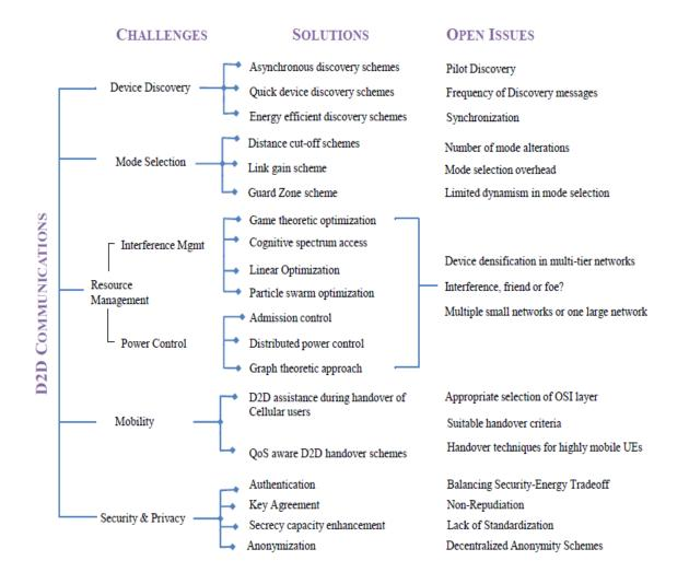
Figure 1.9. Challenges of D2D Communication, Solution and Open Issues.
