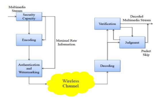
Figure 1.13. Combined Physical-Application Layer Security Scheme
