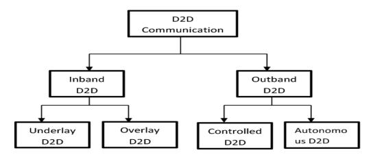
Figure 1.6. Classification of D2D communication.
