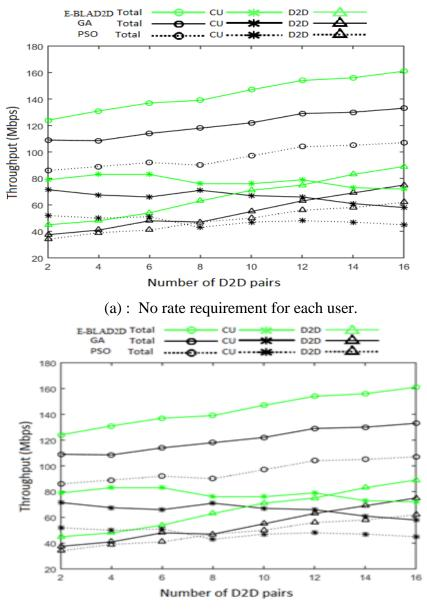
(b) : Rate requirement for one user is 250 Kbps. Figure 3.13. Vary D2D pairs number for E-BLAD2D, PSO and GA.
