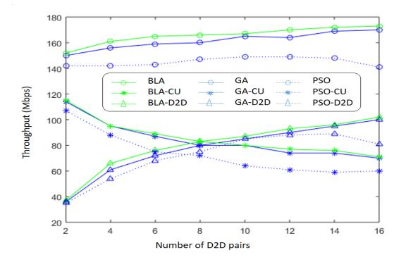
Figure 3.5. Impact of increasing D2D pairs on network throughput.
