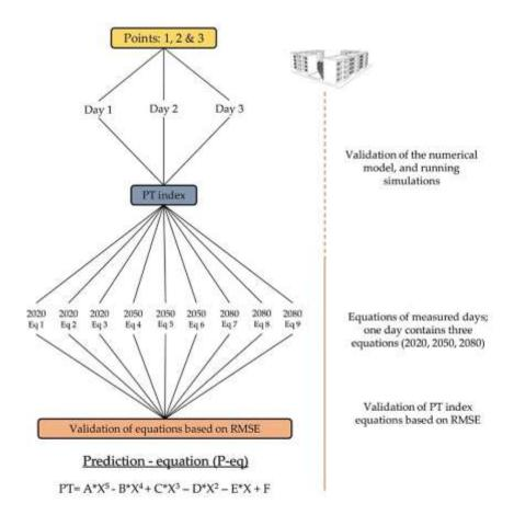
Figure 6.5: Workflow steps of the PT thermal index predictions algorithm
