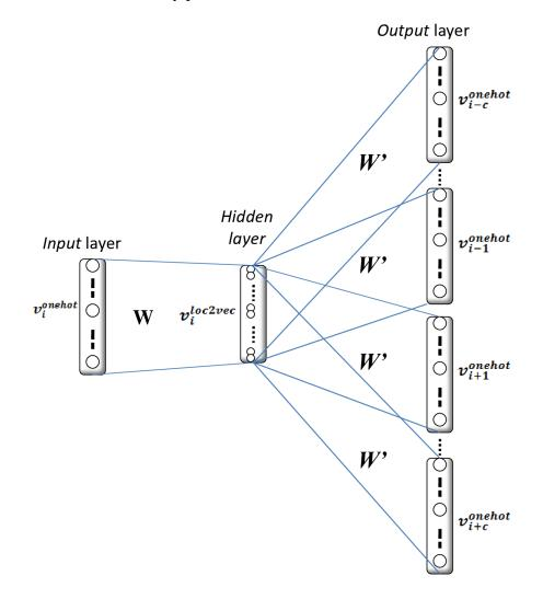
Fig. 3.2 Architecture of the training loc2vec neural network.
