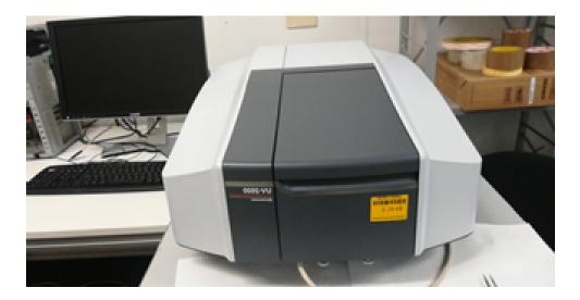
Figure 4.10: UV-VIS -characterization technique.
