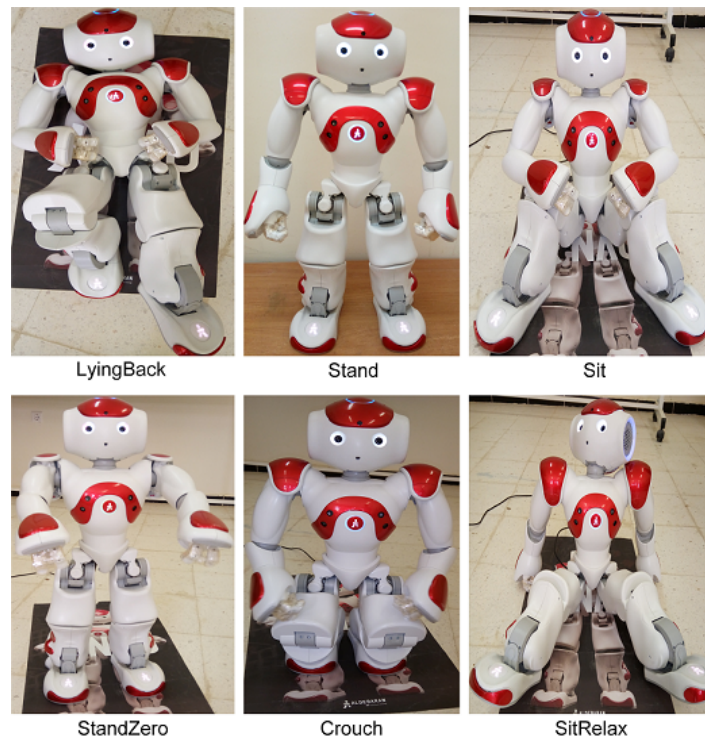
Figure 5.8: Some NAO's postures execution when invoking the Web service.
