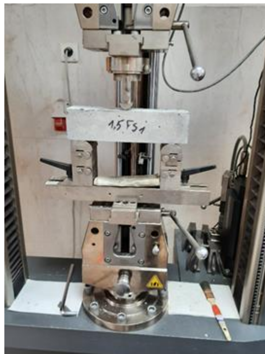
Figure II-11 Essai de flexion 3 points
