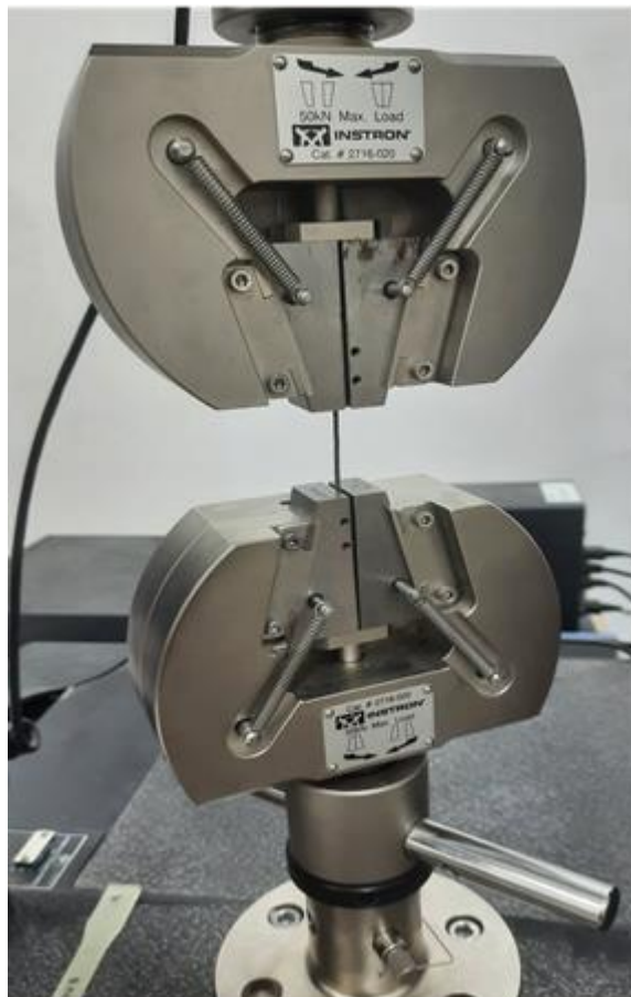
Figure 0-4 Test de traction directe.
