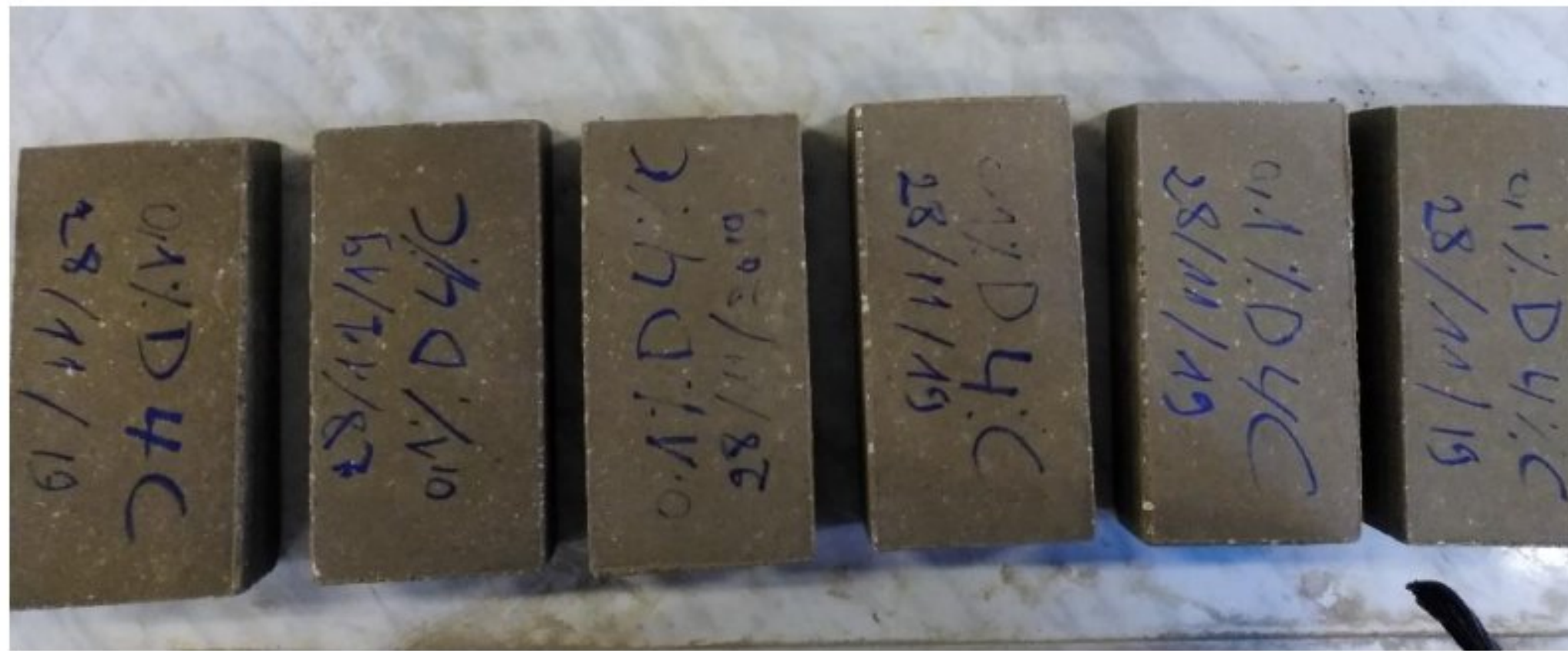
Fig.3. 11. Compressed Earth Bricks (CEBs) manufactured in this study.
