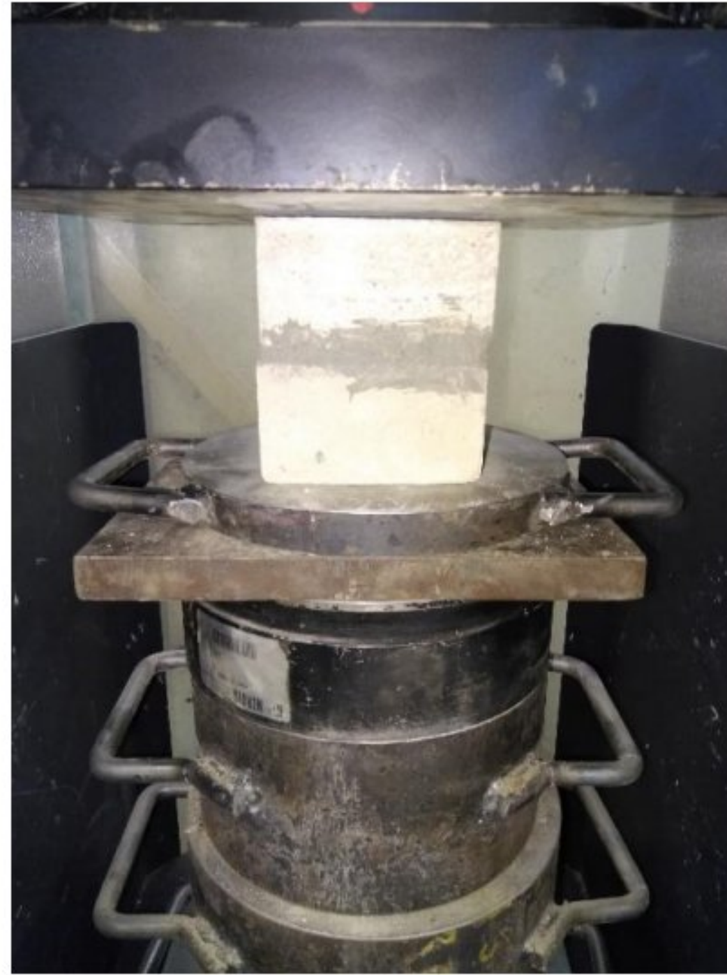
Fig.3. 12. Experimental setup of compressive strength test.
