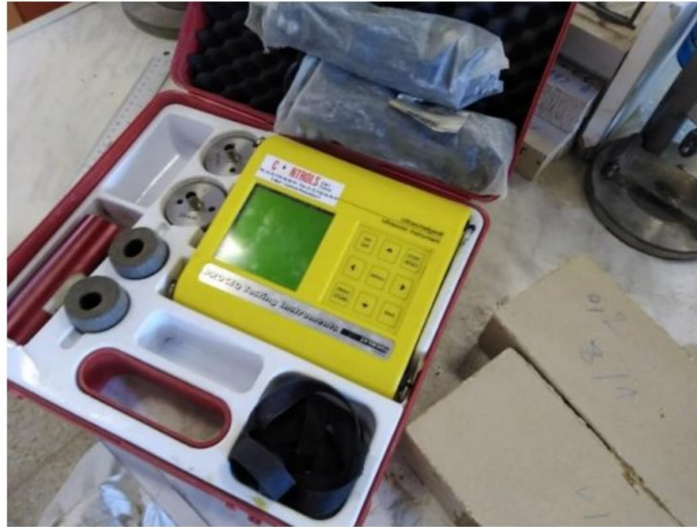
Fig.3. 15. Ultrasonic pulse velocity test (non-destructive test) of CEBs blocks.
