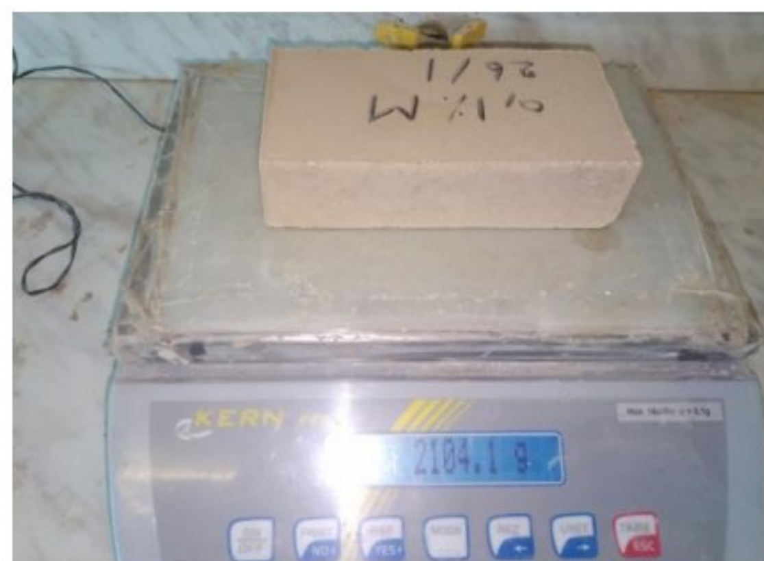
Fig.3. 17. Measuring the weight of block for density.
