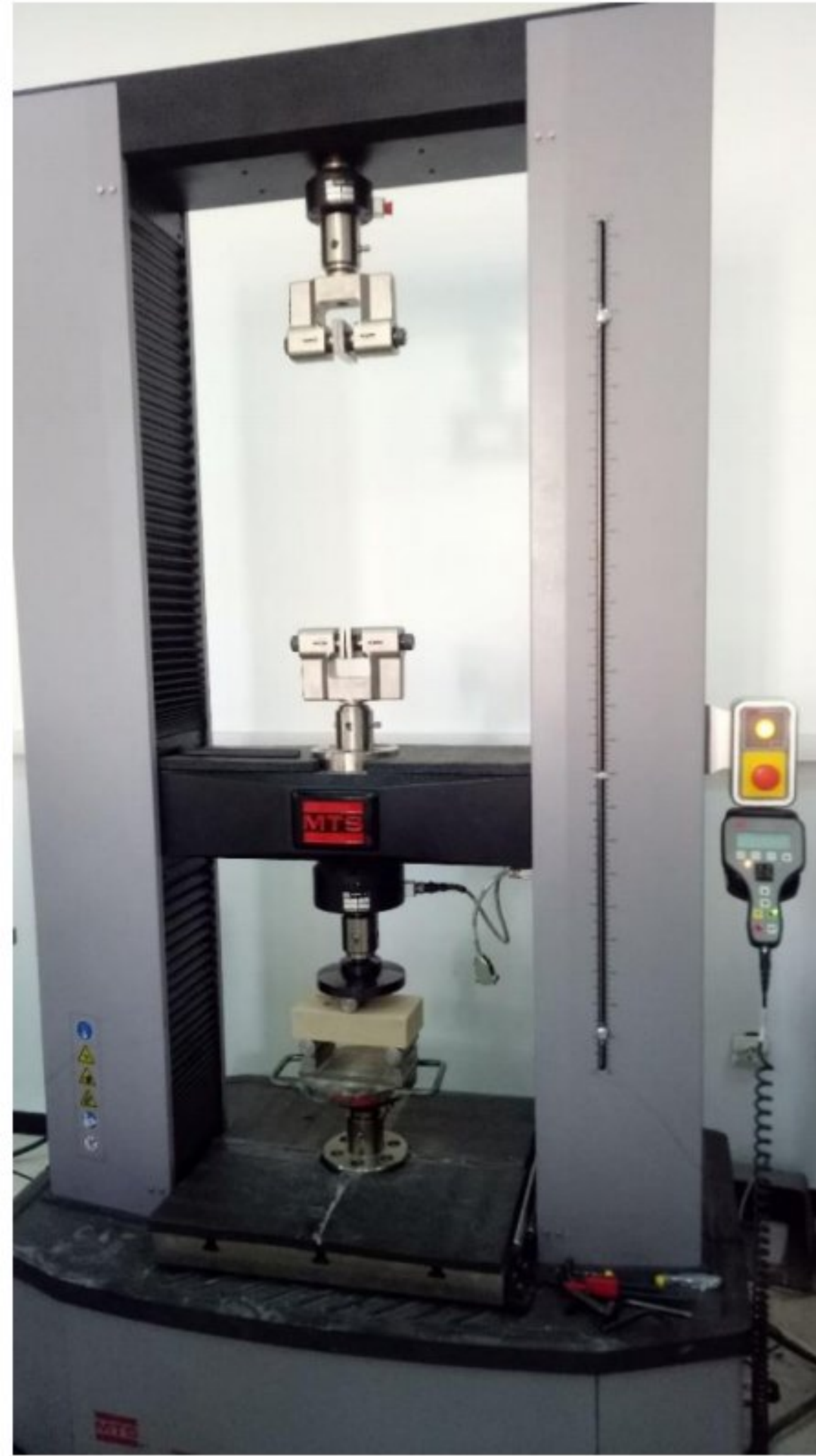
Fig.3. 13. Experimental setup of three-point bending.
