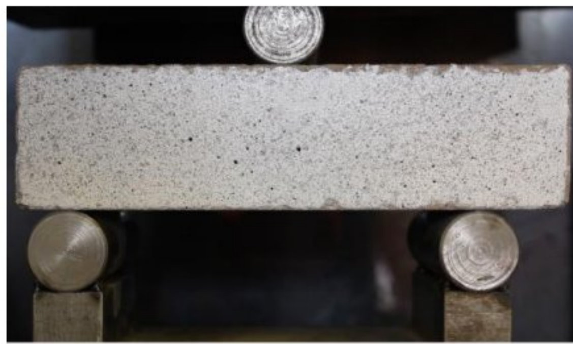
Fig.3. 18. Sample ready for DIC test.
