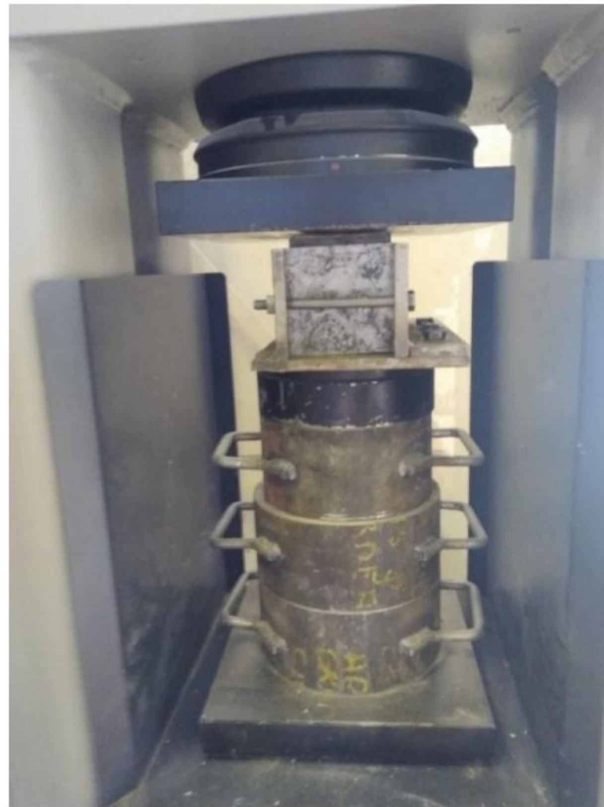
Fig.3. 8. Static compaction for manufacturing of CEBs.
