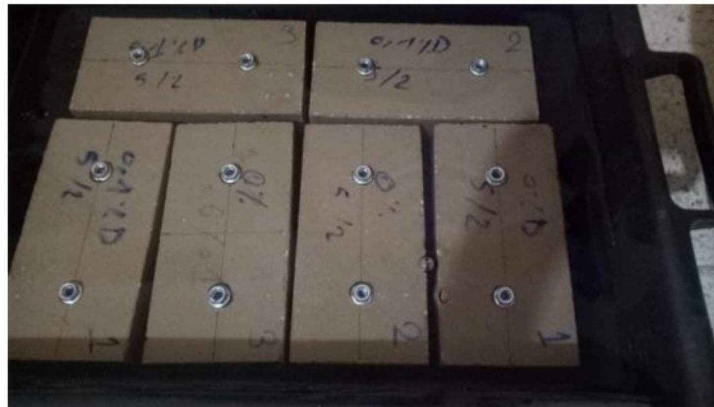
Fig.3. 16. Total water absorption and swelling test.
