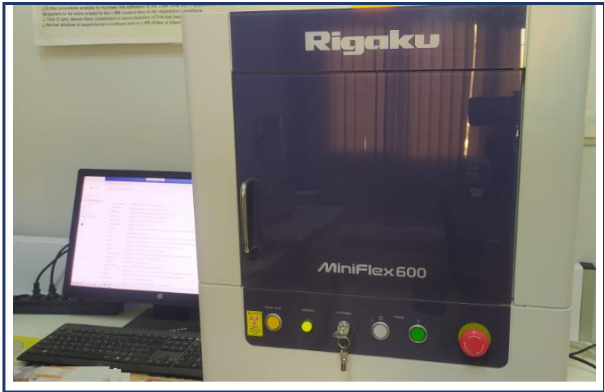
Figure 3. Rigaku-Type MiniFlex600 X-ray diffractometer.
