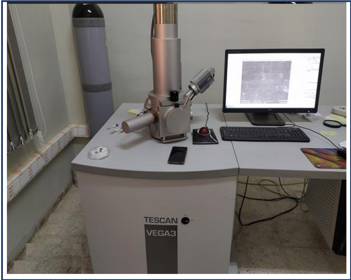
Figure 7. Scanning electron microscope “TESCAN-VEGA3”.
