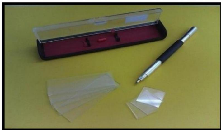
Figure II.4: Cut glass substrates using a sharp pen.
