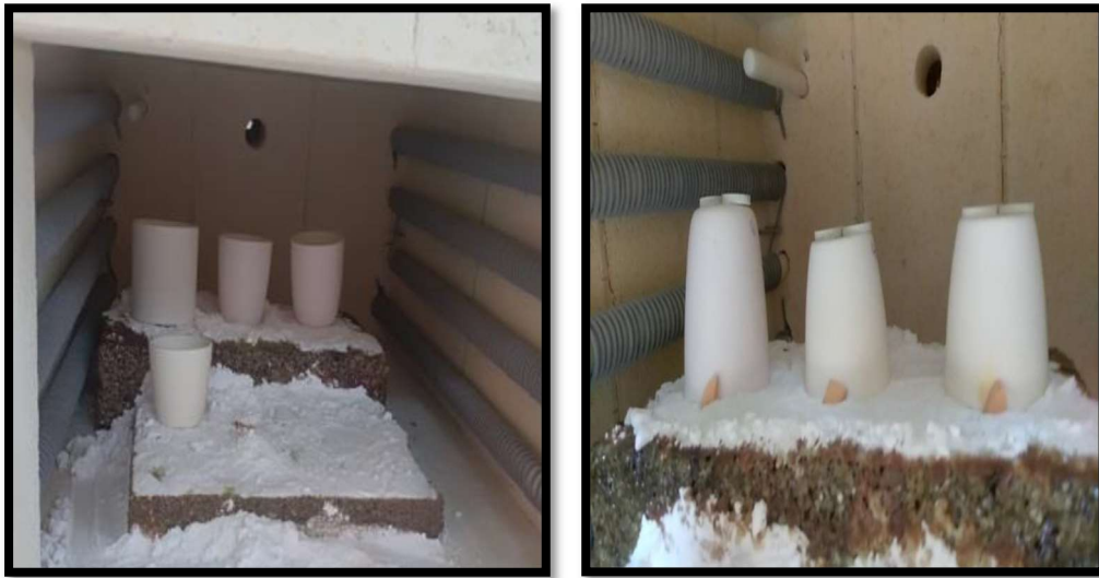
Figure II. 4: The position of the pellets during sintering.
