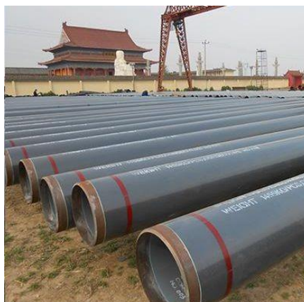
Figure I.7 Pipeline en acier X70 [20].
