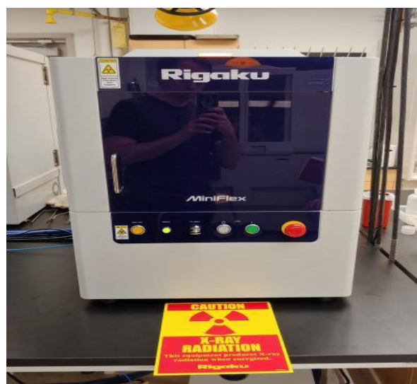
Fig. II. 5. Mini-Flex (Rigaku) diffractometer.
