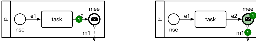
Figure 4.14: Starting Behaviour of a Message End Event. Before (left) and after (right) application of the St rule.
