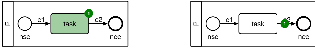
Figure 4.16: Completing Behaviour of an Abstract Task Activity. Before (left) and after (right) application of the Ct rule.
