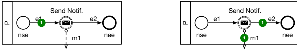
Figure 4.22: Starting Behaviour of a Throw Message Intermediate Event. Before (left) and after (right) application of the St rule.
