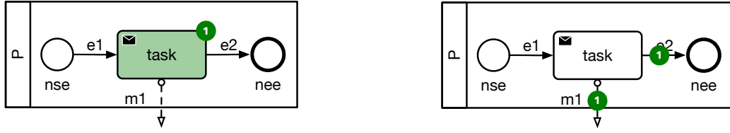
Figure 4.20: Completing Behaviour of a Send Task Activity. Before (left) and after (right) application of the Ct rule.
