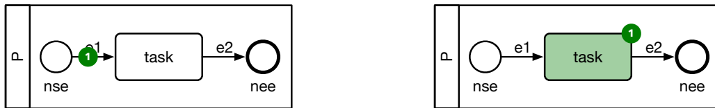
Figure 4.15: Starting Behaviour of an Abstract Task activity. Before (left) and after (right) application of the St rule.
