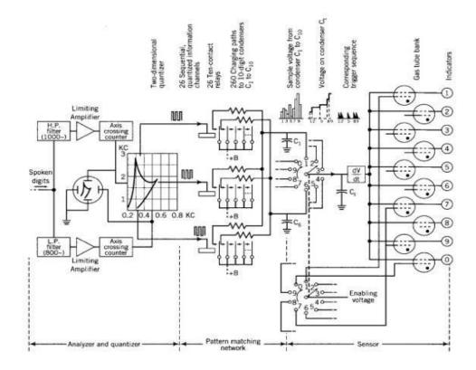
Figure 8 is a schematic for Bell Lab's digit recognizer that demonstrates how speech is produced. Three distinct sequential processes are involved in the recognition stage. First, speech is analyzed to create a formant one vs. formant two. Then, a pattern-matching network determines which pattern in 10 reference distributions most closely resembles an unknown signal distribution. Finally, this information is displayed visually by an indicator of the necessary associated circuits.
