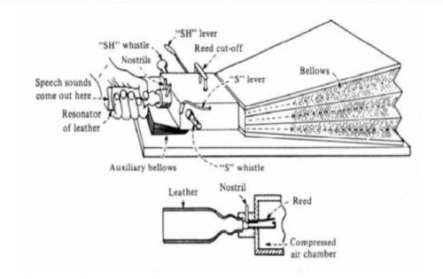
The device shown in Figure 5 is operated by resting the arm in the prominent bellows and blowing the air through a vibrating reed to produce voiced sounds, and the right-hand fingers control the air passages. Vowel sounds require the closure of all air passages and the activation of the reed, while unvoiced sounds are produced with the reed off and a turbulent flow through the passage (Flanagan, 1972).
