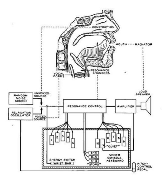
Figure 6 is a schematic of the voder that shows the electrical circuit for producing speech with manual controls.
