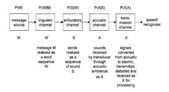
The decision to transmit an intended message M - realized as a word sequence W via a linguistic channel is made by a message source and is determined by a probability measure P. A message source decides to convey an intended message M, realized as a word sequence W through a linguistic channel, specified by a probability measure P. The sound sequence S is then released from the speaker's mouth and travels around the space as acoustic waves (Juang and Furui, 2000).
