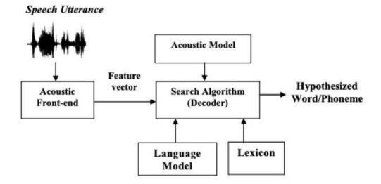
The automatic speech recognition system collects several speech parameters from the acoustic speech signal for each word or sub-word unit. The speech parameters create a pattern that identifies the word or sub-word. The operator then will read all the vocabulary words throughout the training phase, and when a word is recognized, its pattern is compared to the stored patterns (Karpagavalli and Chandra, 2016).
