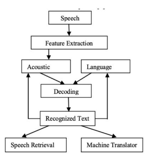
The process of turning speech into a text message is depicted in the above figure. The qualities that distinguish phonemes from one another are first separated from the speech signals. After that, the probabilities for various phonemes at various time instants are provided by the acoustic modeling. The type of phonemes and sequences that can be used in the target language are determined by language modeling. Finally, the acoustic and language models search for the
