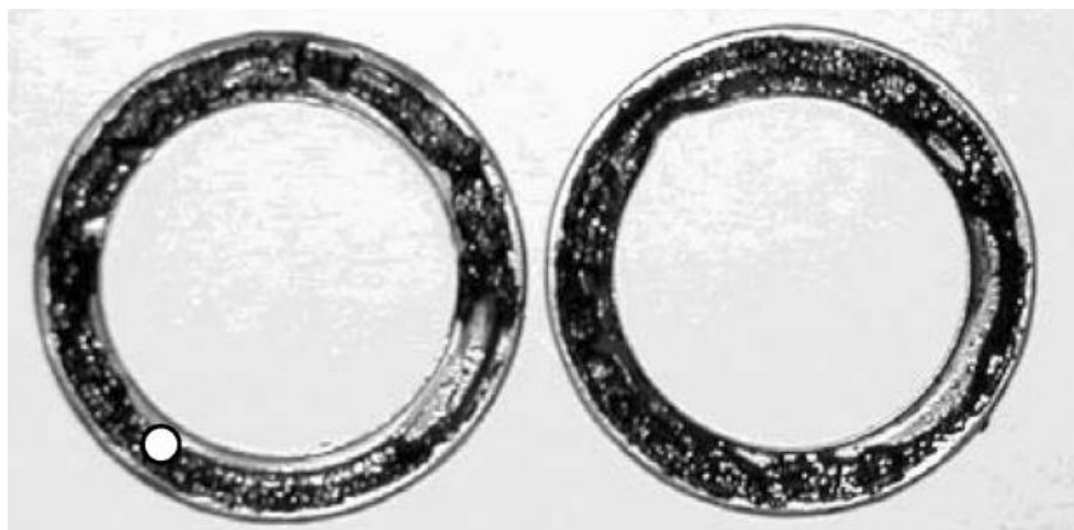
Fig. I.12: Degradation caused by the deterioration of the lubricant [CAN 07].
