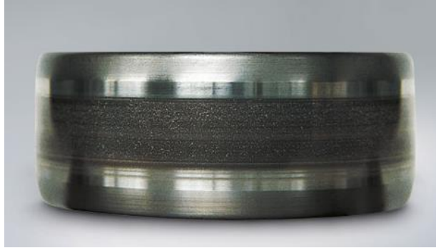
Fig. I.13: Effect on bearing of the flow of electric current [TRA 09]
