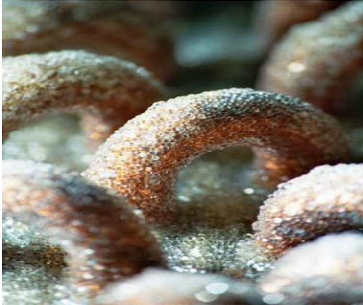
**Figure II-7** Photo of a silica gel coated tube and fin adsorbed heat exchanger [57].
