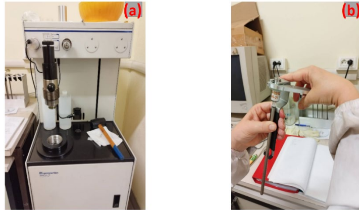
Figure III. 18. (a) The Micromeritics AutoPore IV 9500 series; (b) penetrometer closure
