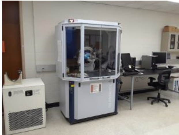
Figure III. 15. Bruker D8 X-ray diffractometer.
