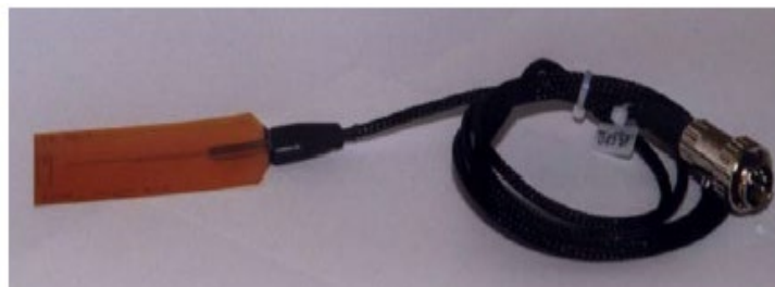
Figure III. 22. The single-rod probe or wire probe.
