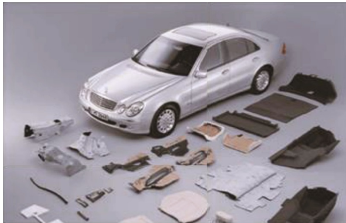
Figure I. 12. Components of automobiles made of natural fiber composites. [55]
