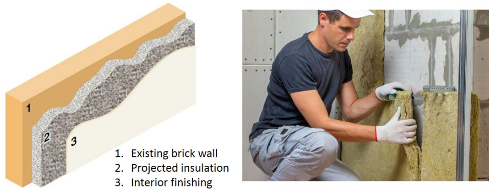
Figure I. 24. Diagram of internal isolation of a wall.
