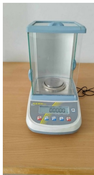
Figure III. 19. The Kern analytical balance ALS-A / ALJ-A
