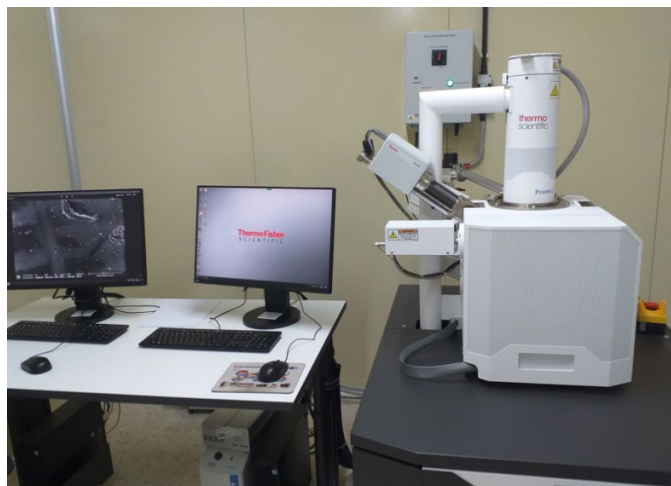
Figure III. 16. Thermo Scientific Prisma E Scanning Electron Microscope (SEM).
