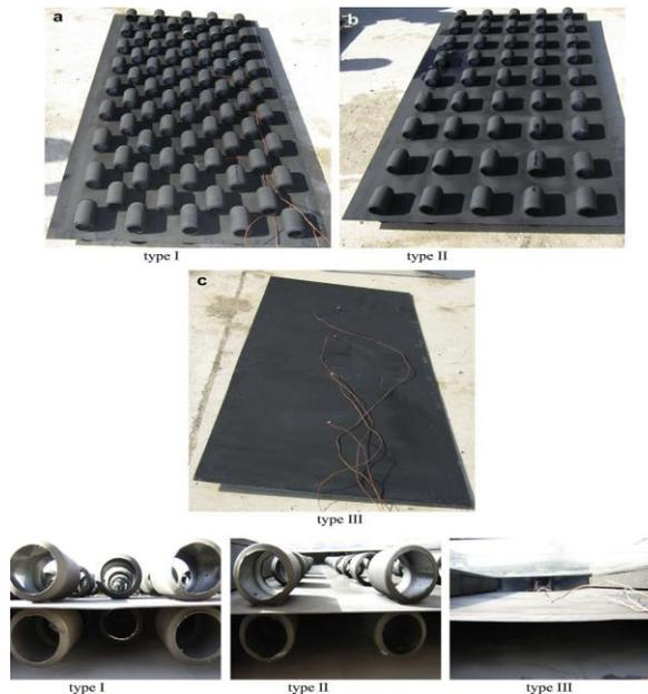
Figure I.17 Types and the view of absorber plates in the collector box, (a) type I, (b) type II, (c) type III [28].
