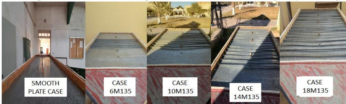
**Figure II.10** Different cases of the position baffles  $\beta = 135^\circ$ .
