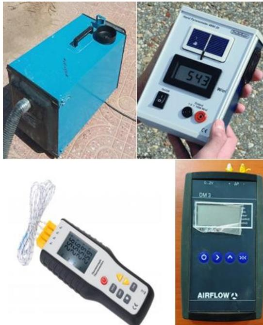
**Figure II.8** Used devices, Thermocouple, Aspirator Pyranometer, and airflow pressure device.
