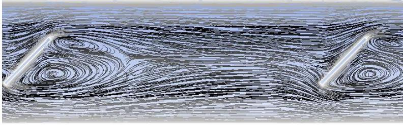
**Figure IV.24** Velocity path lines between two baffles (18 baffles case at  $Re=9515$ ).
