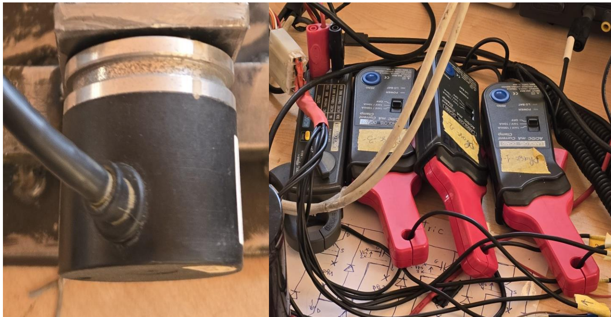
Figure V.5. The optical encoders from LIKA and Current sensors specifically the LANGLOIS DCA60 model.
