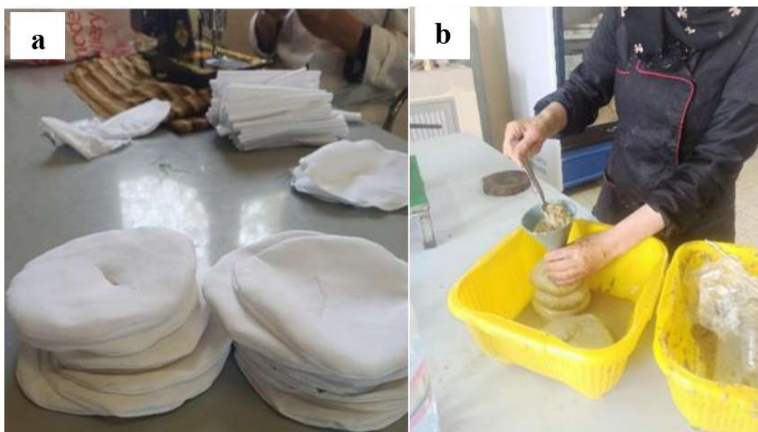
a ; Scourtins preparation, b ; Placing of the olive paste in the scourtin ( Original ).
