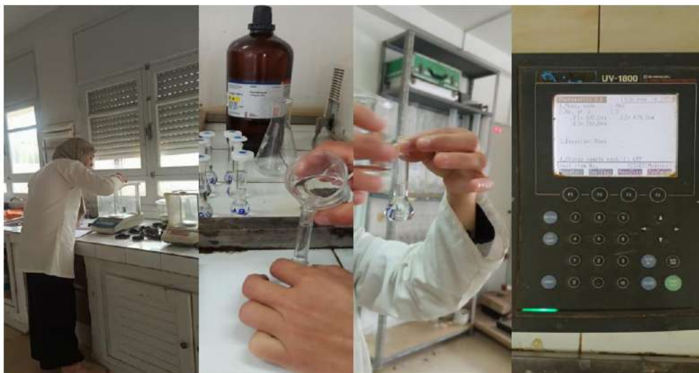
Determination of the Optical density using the spectrophotometer ( Original ).
