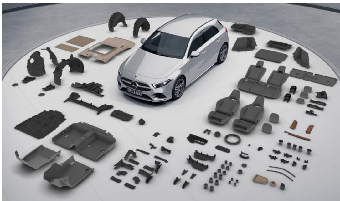
Figure 2 Mercedes-Benz A-Class features components manufactured using natural fiber-reinforced composites[7]
