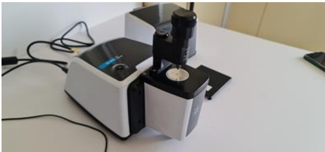
Figure 29 AGILENT CARY 630 FTIR
