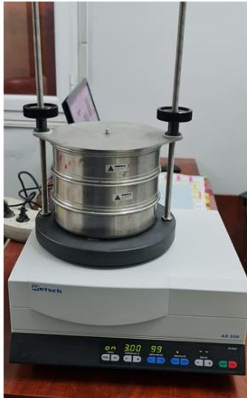
Figure 23 RETSCH AS-200 sieve shaker
