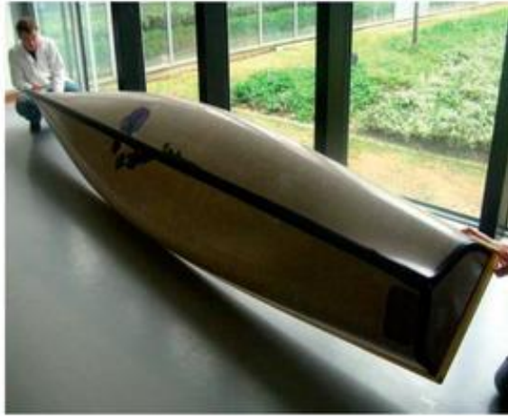
Figure 3 A canoe made from flax/PLA composites was developed as part of the NAVECOMAT project.[8]
