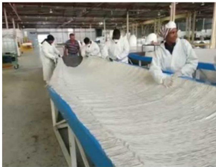
Figure 4 Manufacturing of wind turbine blades using composite material[9]
