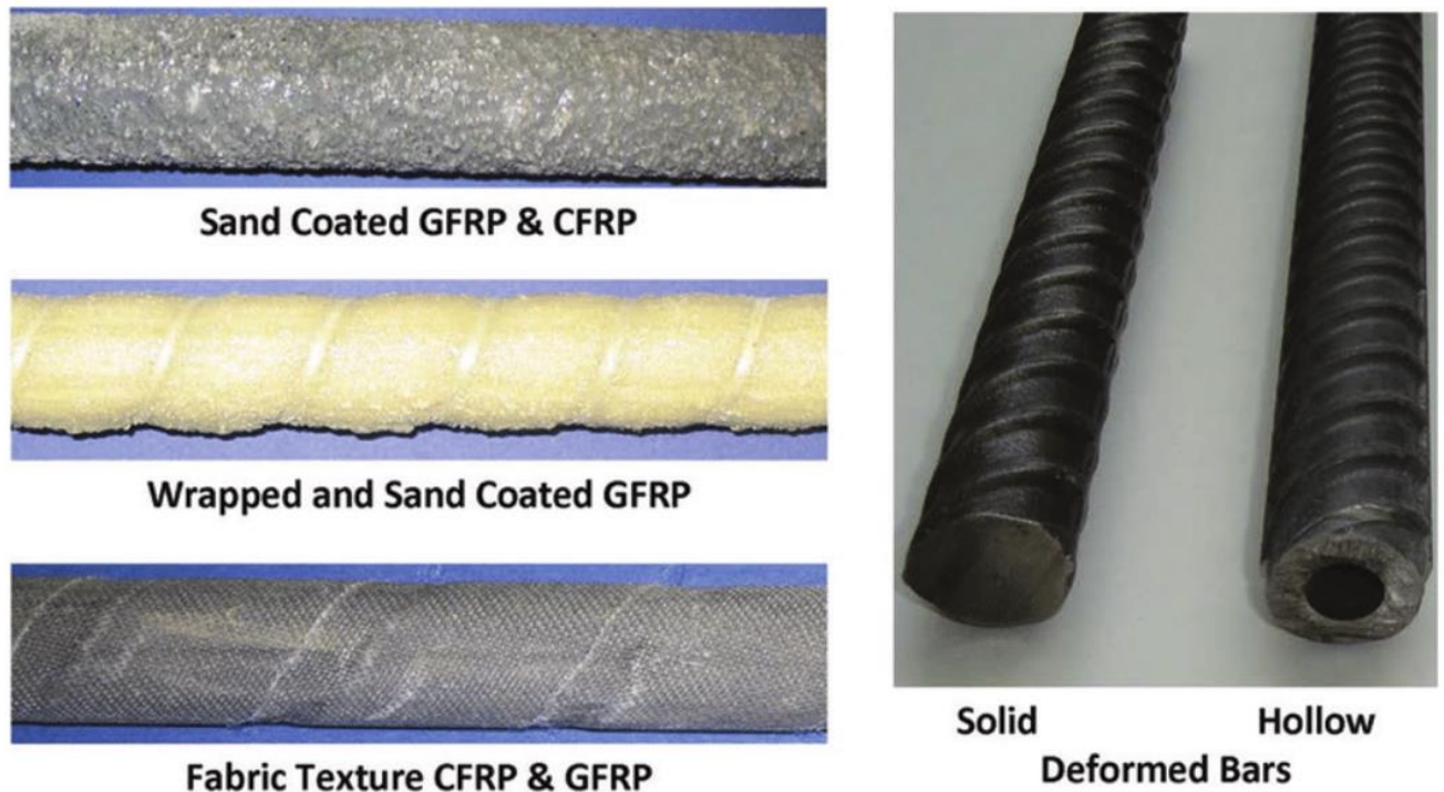
Figure 5 Carbon, glass fibre and steel bars[10]
