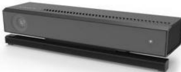
Figure 2.13: Microsoft Kinect 2.0 is an inexpensive depth camera. One of its uses could be markless motion capture [2].
