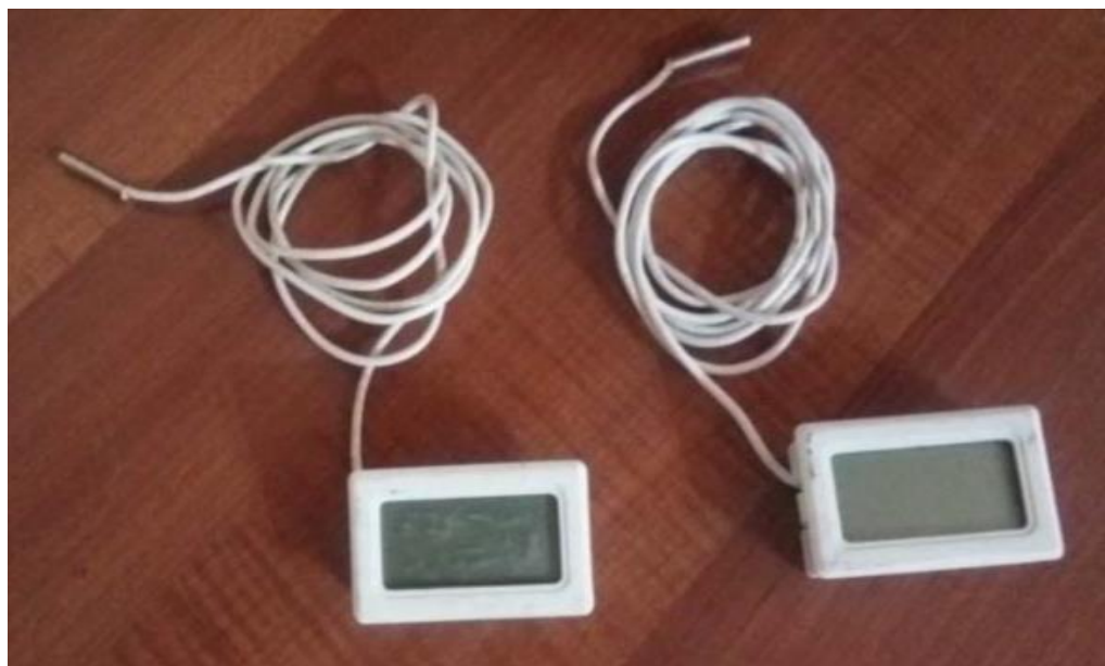
Figure.6: Thermocouples type K ( 0,01^{\circ}\text{C} ).
